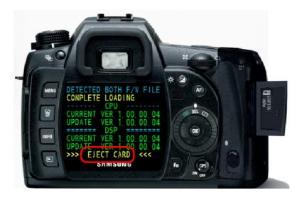
6. Remove the SD card and do not close the memory card slot cover.
