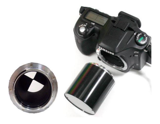
7 Put the camera (with the Cross) on the EV tester.
