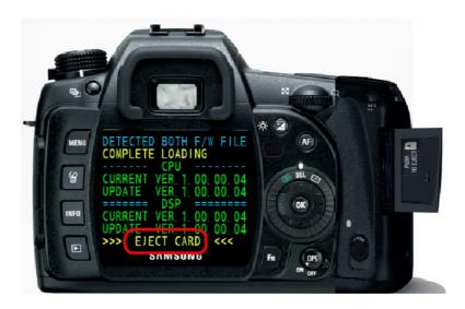
6. Remove the SD card (Do not close the memory card slot cover.)
