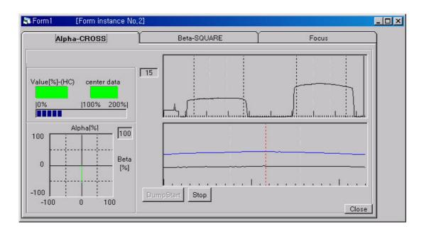
If the result displays as red color, adjust the AF sensor inclination by rotaing the two hexagon screws until the color comes to be green.
