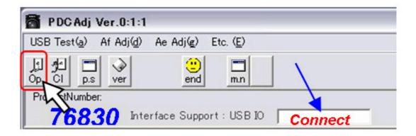
[Check] Check whether the [Connect] message displays on the USB IO.
