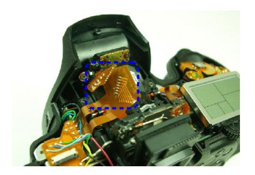
① Connect the lead wire on the 0-O170 (SI-LED) as shown.
