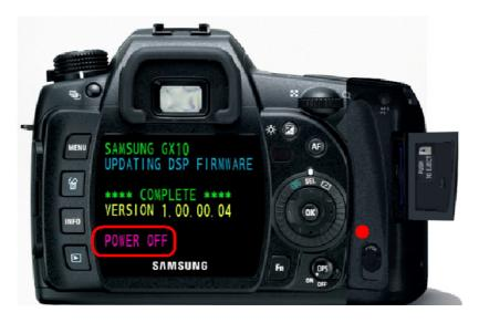
After completing the upgrade, "POWER OFF" message displays. The card access lamp (Red) still blinks.
