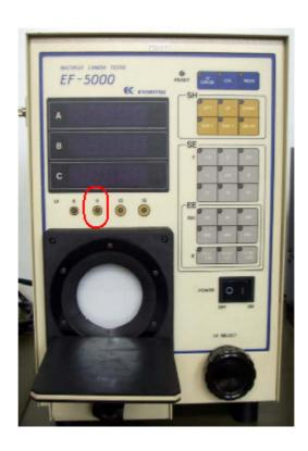
② Set the shutter speed to Tv 500. (In case of LV8, set the shutter speed to Tv 250 (ISO: 200)).
