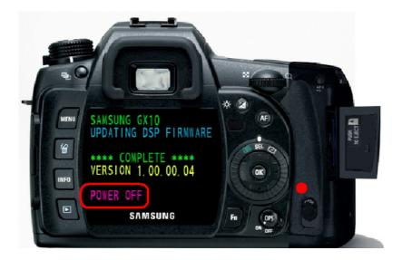
After completing the upgrade, "POWER OFF" message displays. The card access lamp (Red) still blinks.
