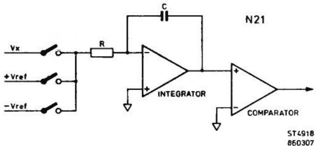
Figure 3.9 ADC principle
