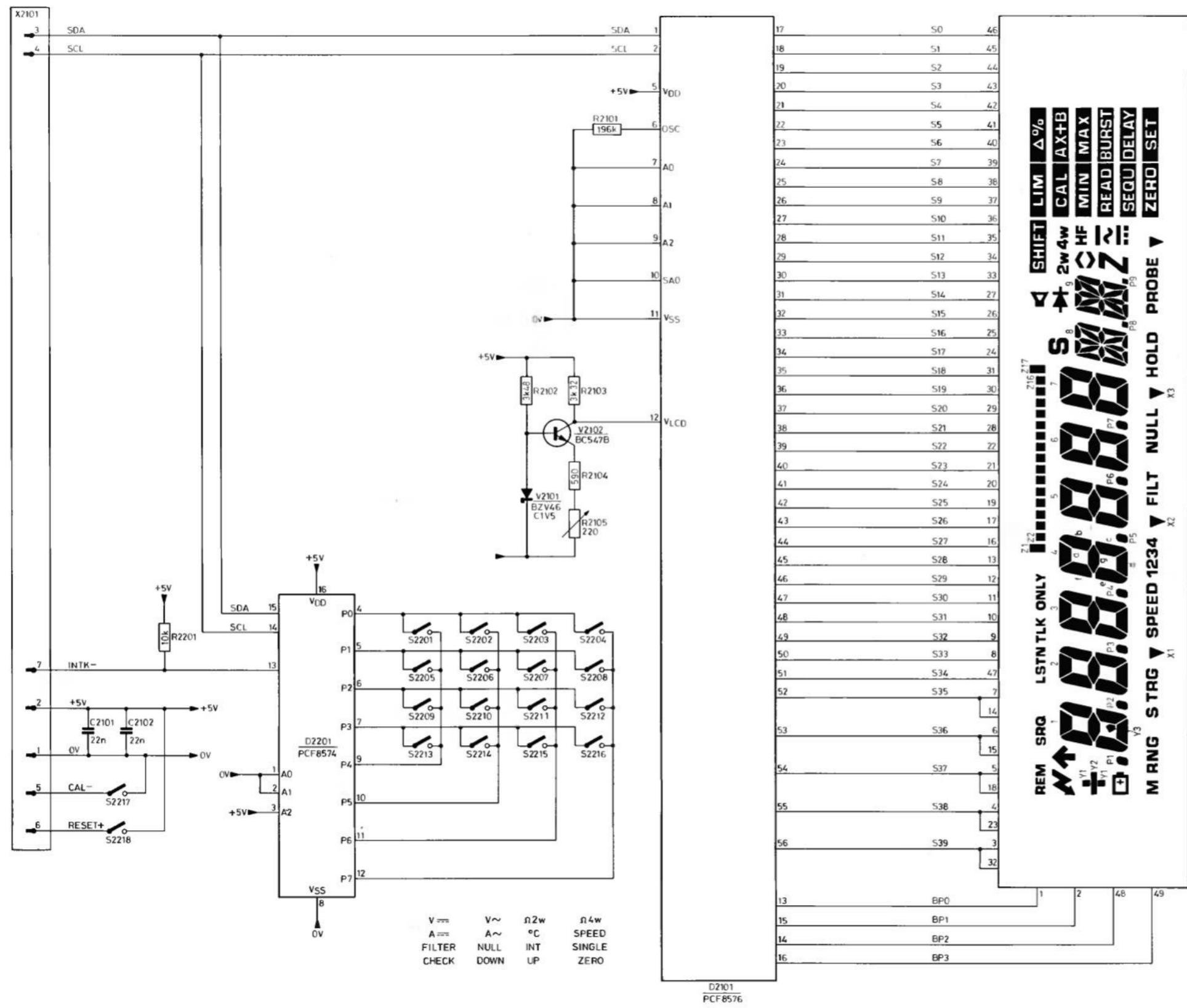
Figure 9.4 Display pcb, circuit diagram
