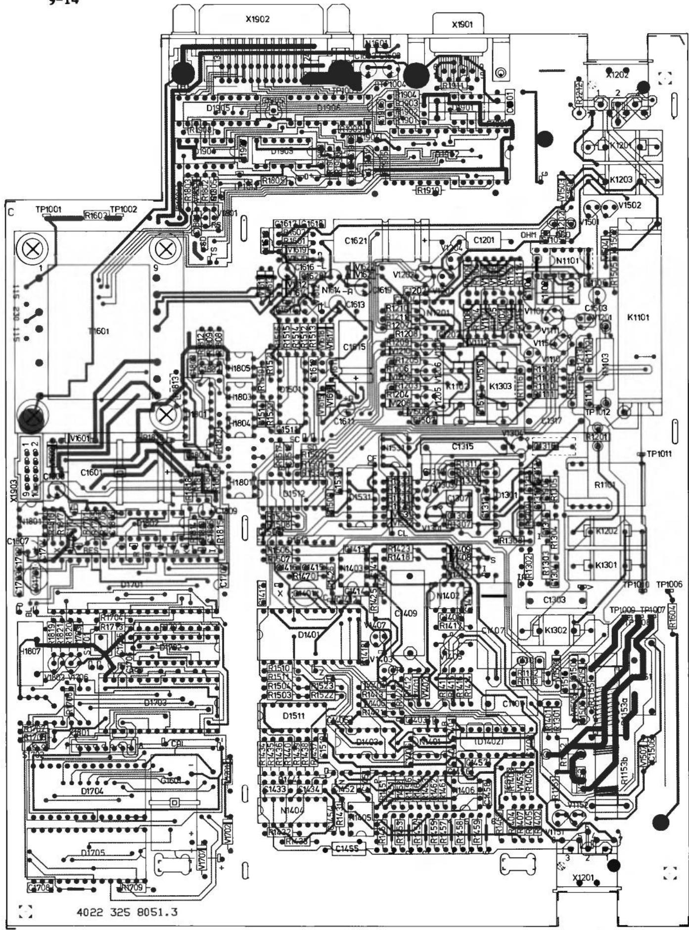
Figure 9.10 Main pcb version 4022 325 8051.3, component side
