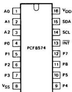
Figure 3.25 Pinning diagram
