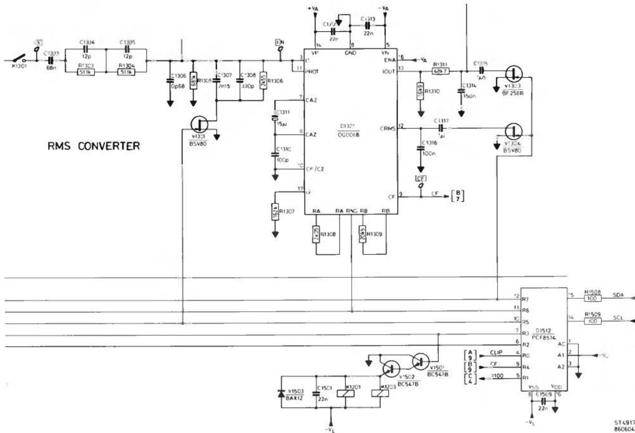
Figure 3.6 RMS converter
