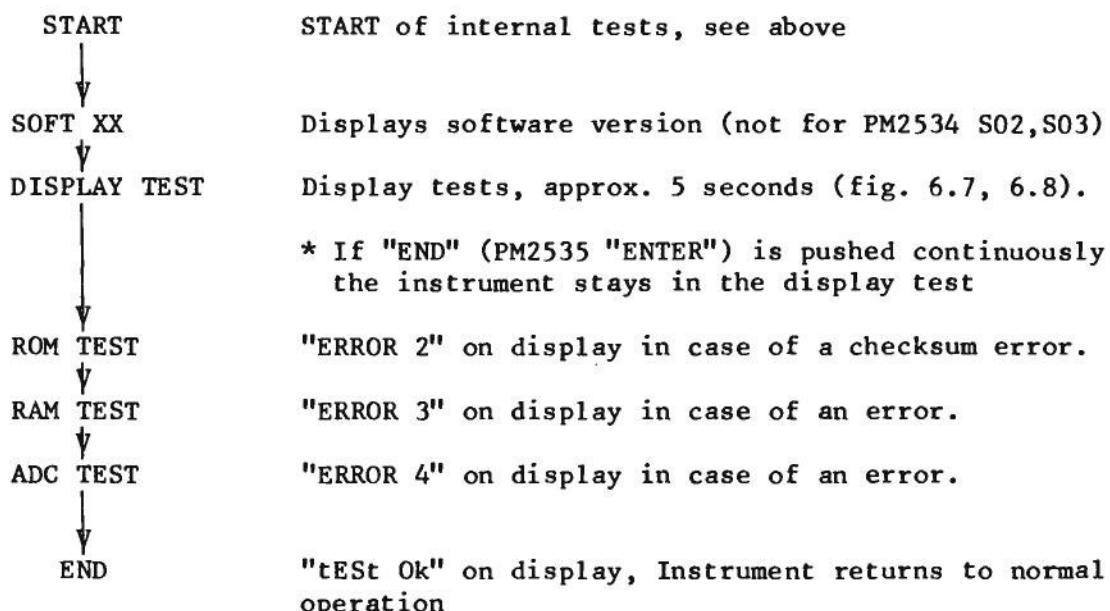
Figure 6.6 Built-in tests
