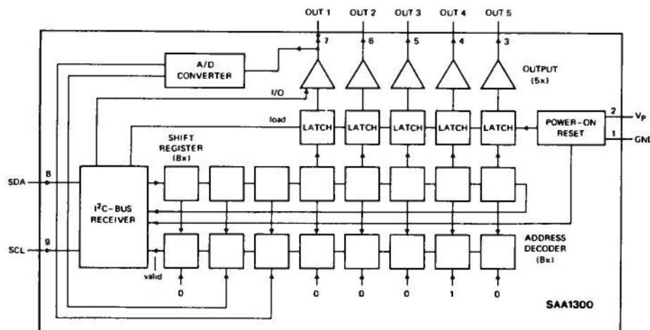
Figure 3.23 Block diagram
