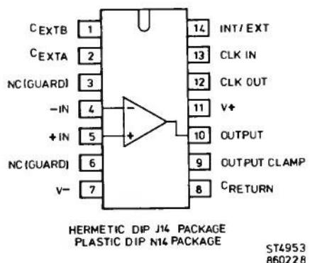
Figure 3.28 Pin connections
