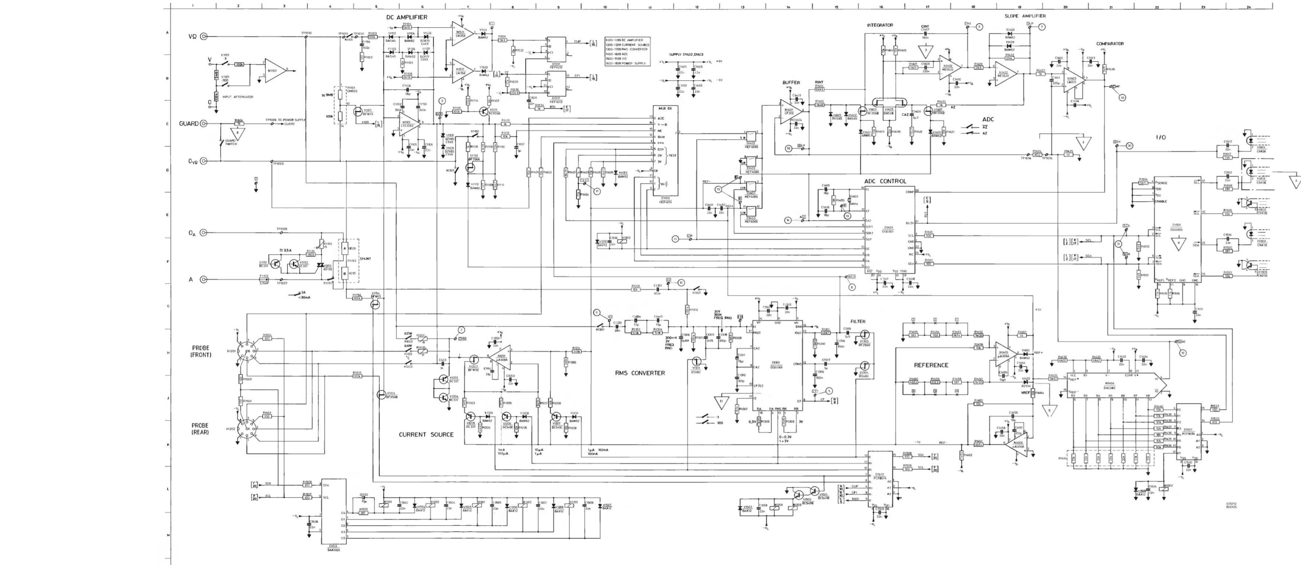
Figure 9.5 Main pcb, analog part circuit diagram
