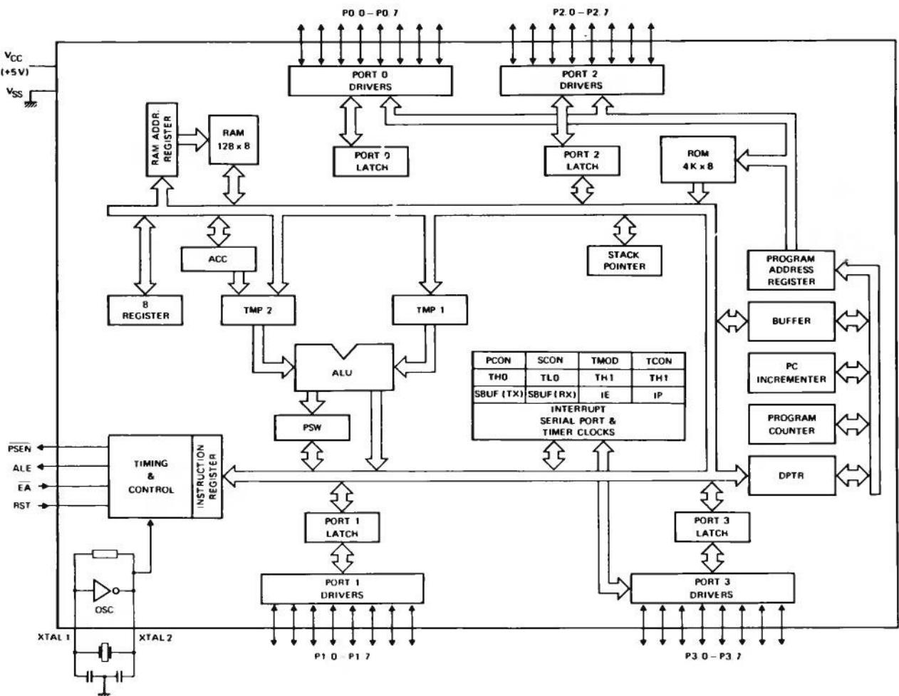
Figure 3.12 Block Diagram
