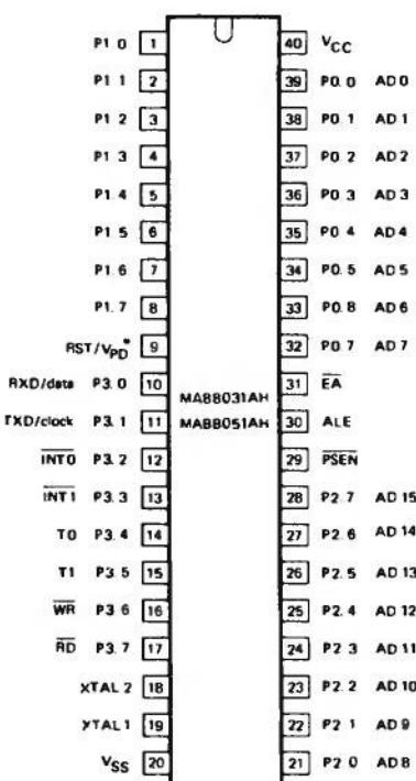
Figure 3.13 Pin Configuration
