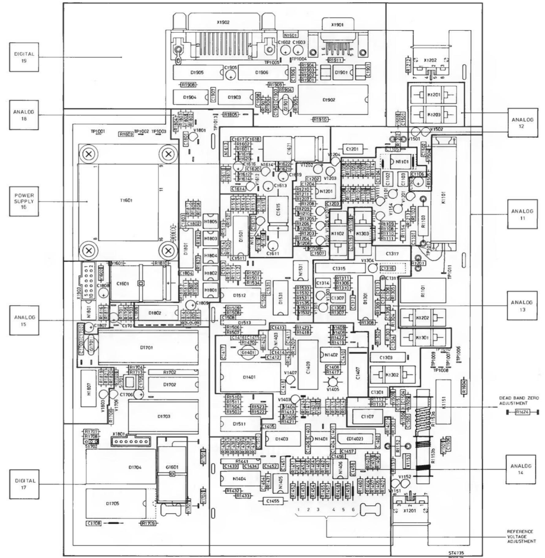
Figure 9-12 Main pcb parts location (version 4022 325 8051.3, almost equal to version 4022 325 8051.2)
