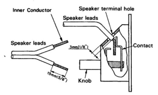
CAUTION: When using DA-A15DC, use more than 18AWG, SPT-2 cord with UL label for speaker leads.
