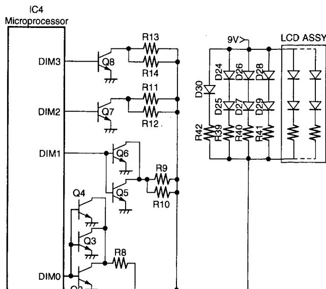
Fig.20 Dimmer circuit
