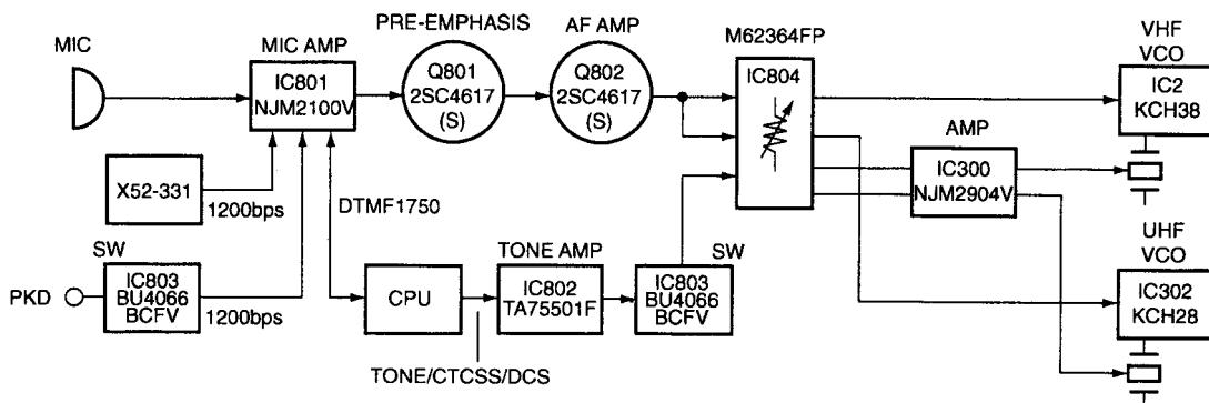
Fig.9 Modulation circuit
