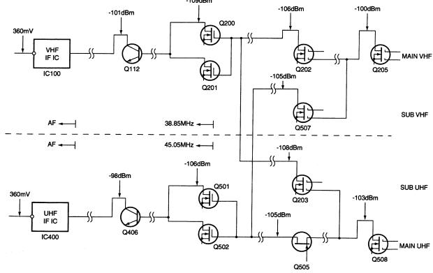
Note1: The 12dB SINAD levels were plotted using a standard signal generator through a 0.01μF ceramic capacitor at each point from the RF to the first IF.
