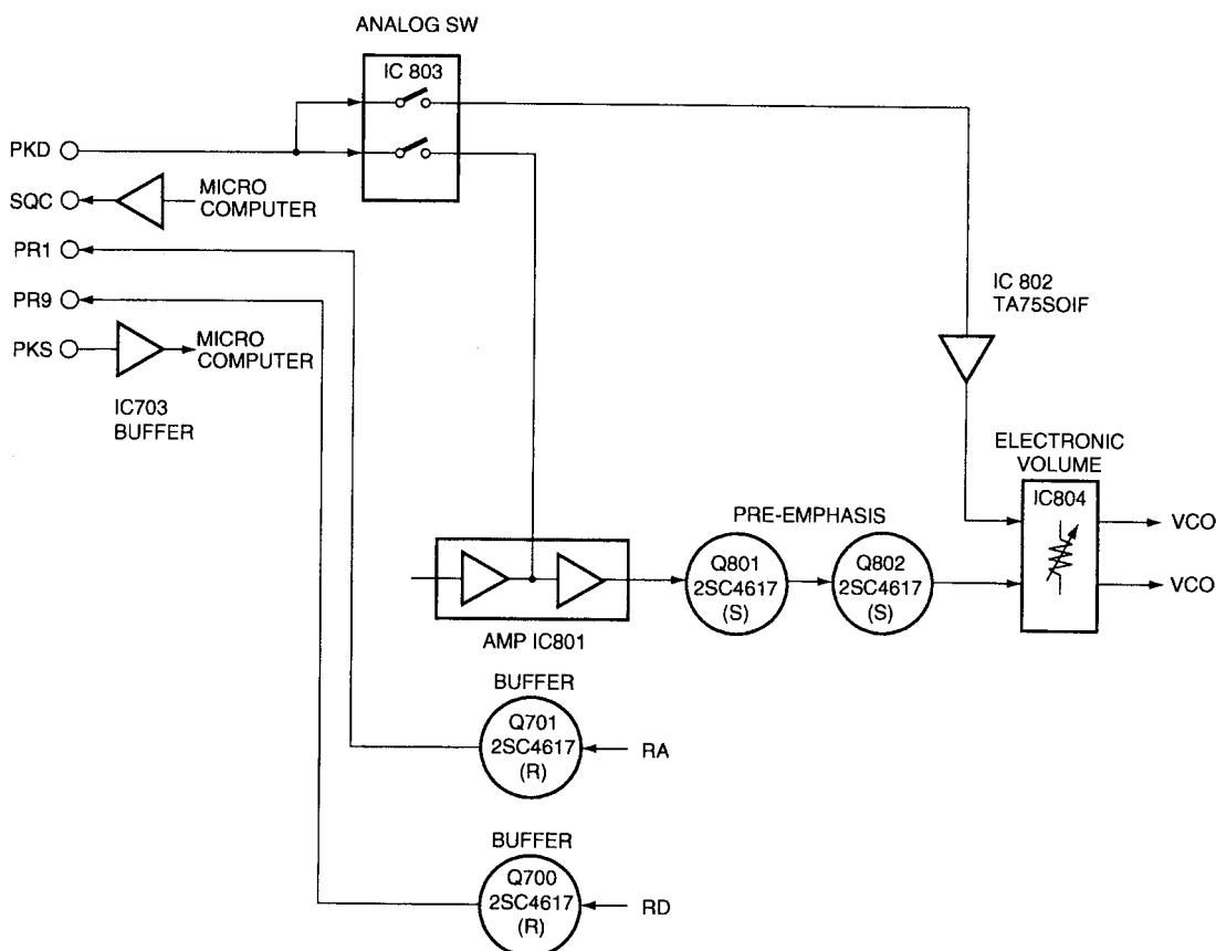
Fig.18 Transmission signals
