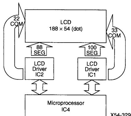
Fig.19 Display circuit
