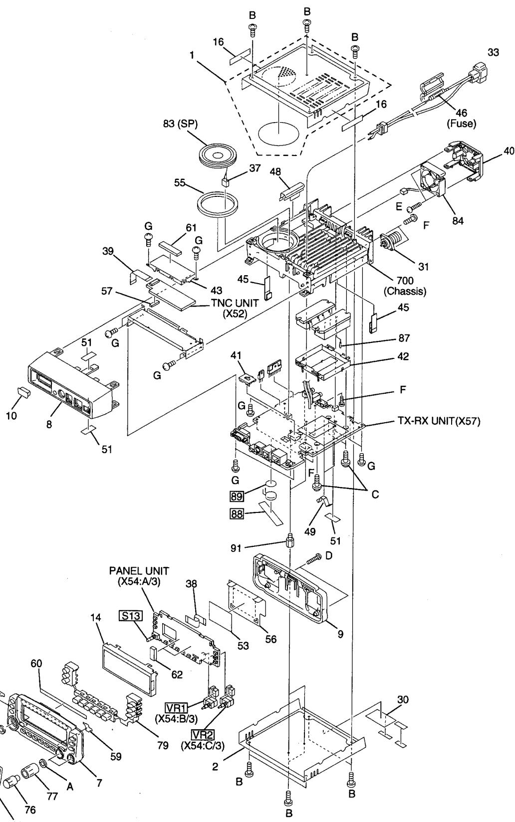
Parts with the exploded numbers larger than 700 are not supplied. 35
