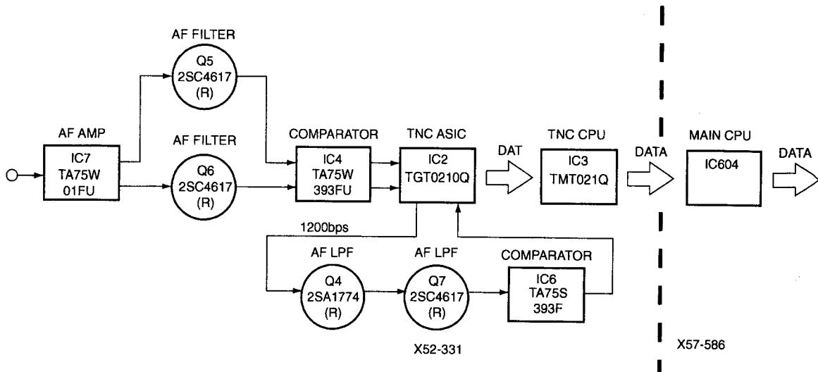
Fig.7 TNC unit circuit
