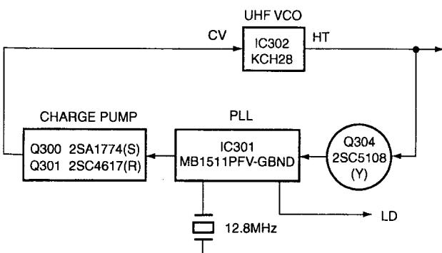
**Fig.12 PLL circuit**
