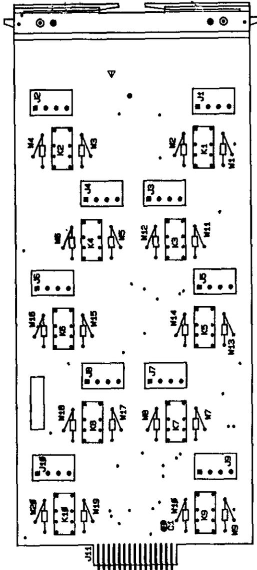
Figure 4-1. Model 7066, Component Location Drawing
