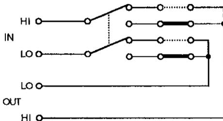
Provides 10 channels of 2-pole switching, with a quick disconnect terminal block for each channel.
