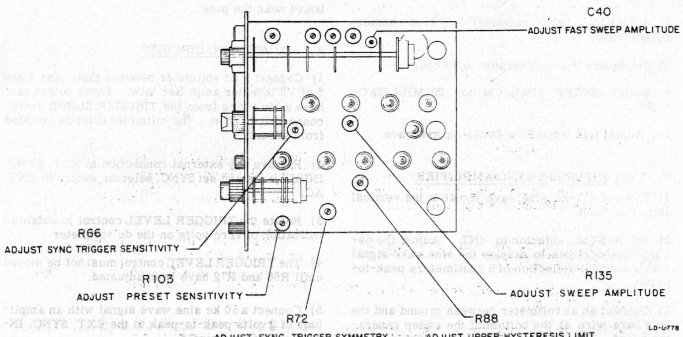
Figure 4-7B. Sweep Generator Adjustments
