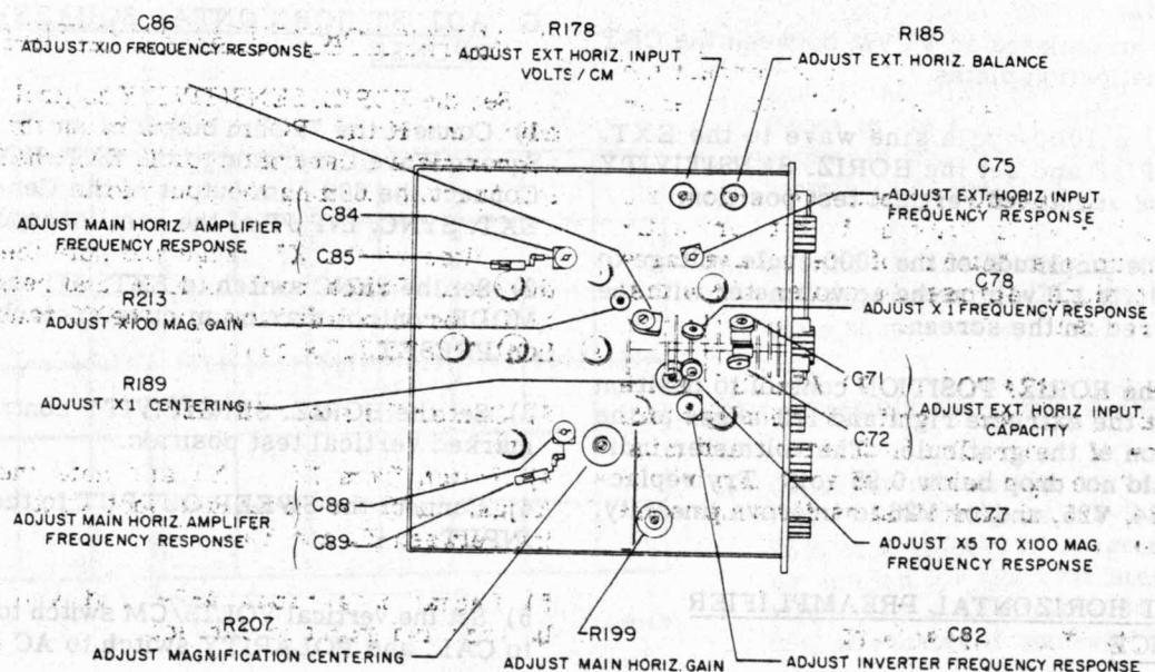
Figure 4-4B. Horizontal Amplifier Adjustments
