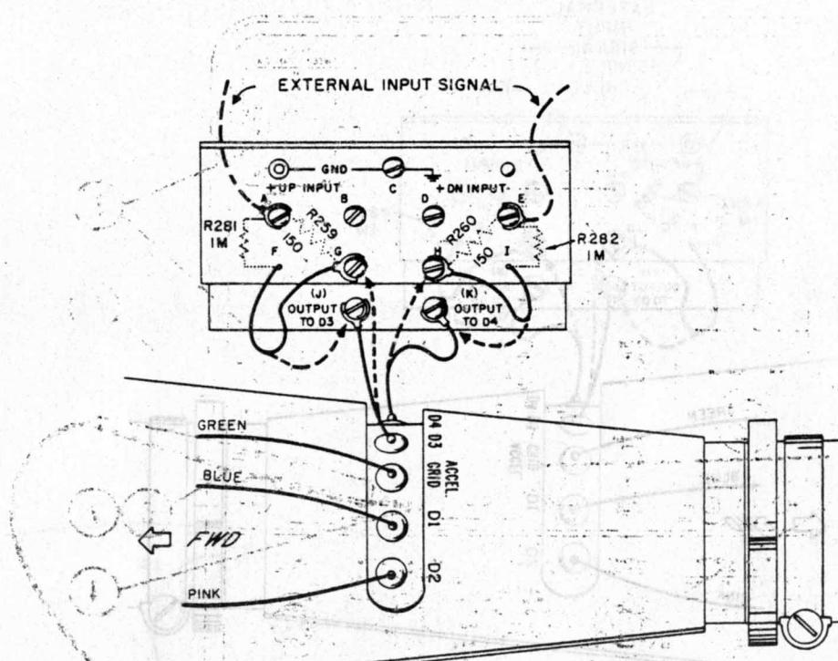
**CAUTION** - The deflection plates of the oscilloscope operate at a d-c potential of approximately +250 volts. Therefore, there can be no common chassis connection between the signal source and the oscilloscope. In most cases the signal source chassis will assume the deflection plate potential. Turn off the instrument before making connection to deflection plate terminals.
