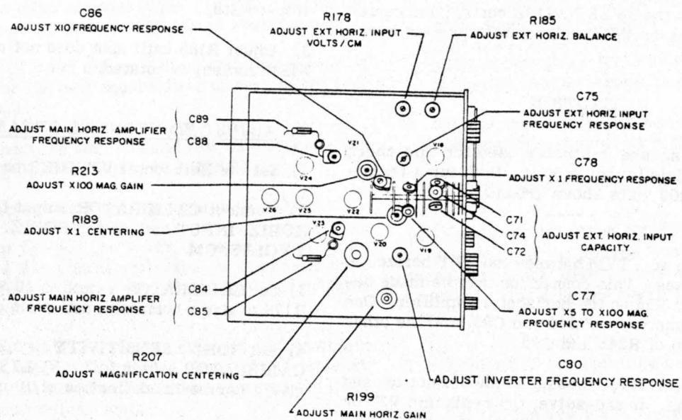
Figure 4-4A. Horizontal Amplifier Adjustments
