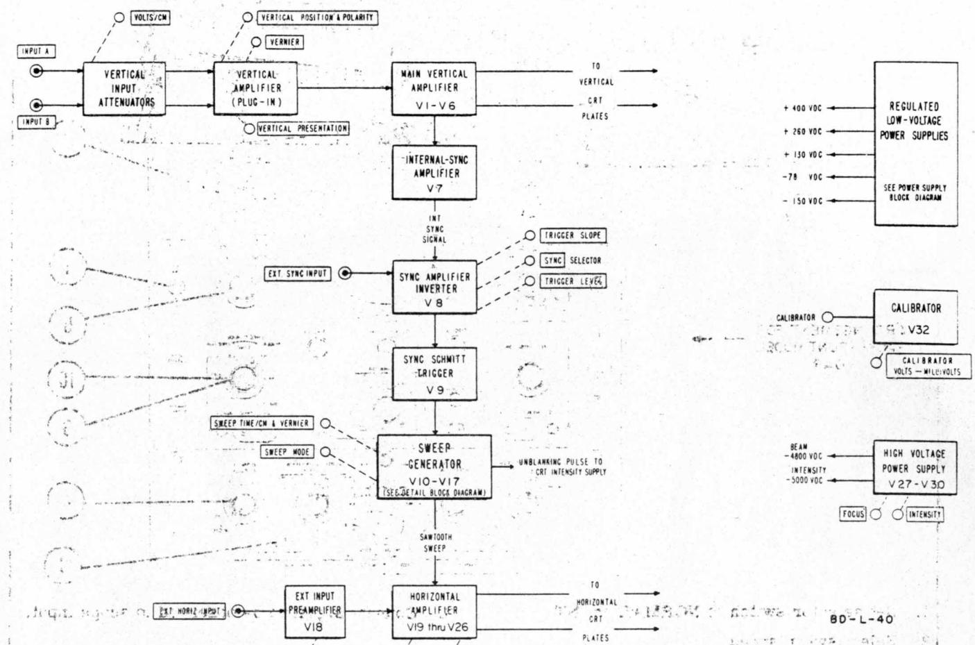
Figure 3-1. Block Diagram: Complete Oscilloscope
