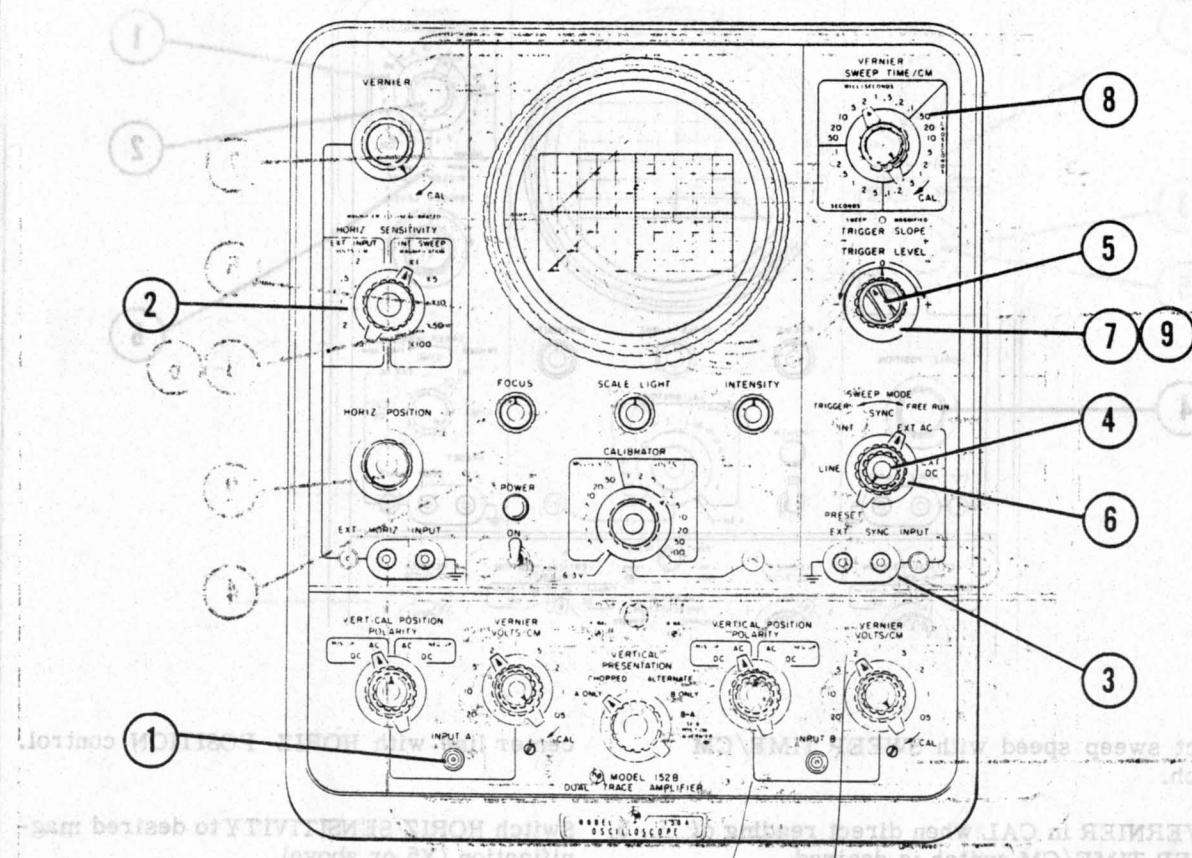
1. Connect vertical input signal to the plug-in amplifier.
