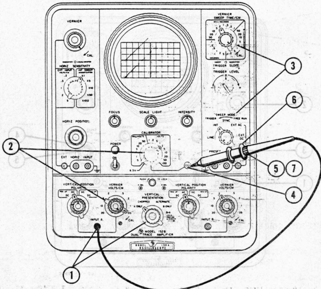
1. Connect the AC-21 Probe to the desired vertical input, and set the VERTICAL PRESENTATION selector to the corresponding input.
