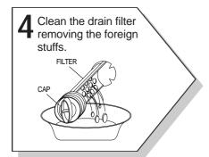
Put in the filter along the guiding prominence of the case. Please note the left position of the filter adjusting the groove to the guide rib.
