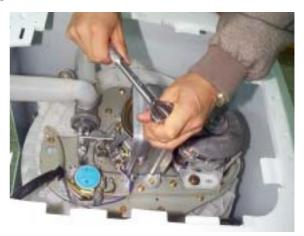
11) Remove four special bolt of gear mechanism assy by using a box wrentch.
