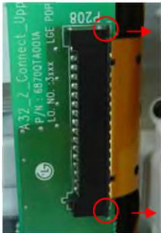
Separate the fixed Screw of Z-Board.
