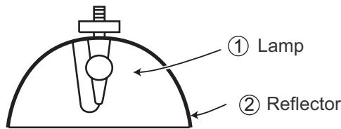
**DANGER !** — Never turn the power on without the lamp to avoid electric-shock or damage of the devices since the stabilizer generates high voltages at its start.
