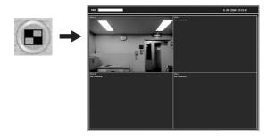
Memo: In case of the quad-screen display, when selecting one camera video a red frame indicating which camera has been selected is displayed.
