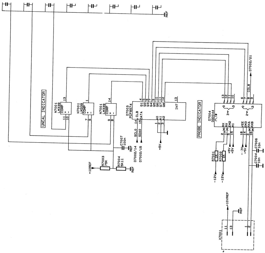
Figure 10.3 Circuit diagram of front unit, front controls and probe indication
