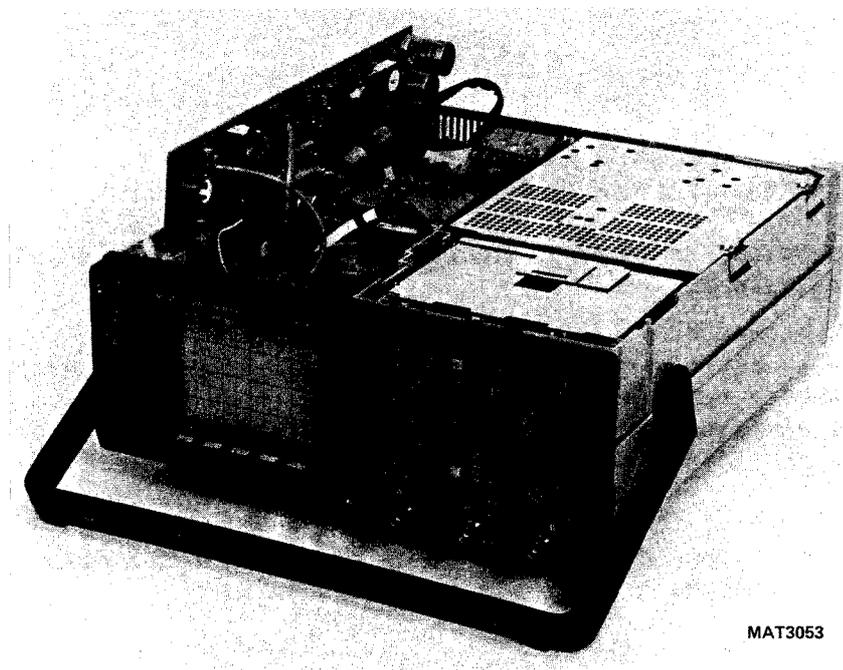
Figure 23.3 Power supply unit outside the instrument
