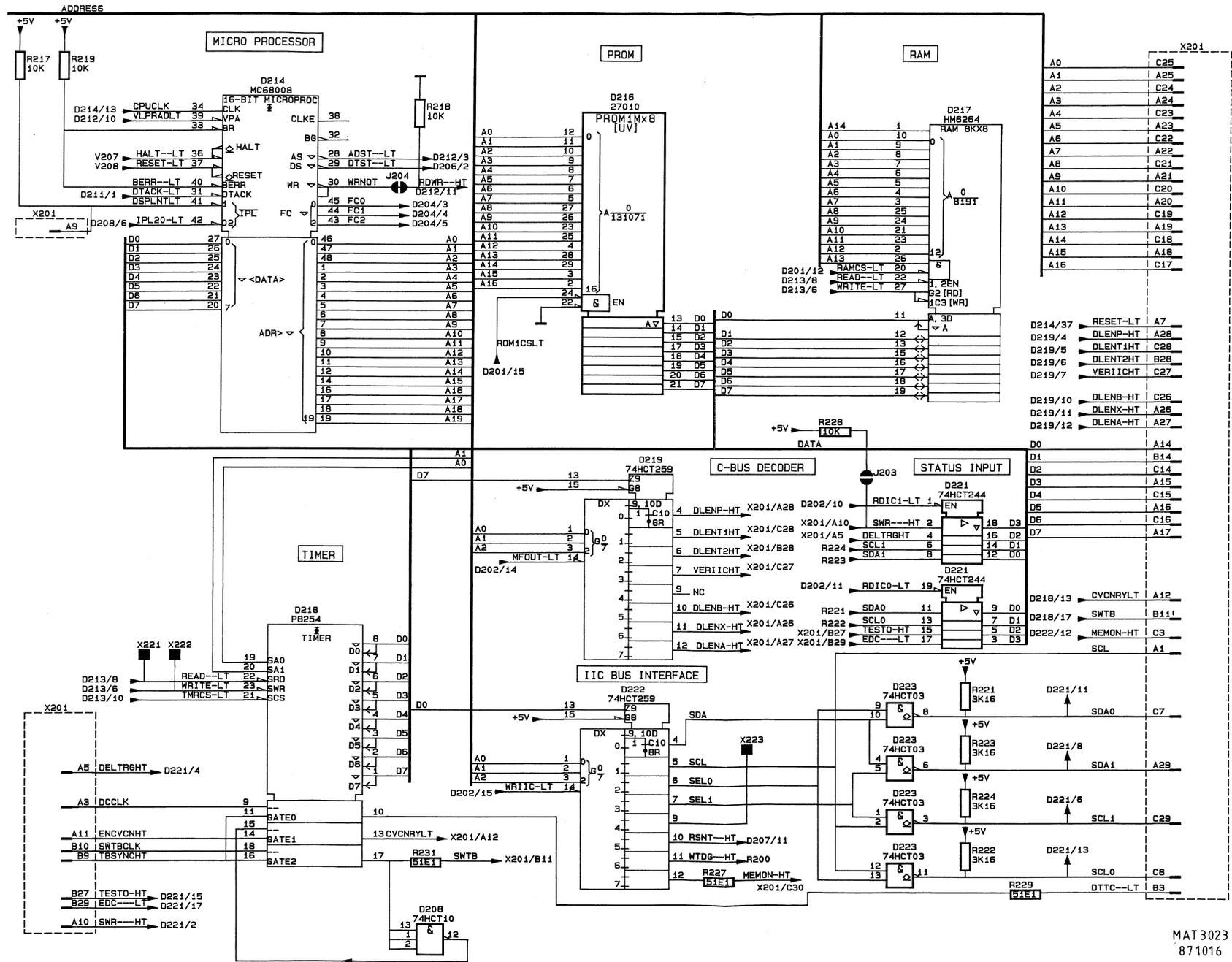
Figure 13.5 Circuit diagram of CPU unit, part 2
