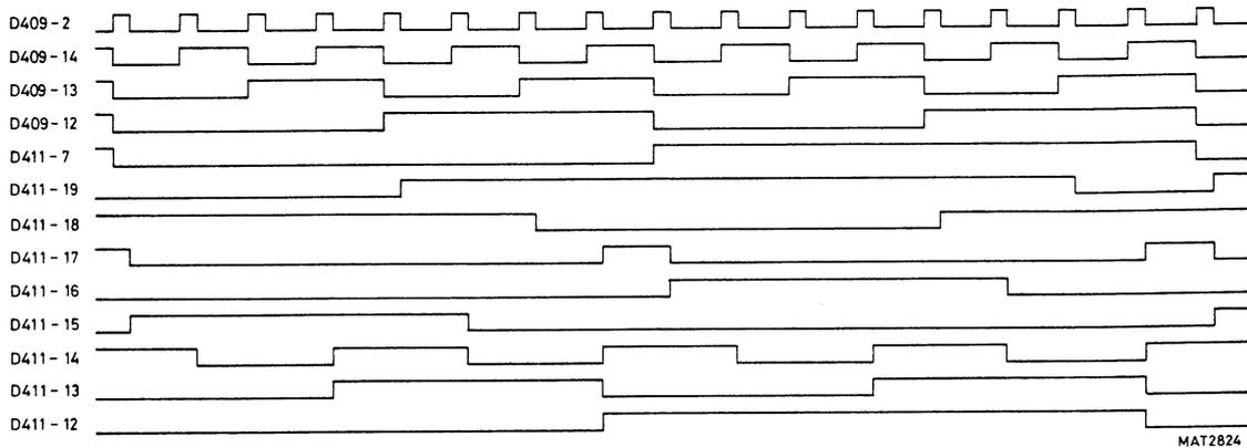
Figure 15.2 Timing diagram CCD and ADC timing
