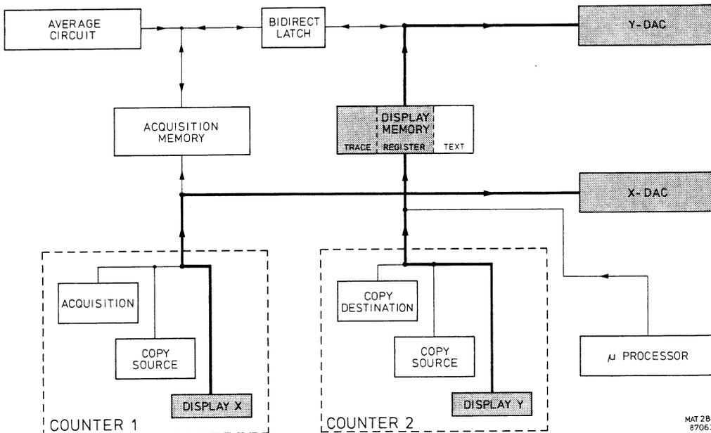
Figure 14.5 Block diagram of trace/register display flow
