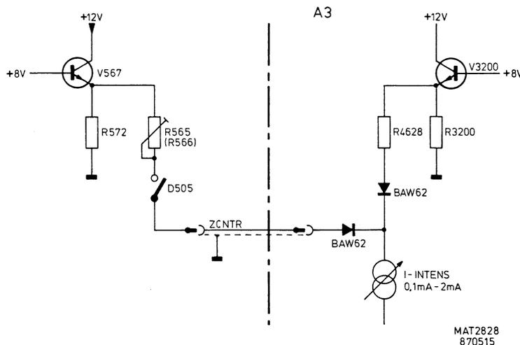
Figure 16.4 Z control for PLOT or DTJN
