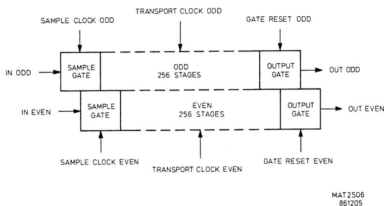
Figure 18.1 Schematic diagram of a P<sup>2</sup>CCD circuit
