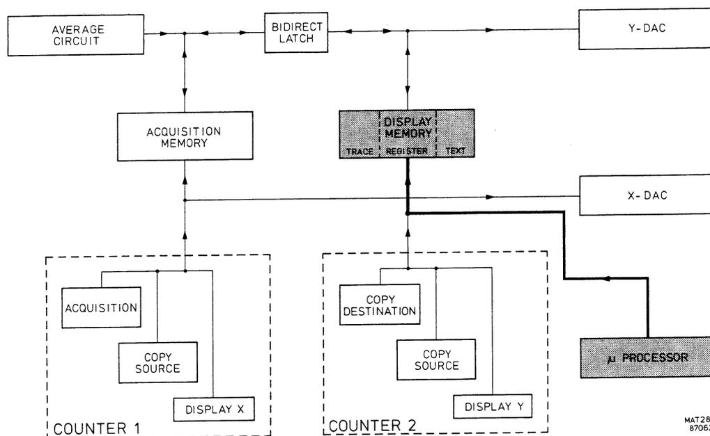
Figure 14.7 Block diagram of the clear function
