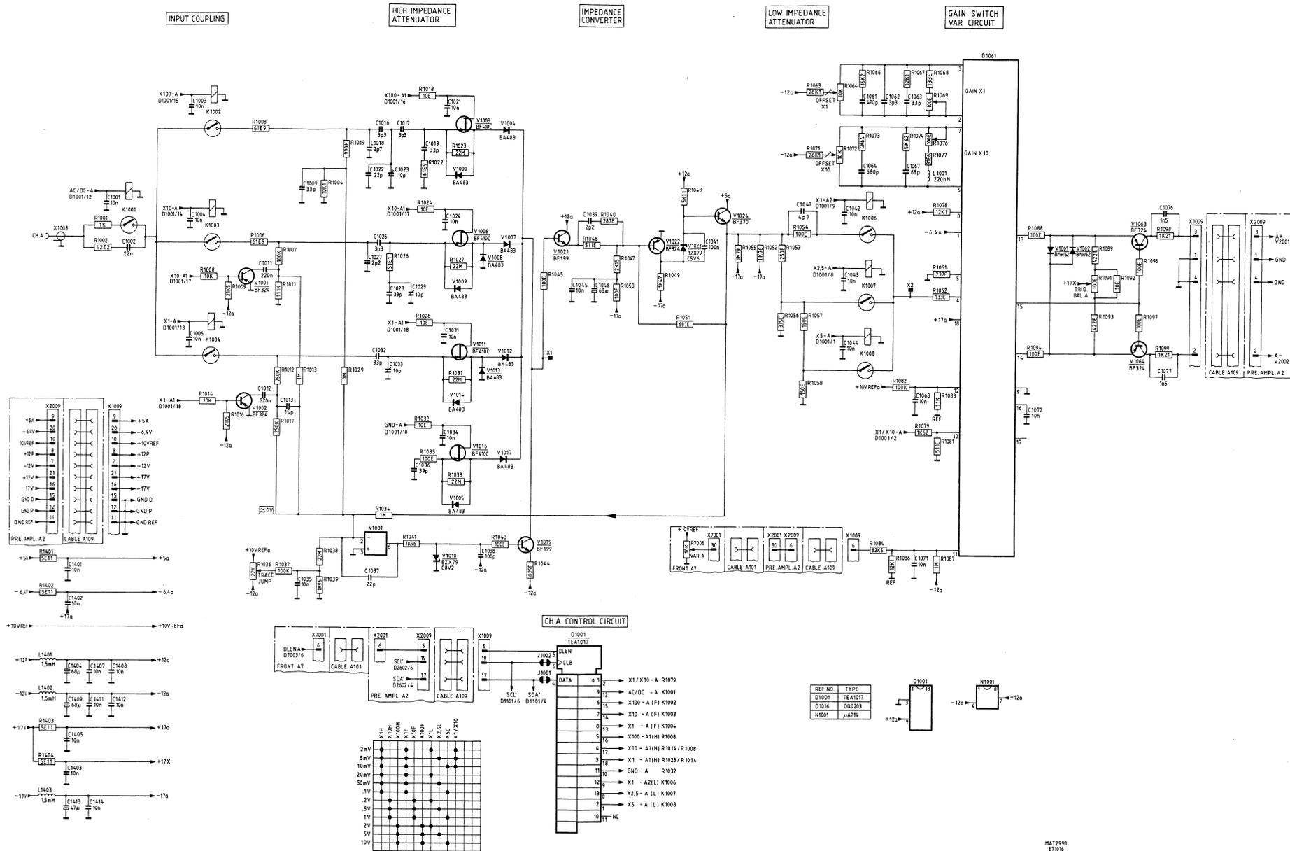
Figure 4.3 Circuit diagram of attenuator, ch.A
