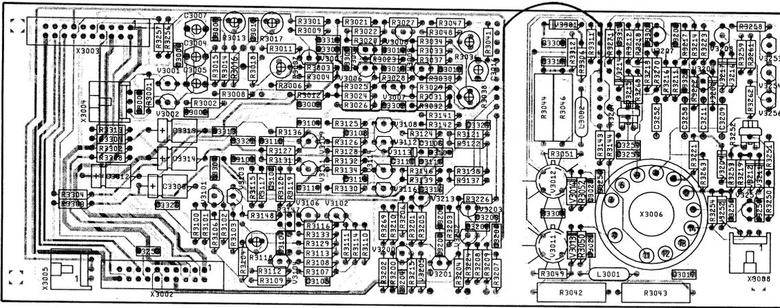
Figure 6.3 XYZ amplifier unit p.c.b.
