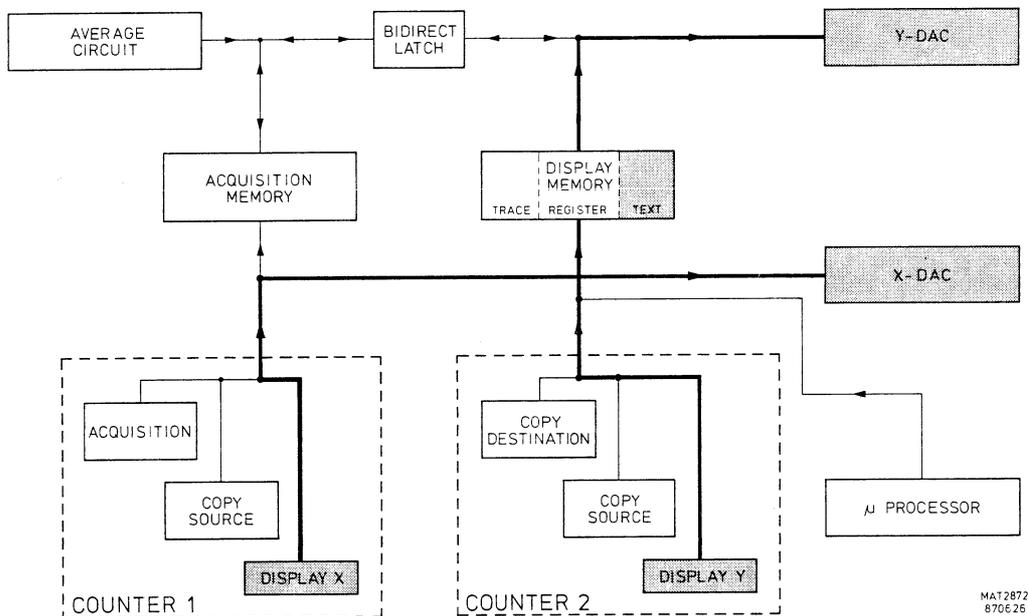
Figure 14.6 Block diagram of text/cursors display flow
