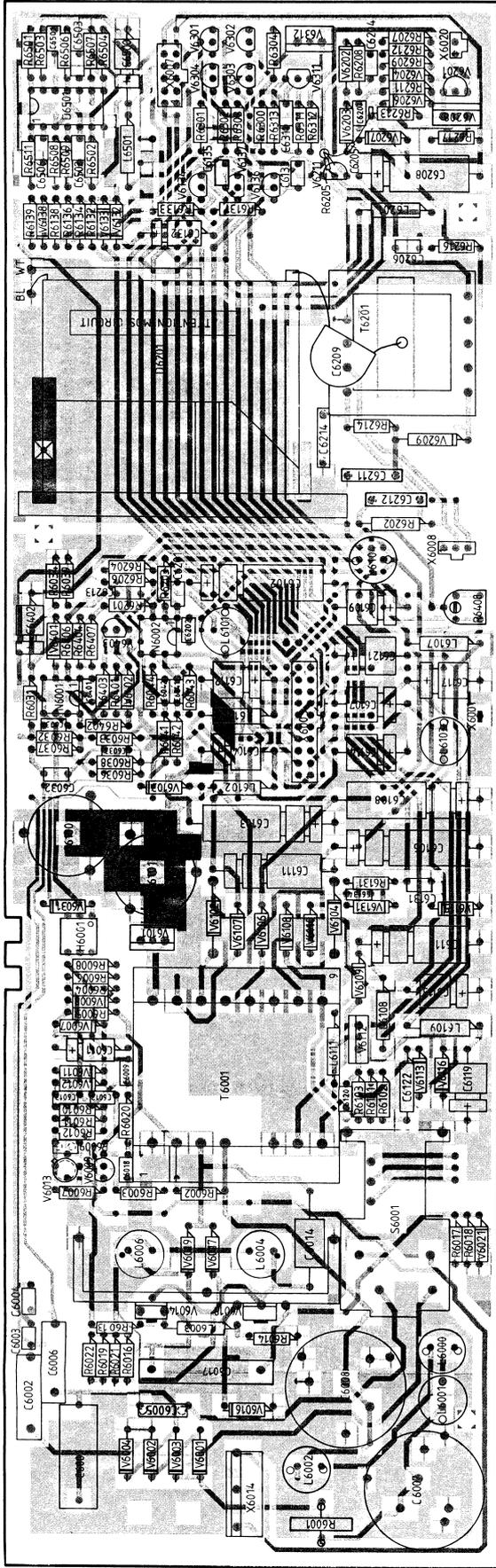
Figure 9.4 Power supply unit p.c.b.
