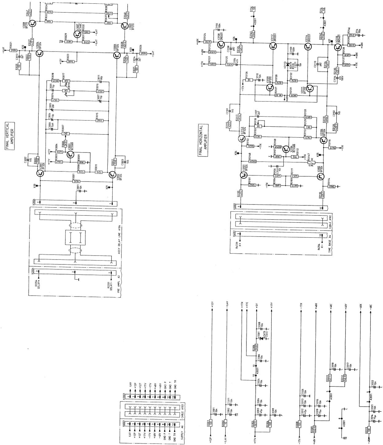
Figure 6.2 Circuit diagram of XYZ amplifiers, final X and Y amplifiers
