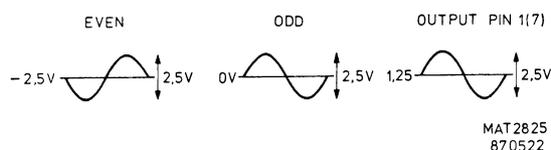
Figure 16.1 Waveforms on N501
