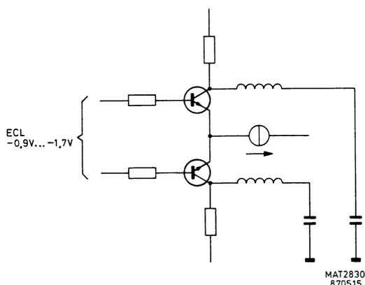
Figure 19.1 Principle of the sample clock drivers
