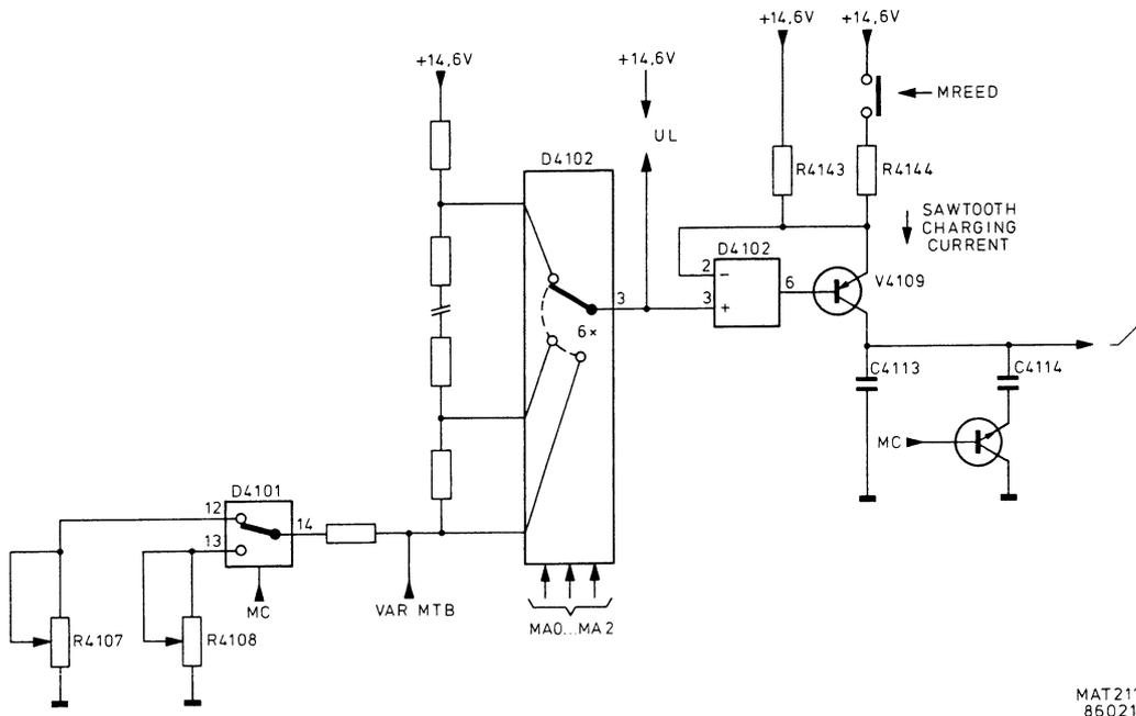
Figure 7.2 Simplified diagram of the time-base sweep generator
