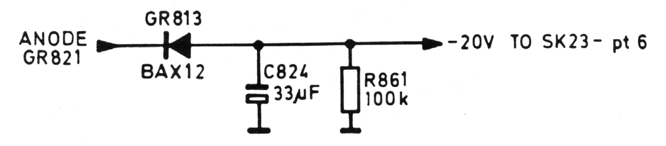
The print track between SK23 pt6 and R1043 on the storage unit is interrupted.
