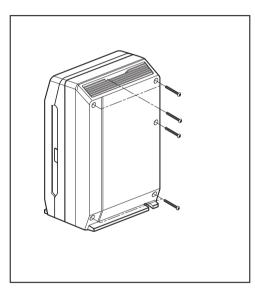
2. Unscrew bolts using a wrench. (Turn it counter clockwise.)
