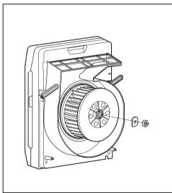
3. FAN is disassembled by holding and pulling fan.
