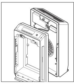
5. Remove 4 screws from the Main PCB using a screw driver(+).
