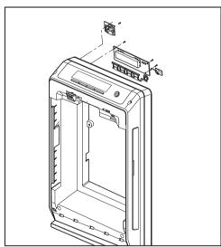
6. Remove a screw from the Control PCB Case using a screw driver(+).
