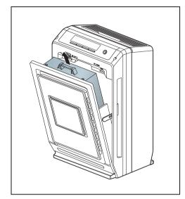
Separate Connector Bar from the Front Panel using a screw driver (-).
