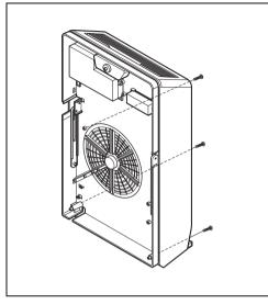
2. Remove 2 screws (1 each from left/right) from the Connector Bar using a screw driver(+).
