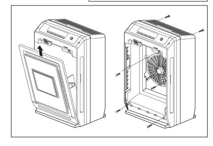
4. Remove Main PCB Wire. (Please be careful not to damage the Main PCB Wire when removing the Front Case Assembly.)
