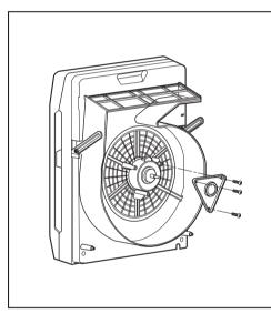
5. Remove the Motor Cover. Take out the Motor. Please be careful not to damage the Motor wire when removing the motor.
