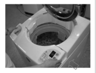
3 Remove 4 bolts and separate PLATE T from washing machine.
