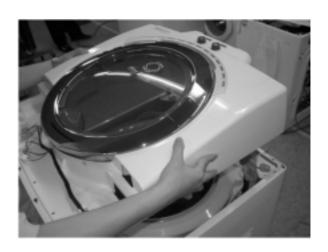
4 Unscrew 4 bolts and separates COVER TUB from TUB ass'y.
