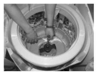
(8) Separate TUB I from TUB ass'y.
