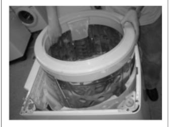
9 Lay the top of the washing machine on the floor. ①Unscrew 4 special bolts of GEAR PROTECT using a box wrench and separate GEAR PROTECT.
