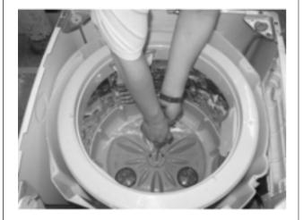
① Unscrew special nut using 'T' type box wrench.
