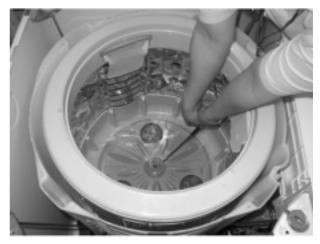
6 Unscrew PULSATOR mounting screw and separates PULSATOR form TUB ass'y.
