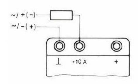
A separate connection terminal (5) is provided for direct current measurements above 2 A up to 10 A.
