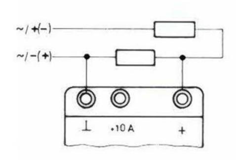
Currents above 10 A can be measured with shunts, e.g. 100 A/100 mV or 300 A/300 mV.
