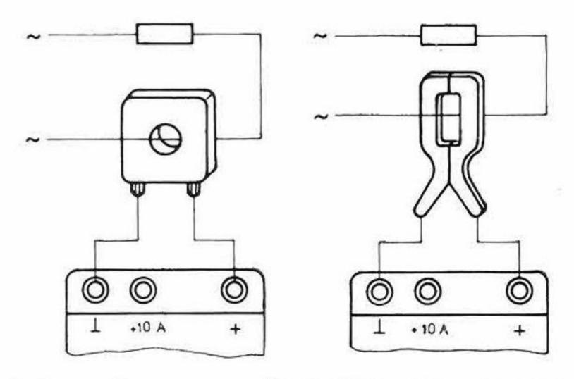
Split-core current transformers allow for measurements of
