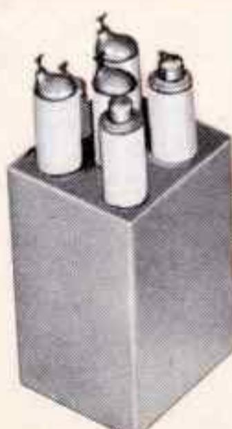
Gaussian wave shape pulse output. Input 2 KV, 3.5  $\mu$ sec. Output 2.5 KV-5A., 80 kHz rate. Corona free-35,000 feet. MIL-T-27C; 1 $\frac{5}{8}$  x 1 $\frac{5}{8}$  x 3 $\frac{1}{8}$ , 1 lb.
