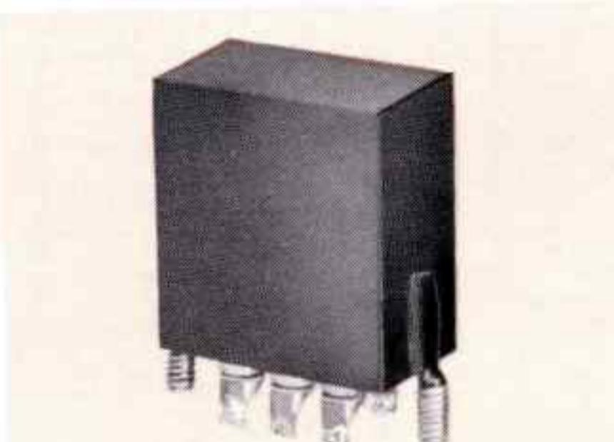
Free running blocking oscillator transformer. 600 ohms, 1:1:1, 5  $\mu$ sec.  $\pm$  1, 12000  $\pm$  10% PPS. Output 600 V.  $\pm$ 10%. Temperature stable -62° C. to 85° C. MIL-T-27C; 3/4 x 1 $\frac{1}{4}$  x 1 $\frac{1}{8}$ ; 1 $\frac{1}{2}$  oz.
