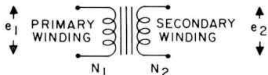
The primary winding is connected to the alternating current voltage source and the secondary winding is connected to the load.
