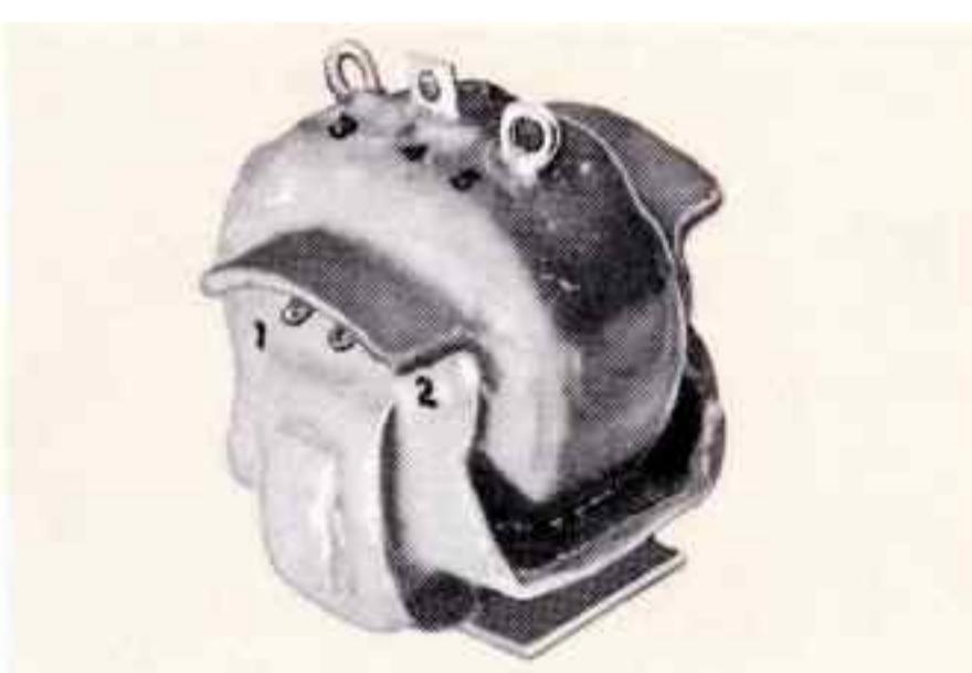
High voltage filament transformer. Primary 115 V., 380/1600 Hz to 5 VCT.-10 A., 21 KV hipot. 160° C. MIL-T-27C Grade 5; 2¼ x 2½ x 2¼", 10 ounce.
