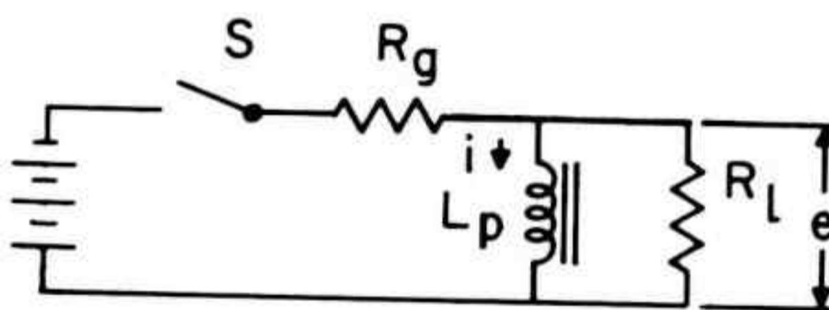
This circuit was obtained from the generalized circuit by eliminating all components that are not effective at low frequency.
