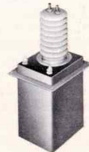
Output to Klystron. 3.5  $\mu$ sec. pulses in group of pulse trains at high rep. rate. 1% droop over pulse train. 43 KV Hipot. MIL-T-27C; NA case; 4 $\frac{1}{4}$  x 5 x 6 $\frac{3}{4}$ , 11 $\frac{1}{2}$  lb.
