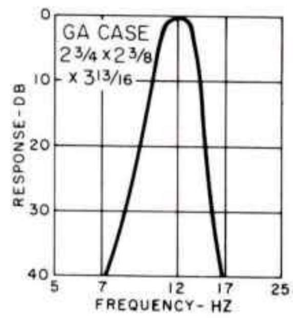
Twelve Hz band pass filter. From 11 thru 13 Hz attenuation less than 2 db. At 7 Hz and at 17 Hz, attenuation greater than 40 db. Source and load 50K ohms. MIL-F-18327C. Wt. 2.5 lbs.
