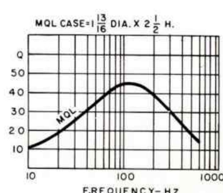
Since these high Q coils will saturate before any appreciable temperature rises occur, heating is usually not a problem. A general rule would be that 4 times the DC listings may be applied without any detrimental heating due to copper loss.
