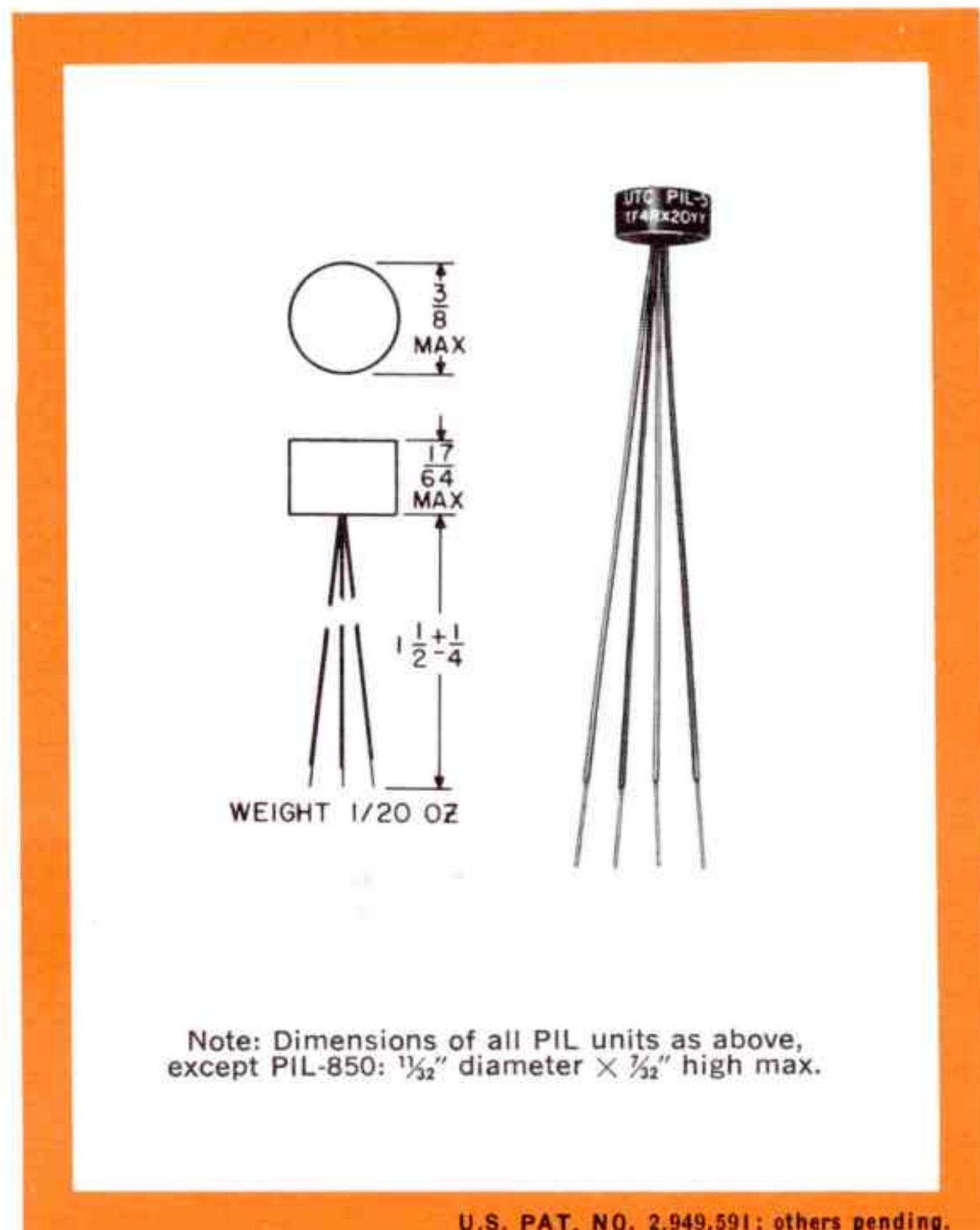
Note: Dimensions of all PIL units as above, except PIL-850:  $1\frac{1}{2}$ " diameter  $\times \frac{7}{32}$ " high max.
