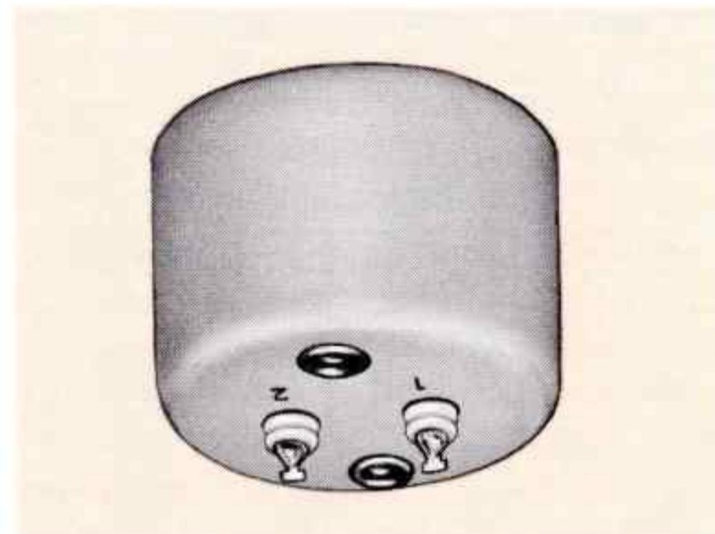
Constant 20 millihenries inductor. Inductance variation less than 2% from 0.1 to 500 V at 100 kHz. Q at 1 volt 100 kHz greater than 100. Case size: 1 1/8 O.D. x 1 3/16" high. MIL-T-27C.
