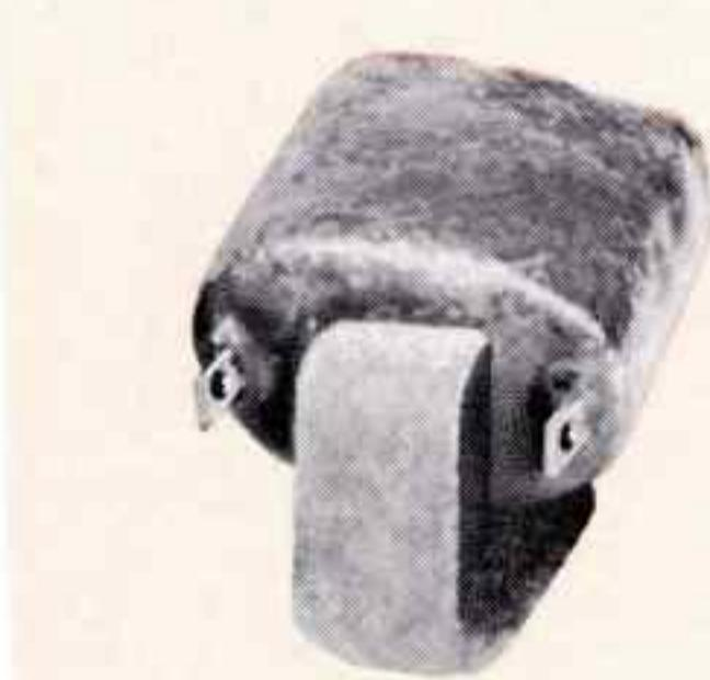
Pulse current transformer, Thyatron cathode to 50 ohms. Input 100A. Output 200 V. to 50 ohms. .5/2.4  $\mu$ sec. 2000 PPS. MIL-T-27C; 1 $\frac{3}{4}$  x 1 $\frac{1}{4}$  x 1 $\frac{1}{4}$ , 2 oz.
