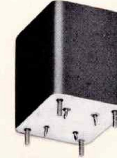
Constant phase shift band pass filter, 400 Hz. 380 Hz to 420 Hz within  $\pm 0.2$  degrees and within  $\pm 0.5$  db. At least 5 db at 800 Hz, 40 db at 1200 Hz and other harmonics of 400 Hz. Harmonic distortion less than 0.3%. Source 200 ohms, load 100 K ohms. MIL-F-18327C. FA CASE, 2 5/16 x 2 5/16 x 3 1/8". Wt. approx. 1 lb.
