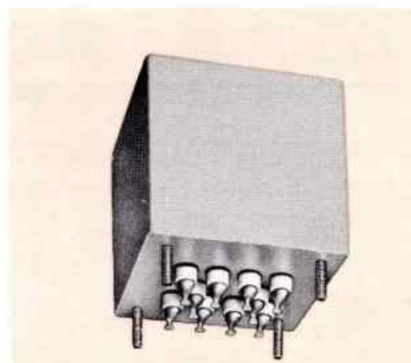
High voltage, constant inductance, tapped inductor. 16 millihenries, 8 kHz, inductance variation less than 1% from 1 volt to 1600 volts. Q greater than 40 at 1600 volts. Case size: 3 1/16 x 3 1/16 x 2 3/4" high. Grade 4, MIL-T-27C.
