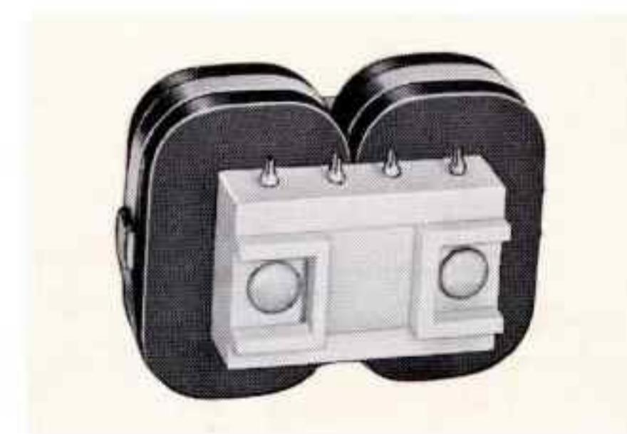
Molded High Temperature, High Voltage Transformer. Input 115 V 400 Hz, output 3400 V, 80 ma DC. Corona free molded terminals. MIL-T-27C Grade 5, Class T (170°C), 3¾ x 2¾ x 2¾", 2 lbs. 10 oz.
