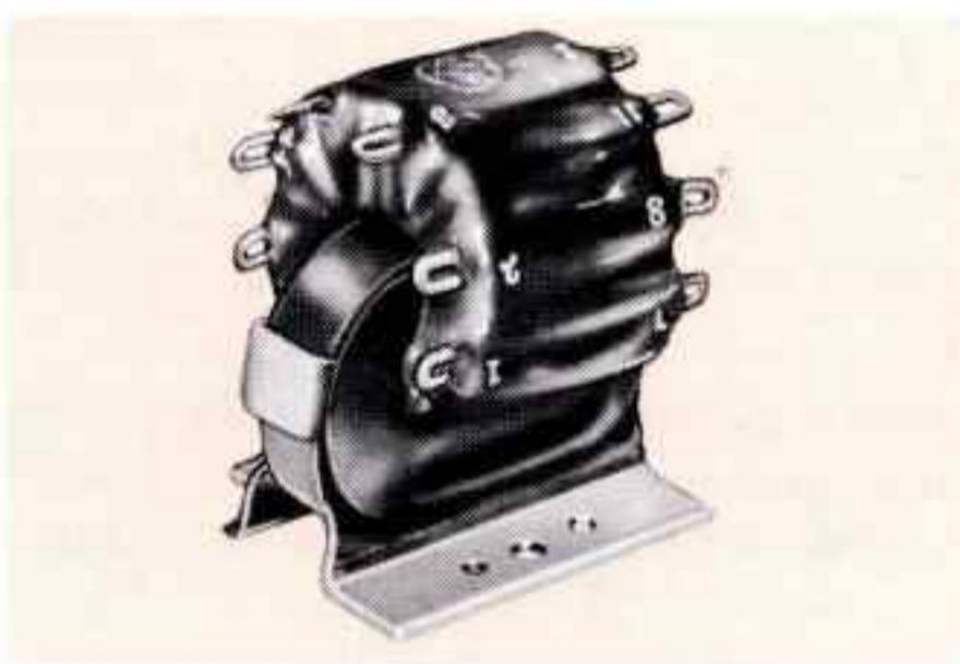
High temperature power transformer. Primary 115 V., 320/1000 Hz to four 6.3 V. and one 475 V. secondaries. 200° C. MIL-T-27C; 2¼ x 2 x 2", 9 ounce.
