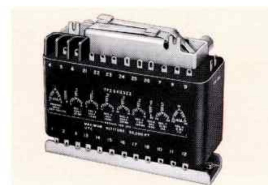
Molded Power Transformer 3 Phase. Input 200V, 380-420 Hz Electrostatic Shield, 8 output windings. 26 terminals. MIL-T-27C, Grade 2 Class S. Max. Alt. 50K Ft. Size 6 x 2½ x 5", 8 lbs.
