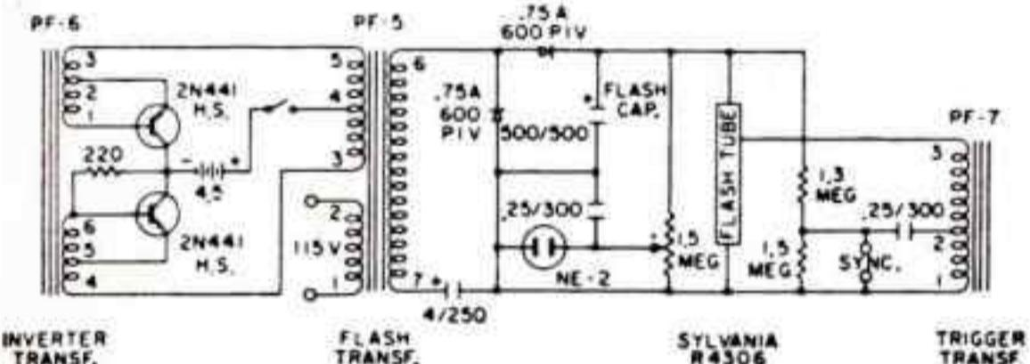
Miniaturized light weight units for transistor type photoflash supply.
