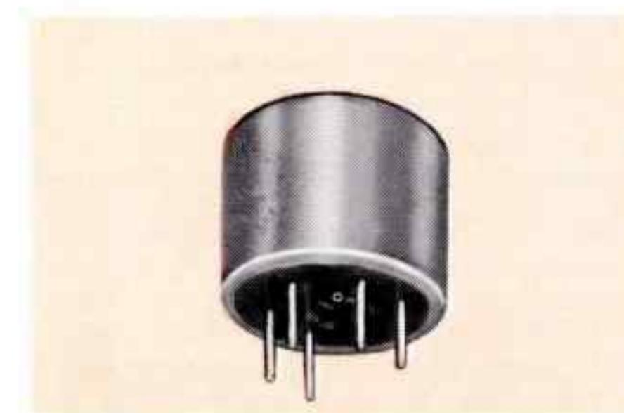
Molded carrier frequency transformer, + 8 dbm level. Within 3 db from 100 Hz to 100 kHz. 4000:4000 ohms.  $\frac{3}{4}$  Dia. x  $\frac{5}{8}$  inches,  $\frac{1}{3}$  oz.
