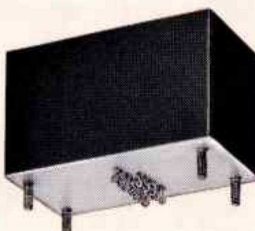
Precision Magnetic Modulator and Filter to produce sine wave output directly proportional to a DC control input. Temperature stabilized from -55°C to 85°C. Distortion and linearity less than 3% thru temperature and frequency range of 380-420 Hz. MIL-T-27C, 1½ x 1¾ x 3⅜", 12 oz.
