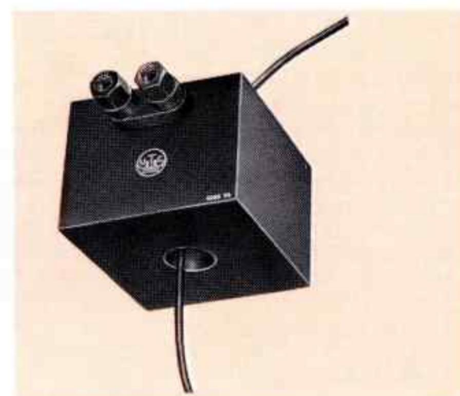
Current Transformer with 1 K load exhibits 1 V/amp/turn sensitivity. From 400 Hz to 30 kHz,  $\pm 0.1$  db. Good linearity with both current, 1 mA-10 A; and turns, 1-5 T.
