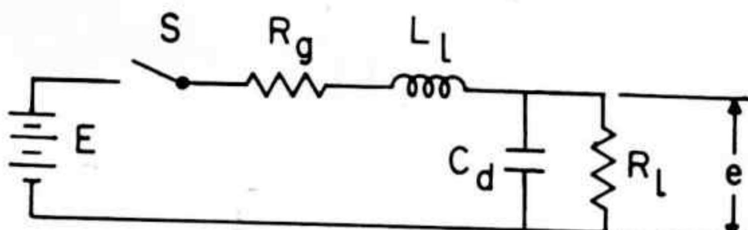
This circuit was obtained from the generalized transformer equivalent circuit by eliminating all components that are not effective at high frequency.
