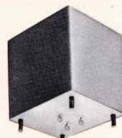
High pass filter, 30 Hz, used to eliminate from the output, 25 Hz sine wave pulses which control automatic programming on audio tracks of music tapes. Flat to 1 db from 50 Hz to 15 kHz, within 3 db to 30 Hz. Attenuation of at least 35 db from 25 Hz to 20 Hz. Source and load 600 ohms. Wt. approx. 6 lbs. MIL-F-18327C.
