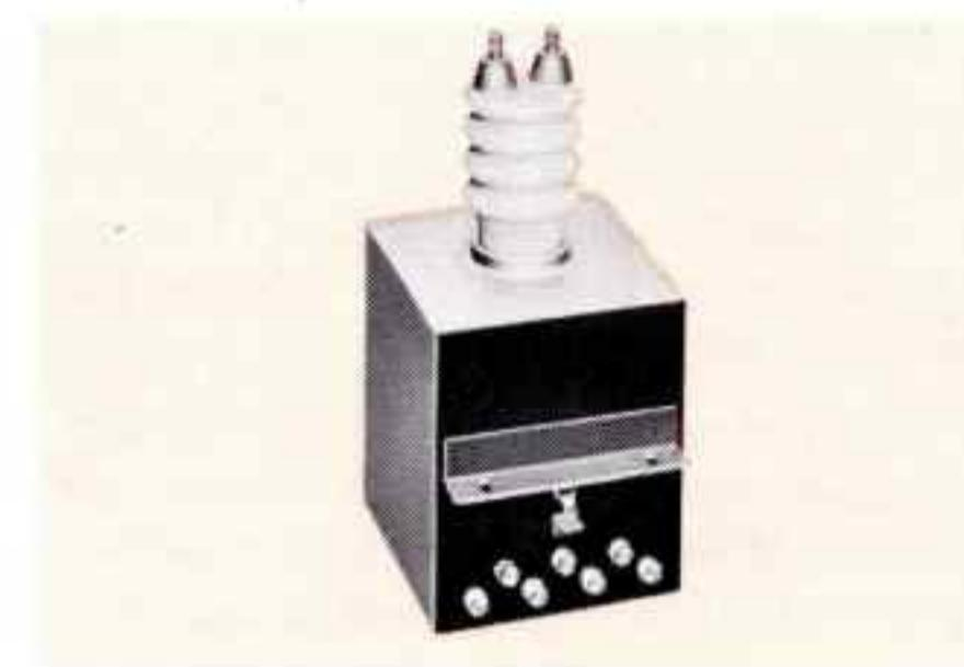
Low capacity current limiting filament transformer. Primary 118 V. 60 Hz to 6.3 V. at 3 A., 8 A. at short circuit. 25 MMFD capacity, 30 KV hipot and 200:1 capacity divider; 5 x 3¾ x 4½", 9 lbs.
