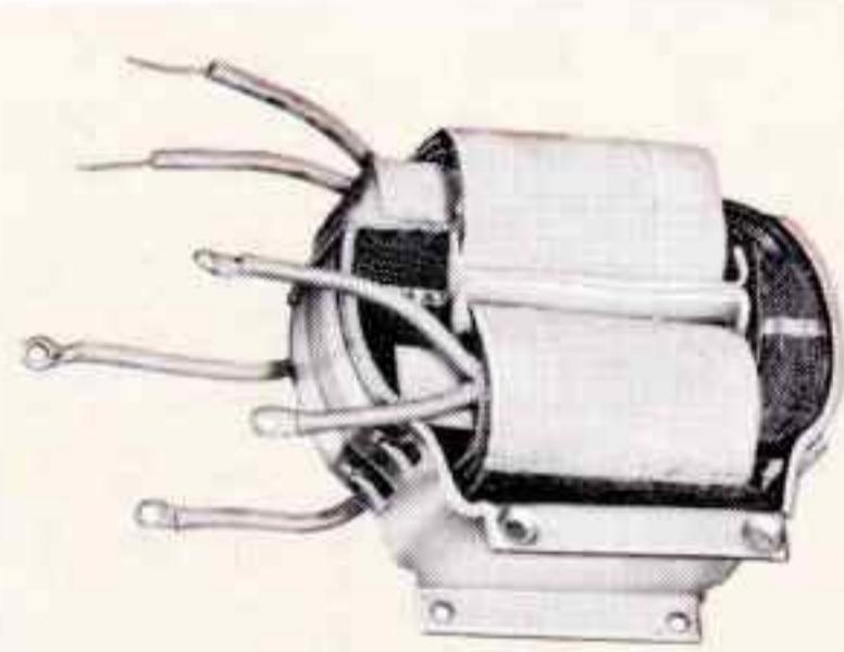
Output to magnetron. Input 6 KV peak 2.5  $\mu$ sec. or .5  $\mu$ sec. Output 28 KV-27 A. peak and 14.2A. bifilar magnetron filament winding. MIL-T-27C, 170° C.; 2 $\frac{5}{8}$  x 5 $\frac{3}{8}$  x 4 $\frac{5}{8}$ , 7 $\frac{1}{2}$  lb.
