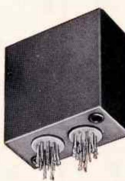
Precision reference transformer. Input 14 V., 400 Hz. Twelve secondaries held to low phase shift and .1% tolerance MIL-T-27C; 1¾ x 2 x 1¾, 4.5 oz.
