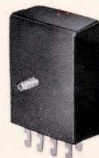
Ferrite core pulse transformer. 30 V. . . . three windings, 5-10  $\mu$ sec. Couples to magnetic tape head for high speed read in and out. Hipermalloy shield. Commercial; 5/8 x 1 $\frac{1}{4}$  x 1 $\frac{5}{8}$ , 2 oz.
