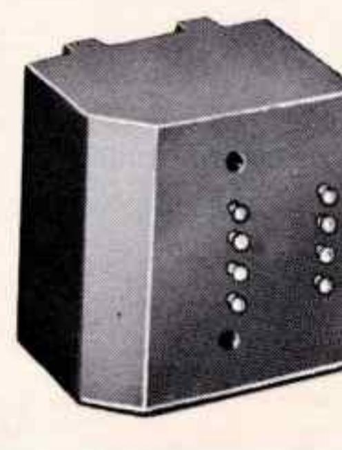
Dual saturable reactor. Input 10 V. - 1 kHz. Output 3.5 V. 2 MA DC control current. 130° C. MIL-T-27C; 1¾ x 1¾ x 1¼, 5 oz.
