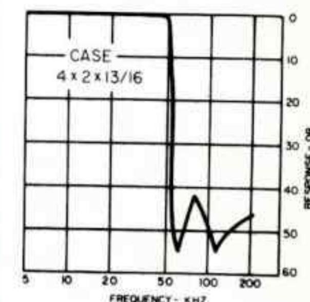
Sharp cutoff 49 kHz low pass filter. Stable to .1 db in pass band from 0°C. to 85°C. Within 1 db 5 kHz to 49 kHz, over 40 db at 56 kHz. MIL-F-18327C; .6 lbs.
