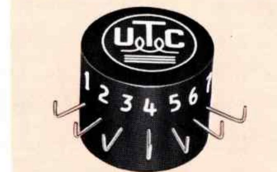
Instrument reference transformer. To operate from 15 kHz to 20 kHz with 12.5 V on one half of primary and to deliver 9.0 V on each half of secondary; secondary halves loaded with different impedances. Size: 1.1 Dia. max. x .79" high max. Weight: 34 gms.
