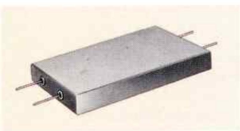
Ultra-miniature low pass filter only 1/4" high. DC to 40 kHz within  $\pm 0.1$  db, within 1 db to 60 kHz, 3 db to 70 kHz. Attenuation of at least 40 db above 81 kHz. Source and load 1K ohms. MIL-F-18327C. Wt. 1.2 ounces.
