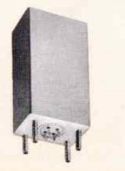
Miniaturized receiving filters, available from 425 Hz to 3315 Hz. Within 3 db at  $\pm 42.5$  Hz and attenuation of at least 36 db at  $\pm 130$  Hz. Source and load 600 ohms. Wt. approx.  $\frac{3}{4}$  lbs.
