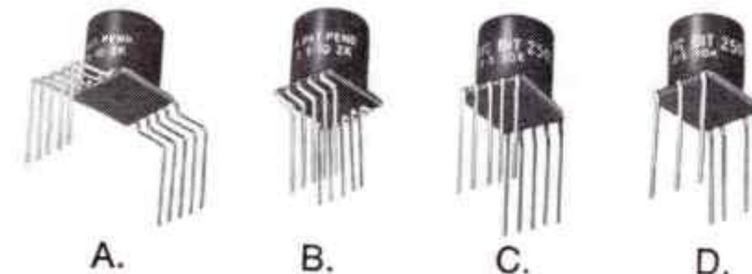
BIT-250 stock units are manufactured with Flat Pack type terminations extending outward. Terminations may be bent for adaptation to plug-in applications. Unique termination configuration isolates strain and affords safety during bending process. Variations of bends are pictured above.
