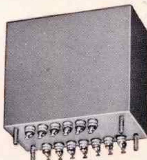
Servo reference transformer. Input 120 V., 380 to 420 Hz. Output ratios under load held to .005% tolerance. Phase shift .05° max. MIL-T-27C; 2¼ x 1¾ x 2, 12 oz.
