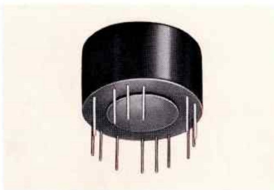
Self-saturating inverter transformer; 100 V DC input. Frequency of oscillation 20 kHz. MIL-T-27C, Class T. Size: 1.25 Dia x .60 H, PC mounting.
