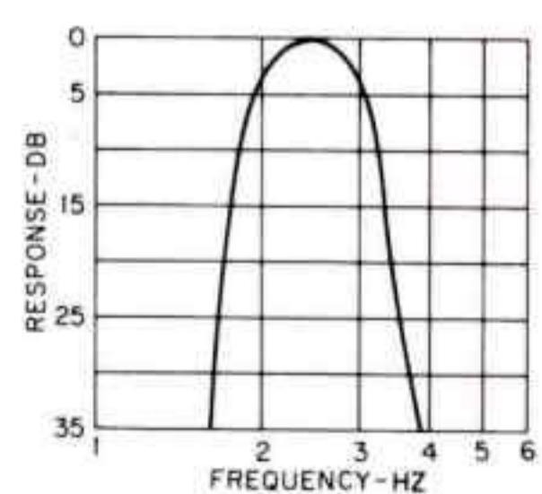
Low frequency band pass filter. From 2 to 3 Hz within 3 db. At 1.5 Hz and lower, and 4 Hz and higher, greater than 30 db. Source and load 10K ohms. MIL-F-18327C. Wt. 12 3/4 lbs. MA case, 4 x 4 1/16 x 6".
