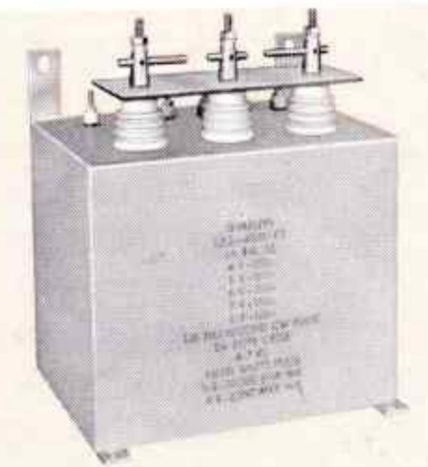
Sonar Output Transformer. 36 KW pulses, 100 millisec @ 5% duty cycle. Input 4K  $\Omega$  CT, output 120-180  $\Omega$ . Hipot 29 KV. Hermetic, MIL-T-27C Grade 4, 6 $\frac{1}{2}$  x 9 x 8", 37 lbs.
