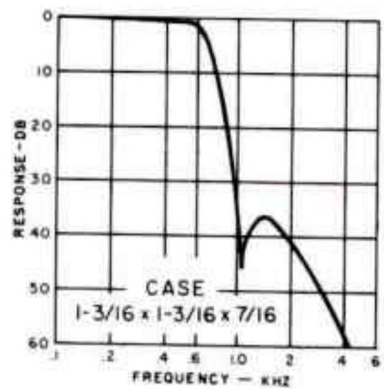
Telemetering low pass filter 560 Hz. Available from 400 Hz to 70 kHz.  $\pm 7.5\%$  bandwidth flat to 1 db. Attenuation greater than 35 db beyond the 2nd harmonic of  $-7.5\%$  frequency. Impedance 47K ohms. MIL-F-18327C. Wt. 0.8 oz.
