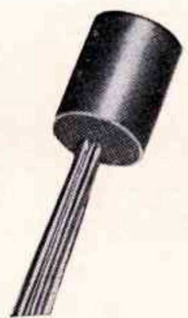
DO-T Pulse Transformer, width 150  $\mu$ sec., ratio 1:1:1. Transistor output to gating circuits. -65° C to 105° C. MIL-T-21038B. 5/16 Dia. x 13/32, 1/10 oz.
