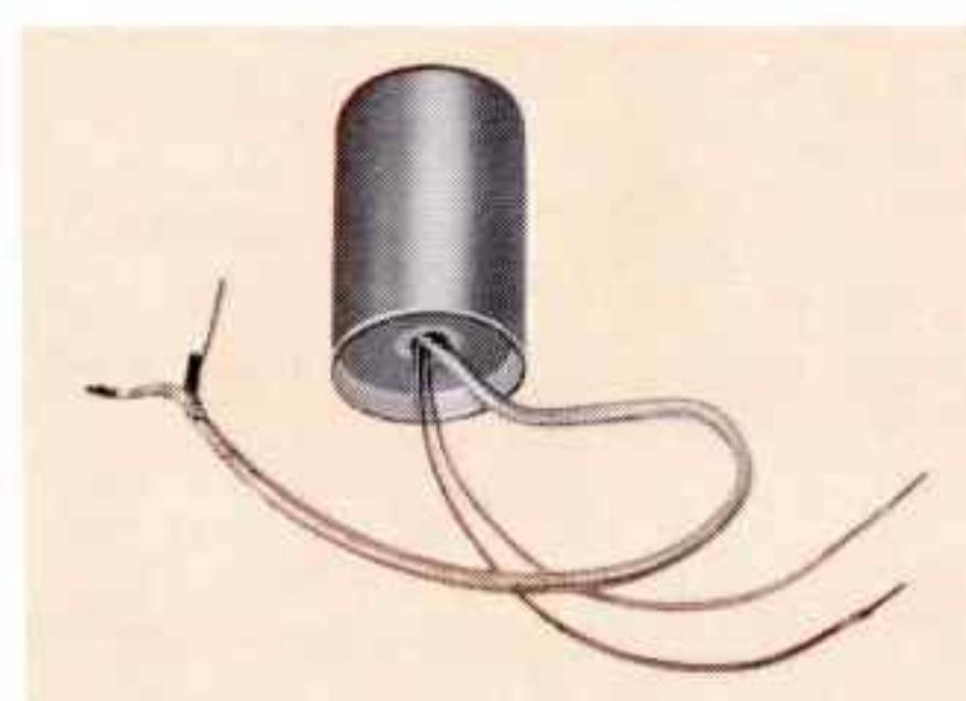
Microphone input transformer, double drawn hipermalloy shields. Shielded cable leads. Ratio 100:1.  $1\frac{1}{16}$  Dia. x  $1\frac{1}{32}$  high. Inductance greater than 1000 Hys. at 60 Hz.
