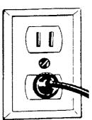
Insert the line cord into a 110-120 volt 60 cycle power source. 2
