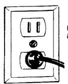
Insert the line cord into a 110-120 volt 60 cycle power source. 2
