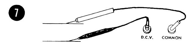
Connect the test-leads across the voltage to be measured.
