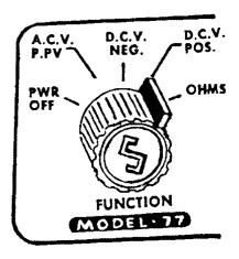
Put the instrument "on" by turning the function switch to the "positive volts" position.
