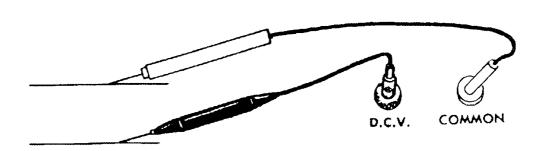
Connect the test leads across the circuit to be measured.
