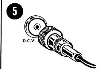
Connect the "DC Volts" lead to the DC Volts connector at the lower center of the panel.
