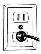
Insert the line cord into a 110-120 volt 60 cycle power source.
