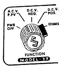
Place the instrument "on" by turning the selector switch to the "ohms" position.
