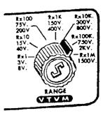
Set the "range" selector switch to the range desired. When in doubt, use the highest range.
