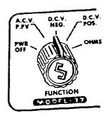
Put the instrument "on" by turning the function switch to either the "positive volts" or "negative volts" position.
