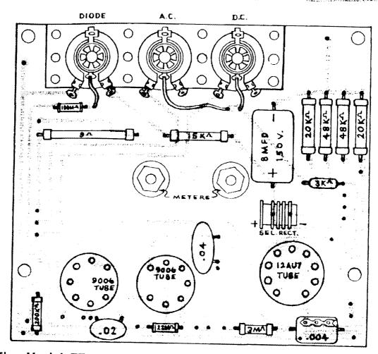
The Model 77 utilizes the latest development in printed circuitry. All the components on the printed board are mounted below the board for protection except the 3 controls.
