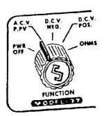
Put the instrument "on" by turning the function switch to the "AC-volts" position.
