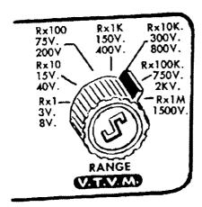
Set the "range" switch to the range desired. Since the meter is already reading at half scale, all ranges will be 1/2 of the markings appearing on the range switch.
