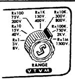
Set the "range" selector switch to the range desired. When in doubt use the highest range.
