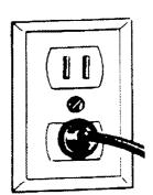
Insert the line cord into a 110-120 volt AC power source. 2
