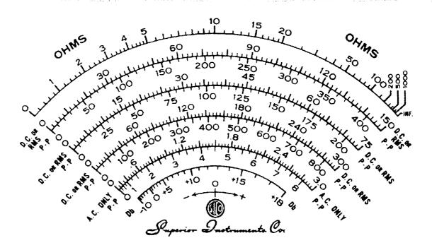
The Model 77 meter face contains the 7 main calibrated scales that are used for all measurements. Four of the scales are dual scales printed in black and red.
