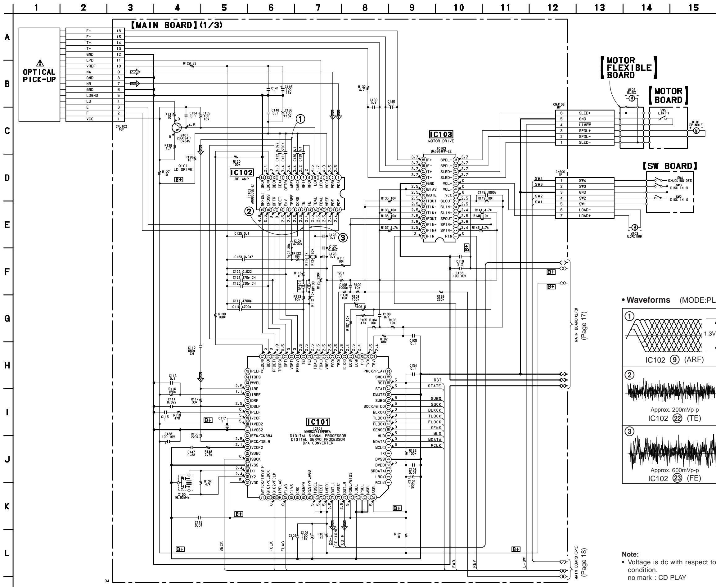
**3-6. SCHEMATIC DIAGRAM — MAIN SECTION (2/3) —** • Refer to page 22 for IC Block Diagrams
