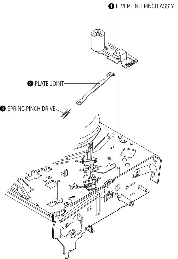
Fig. 1-24 Lever Unit Pinch Ass'y, Plate Joint, Spring Pinch Drive Removal
