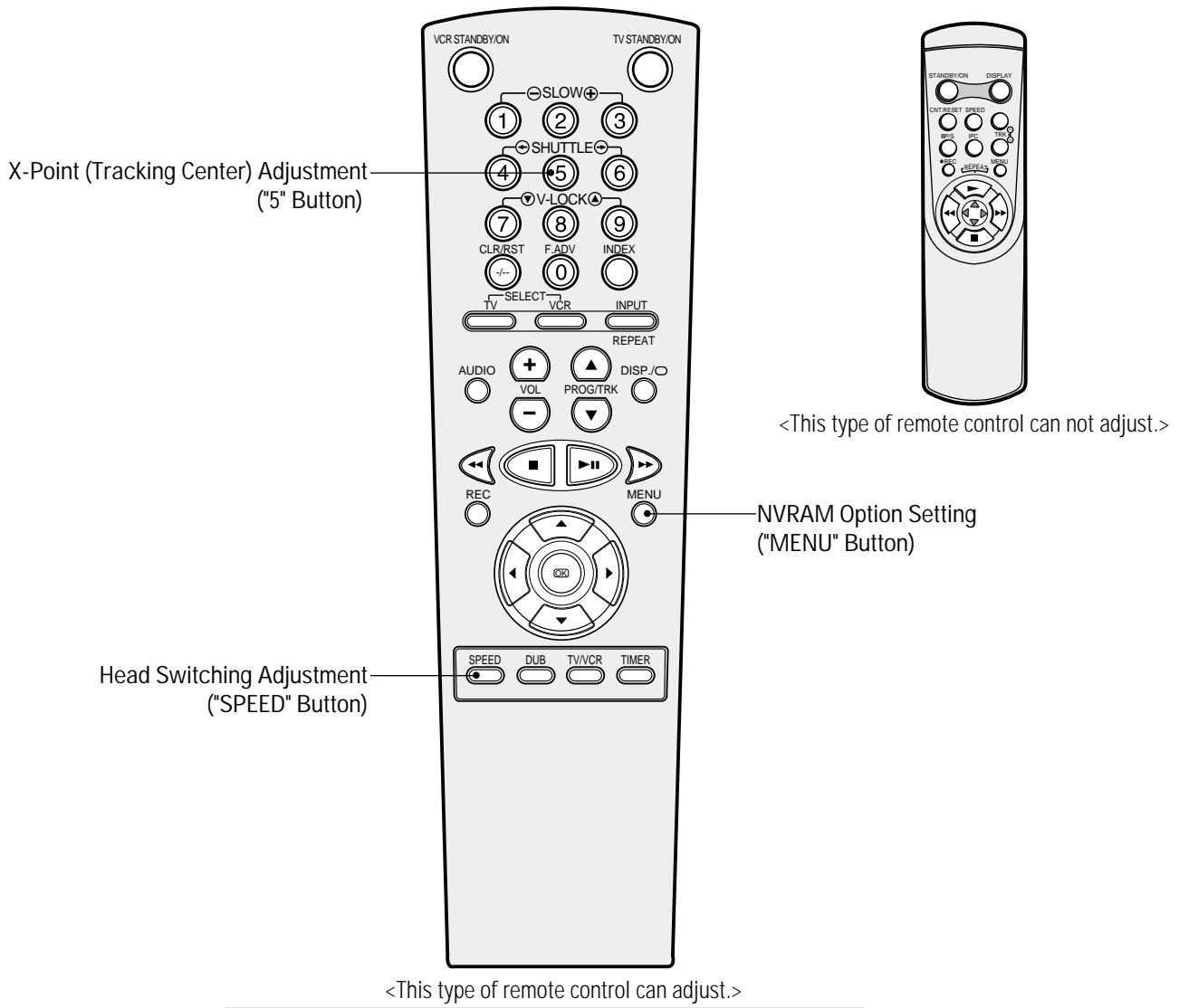
Remote Control for adjustment is not supplied as a Service Jig.
