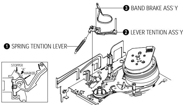
Fig. 1-16 Lever Tension Ass'y,
