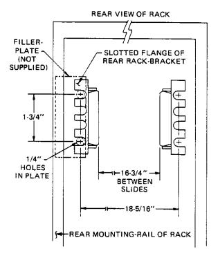
Figure 2-7, Rear End Slide-Mount Rack Dimensions
