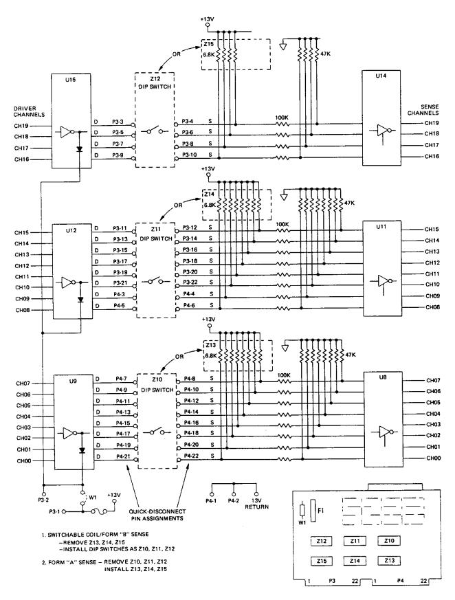
Figure 3-5, 1250-15 Relay Driver Connection Diagram
