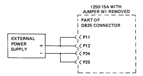
Figure 3-14, 1250-15A Using an External Power Supply
