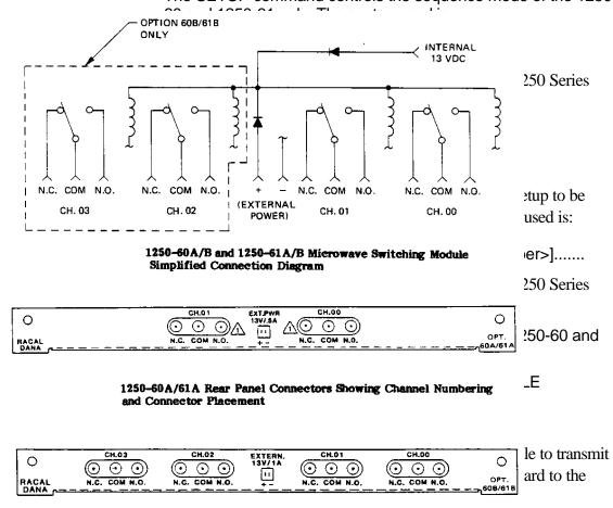
1250-60B/61B Rear Panel Connectors Showing Channel Numbering
