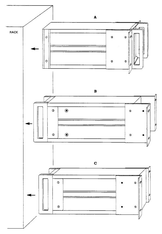
Figure 2-8, Standard (A) and Optional Rear-Forward Rack-Mount (B and C) Assembly-to-Instrument Configurations
