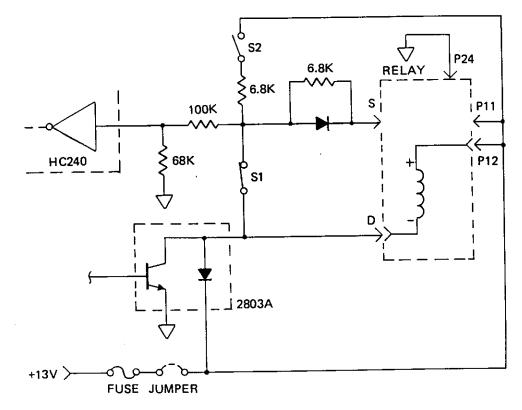
Figure 3-12, 1250-15A Coil Current Sense
