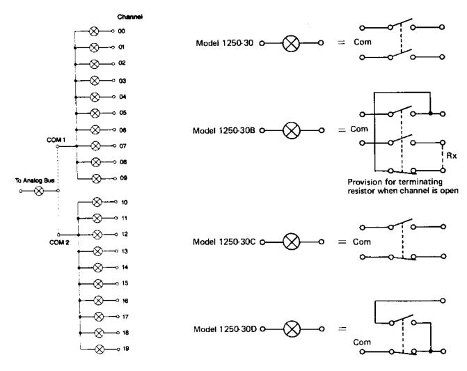
Figure 1-9, Block Diagram of 1250-30 Series
