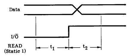
$t_{1}$  is the time from output disabled until  $I/\overline{O}$  equals the input (90  $\mu s$  typical)
