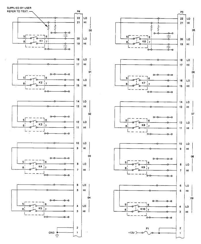
Figure 3-19, 1250-20 Relay Power Module Connection Diagram
