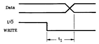
$t_1$  is the time from when  $I/\bar{\rm O}$  equals output until the output is enabled (250  $\mu s$  typical)
