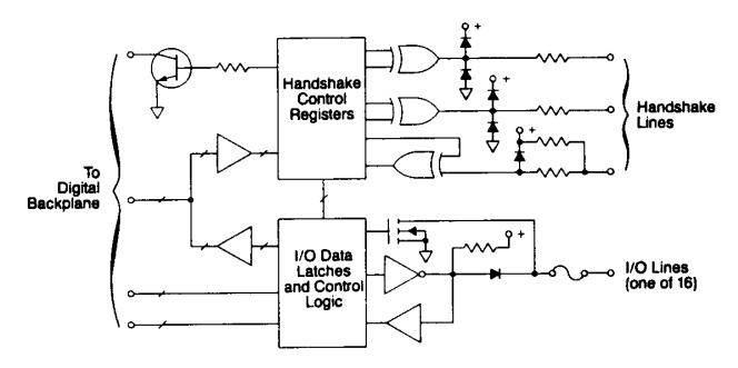
Figure 1-5, Block Diagram of 1250-14
