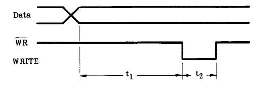
$\mathbf{t_1}$  is the time from data valid (output enabled) to the start of strobe (90  $\mu s$  typical)
