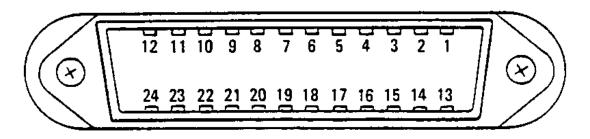
Figure 2-5, GPIB-Connector (Rear Panel)
