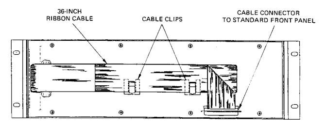
Figure 2-12, Rear View of Option 90 Showing Ribbon Cable
