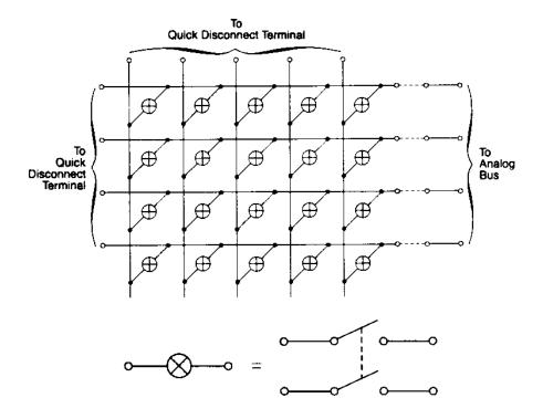
Figure 1-11, Block Diagram of 1250-40
