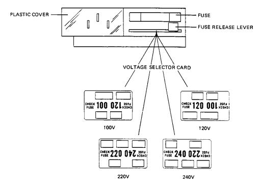
Figure 2-1, AC Line Voltage Selection
