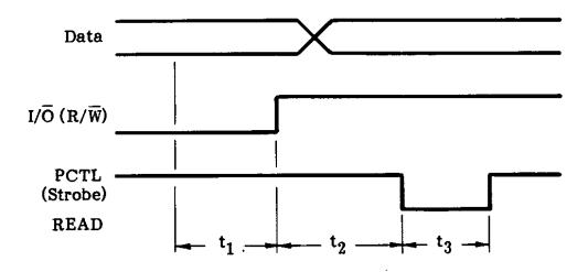
$t_1$  is the time from output disabled until  $I/\overline{O}$  equals the input (100  $\mu s$  typical)
