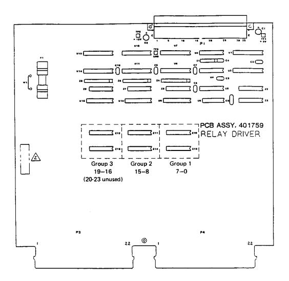
This example of Form A, B, and C sensing uses the 3 different channel groups 1, 2, and 3 on Relay Driver PCB shown above. See text for configuring to meet your particular needs.
