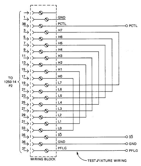
Figure 4-1, 1250-14 Test Configuration
