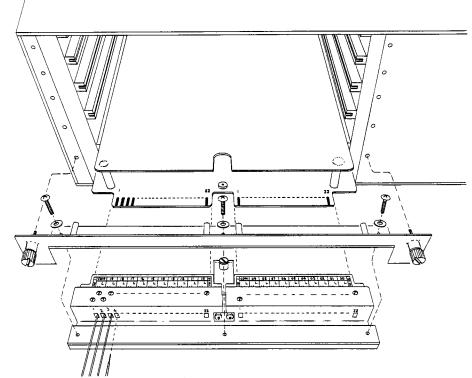
Figure 2-2, 1250 Switching Module Installation
