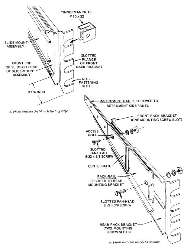
Figure 2-6, A & B Slide-Mount and Bracket Assembly
