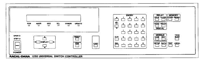
Figure 1-2, 1250 Option 90, Intelligent Front Panel
