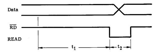
$t_1$  is the time from output disable to the start of strobe (80  $\mu$ s typical)
