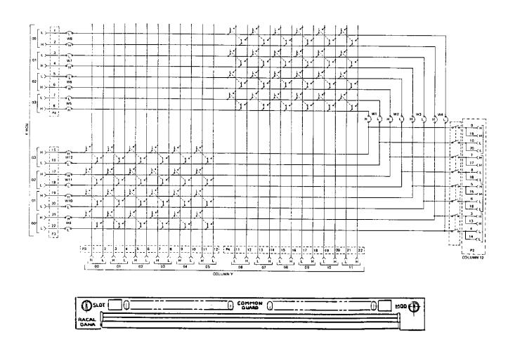
Figure 3-25, 1250-45 Block Diagram
