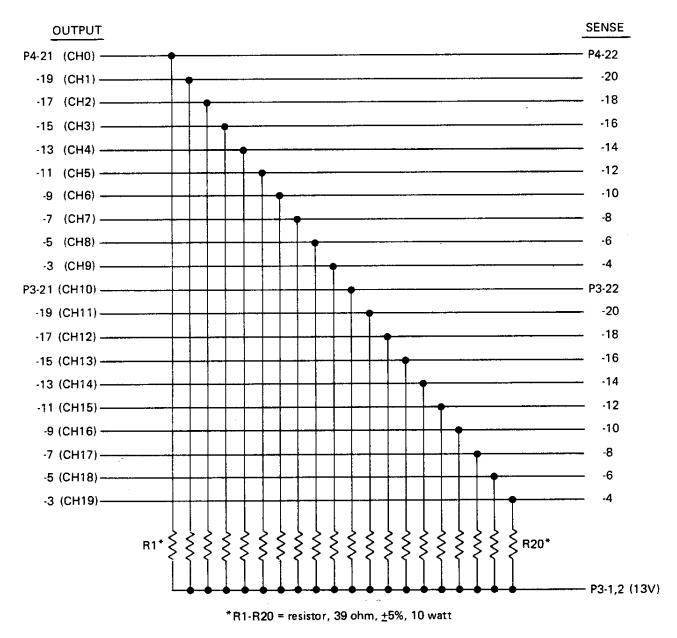
Figure 4-4, 1250-15 Test Configuration
