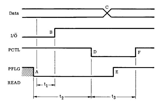
$t_1$  is the time from output disabled until when  $I/\bar{O}$  equals the input (100 µs typical)
