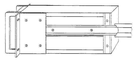
Figure 2-9, Slide Assembly-to-Side Channel Installation
