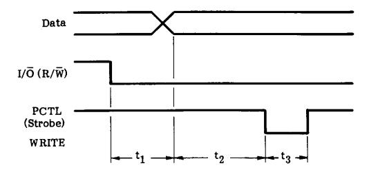
$t_1$  is the time from when  $I/\bar{O}$  equals output until the output is enabled (260 µs typical)
