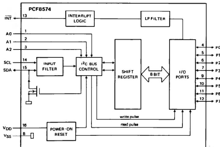
Figure 3.24 Block diagram
