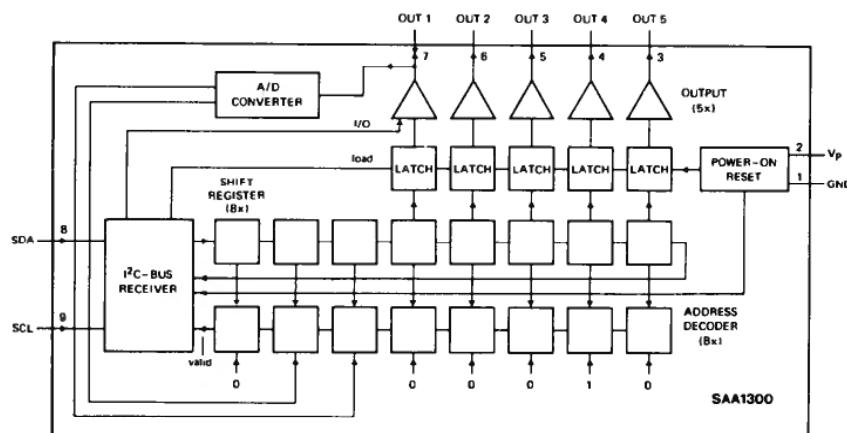
Figure 3.23 Block diagram
