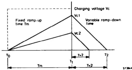
Figure 3.8 Dual slope system
