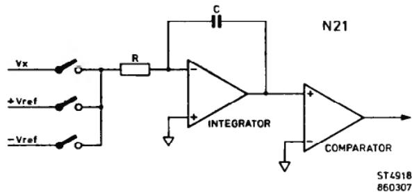
Figure 3.9 ADC principle
