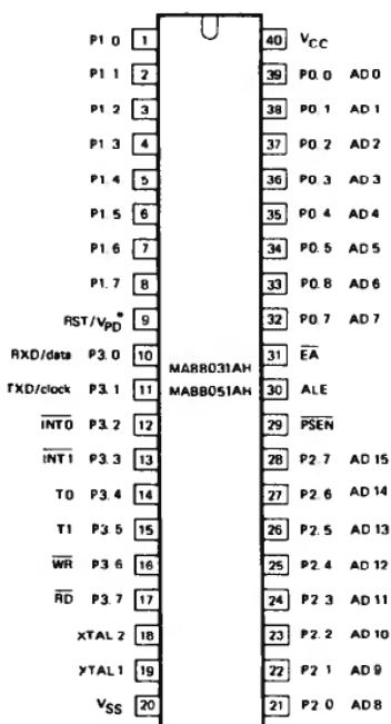
Figure 3.13 Pin Configuration
