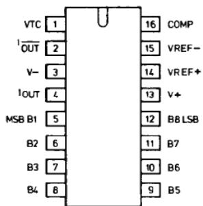
Figure 3.16 Pin connections
