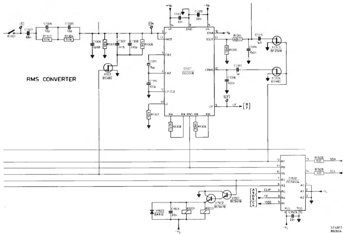
Figure 3.6 RMS converter
