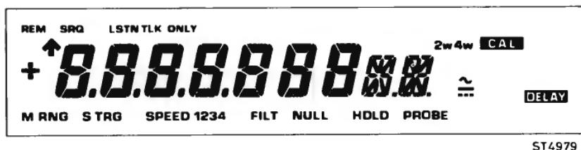
Figure 6.7 PM2534 display in display test
