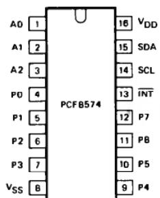
Figure 3.25 Pinning diagram
