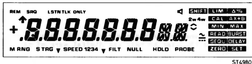
Figure 6.8 PM2535 display in display test
