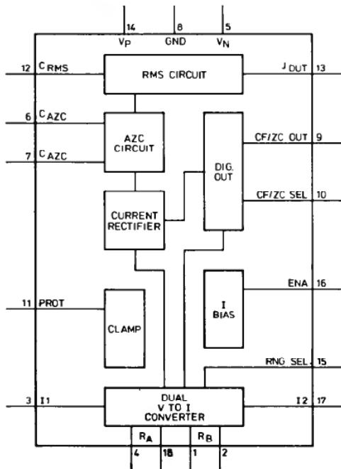
Figure 3.26 Block diagram OQ0068A
