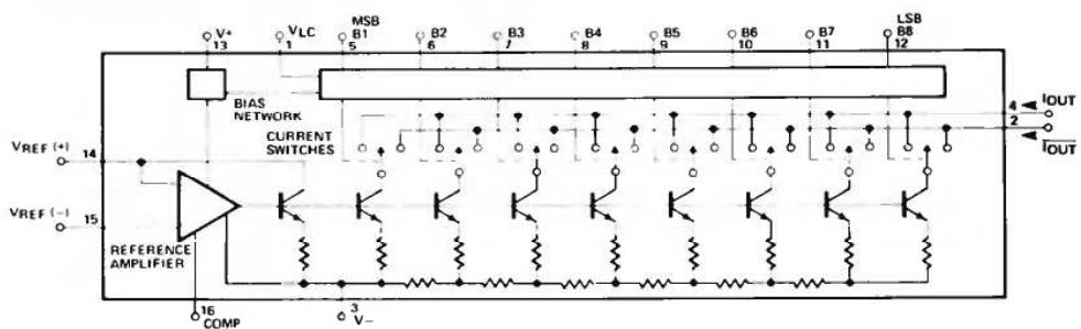
Figure 3.15 Block diagram
