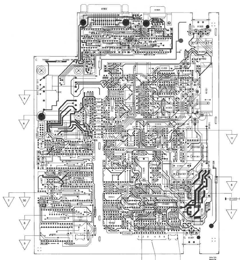
Figure 9.8 Main pcb version 4022 325 8051.2, component side
