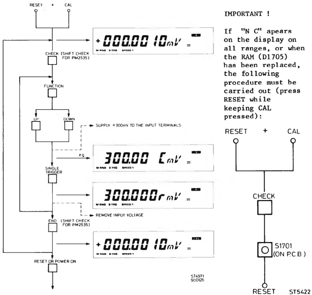
Figure 5.1 Calibration adjustment procedure
