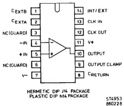
Figure 3.28 Pin connections
