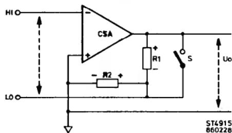
Figure 3.4 DC amplifier principle
