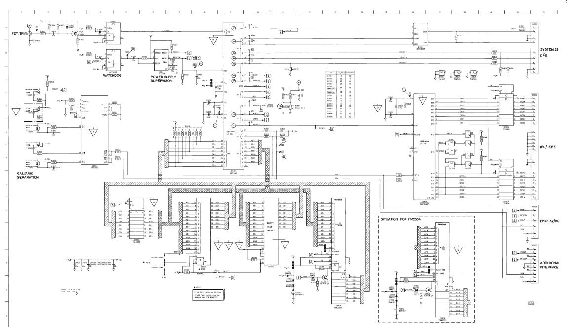
Figure 9.6 Main pcb, digital part circuit diagram
