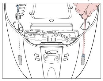
3. If all the screws (step 1 and 2) are removed, next step is to find the hidden snap locks were the housing is connected to the upper Grey top ring.
