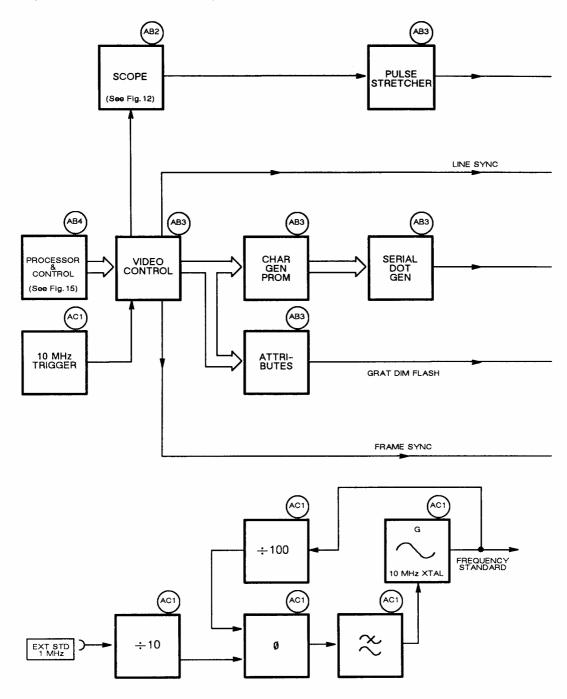
Fig. 4-14 Block diagram of video control and freq. standard (showing main functions of boards)
