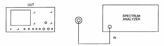
Fig. 5-1-24 Test equipment connections for RF generator RF leakage performance checks
