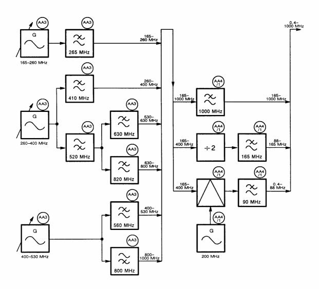
Fig. 4-5 RF synthesizer frequency generation summary (switching omitted for the sake of clarity) - AA3, AA4/1
