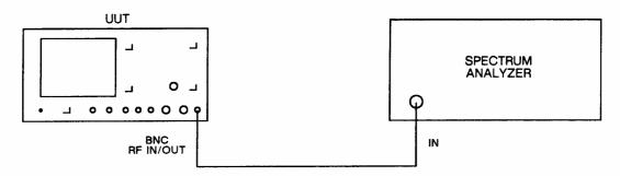
Fig. 5-1-26 Test equipment connections for RF generator harmonics, sub-harmonics & spurious signals performance checks
