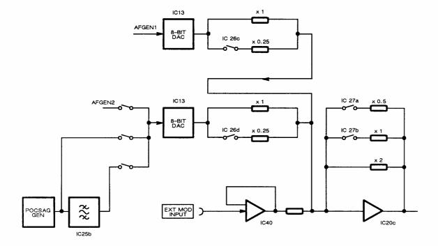
Fig. 4-8 Level control switching - AB6/1
