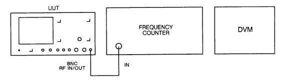
Fig. 5-2-4 Test equipment connections for adjusting C79 on AA4/1
