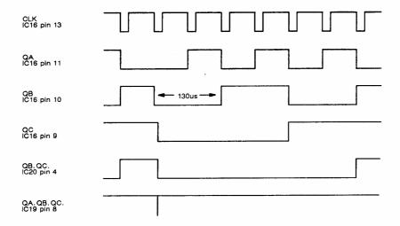
Fig. 5-3-4 Columns counters timing waveform diagram for AB3/2
