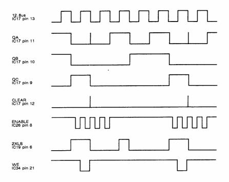
Fig. 5-3-3 Rows counters timing waveform diagram for AB3/2
