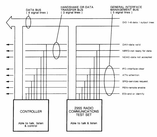
Fig. 4-17 General Purpose Interface Bus (GPIB) structure
