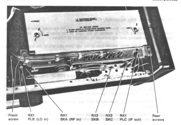
Fig. 5-0-1 Receiver tray assembly RX1 in normal position
