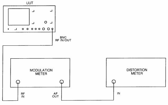
Fig. 5-1-22 Test equipment connections for RF generator AM & FM distortion performance checks
