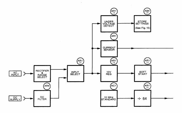
Fig. 4–19 Block diagram of power supply (showing main functions of boards)
