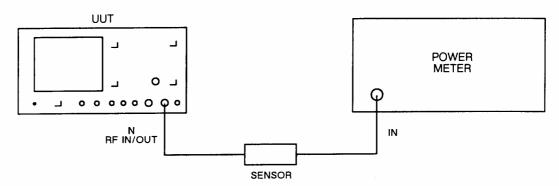
Fig. 5-2-11 Test equipment connections for adjusting R20 on AB6/1
