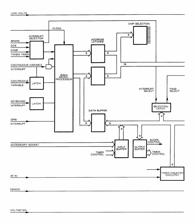
Fig. 4-16 Block diagram of Microprocessor board AB4/1
