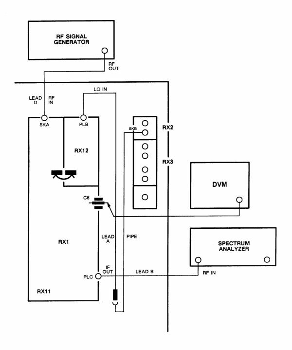
Fig. 5-2-20 Connections for AGC and 38 dB amplifiers
