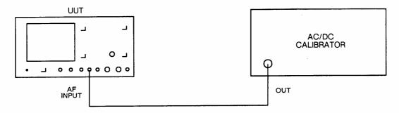
Fig. 5-2-5 Test equipment connections for adjusting R231 on AB5/1
