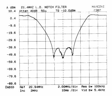
Fig. 5-2-16 Response of 21.4 MHz LO notch filter
