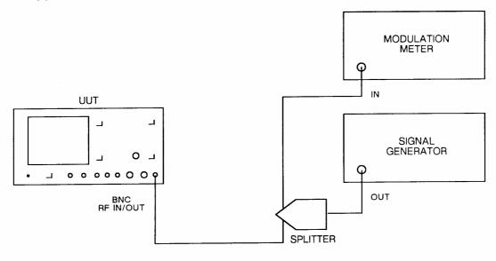
Fig. 5-1-4 Test equipment connections for modulation meter AM & FM monitor accuracy performance checks
