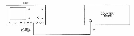
Fig. 5-1-14 Test equipment connections for AF generator frequency accuracy performance checks
