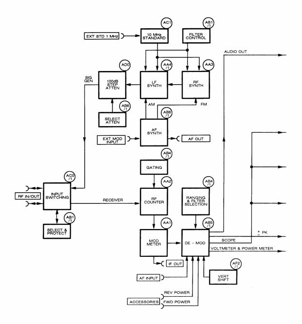
Fig. 4-1 Block diagram of the 2955A
