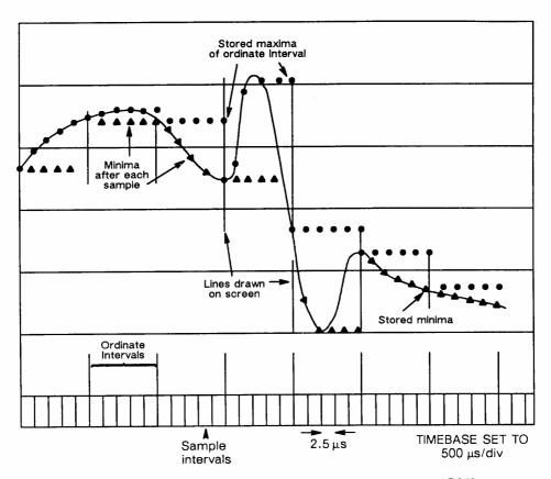
Fig. 4–13 Oscilloscope display generator process – AB2/2
