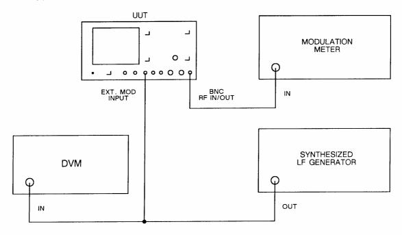
Fig. 5-1-23 Test equipment connections for RF generator external AM & FM performance checks
