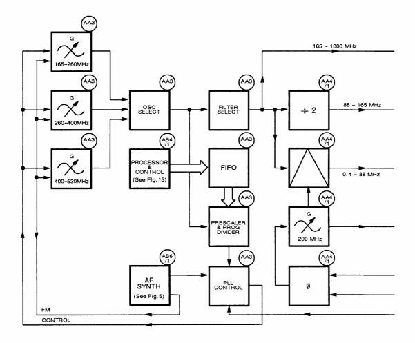
Fig. 4-3 Block diagram of RF and LF synthesizers (showing main functions of boards)
