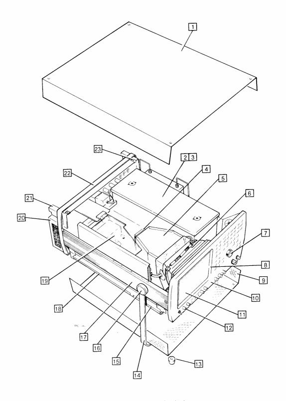
Fig. 6-1 Miscellaneous mechanical parts
