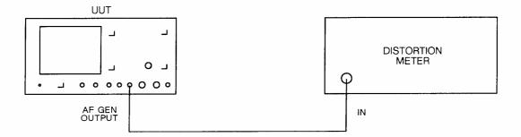
Fig. 5-1-13 Test equipment connections for AF generator distortion performance checks
