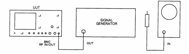
Fig. 5-2-2 Test equipment connections for adjusting R11 and R27 on AA1
