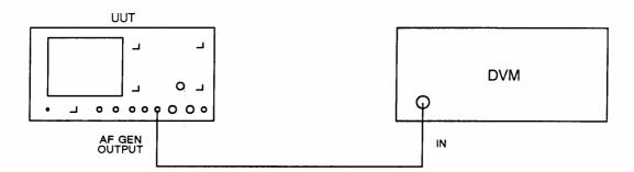
Fig. 5-2-10 Test equipment connections for adjusting R1 on AB6/1
