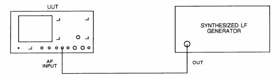
Fig. 5-2-6 Test equipment connections for adjusting R305 and R314 on AB5/1
