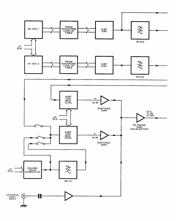
Fig. 4-6 Block diagram of AF synthesizer and modulation control
