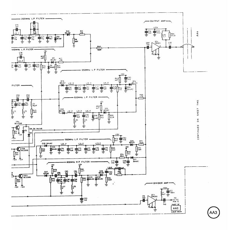
F synthesizer (oscillator & filters)
