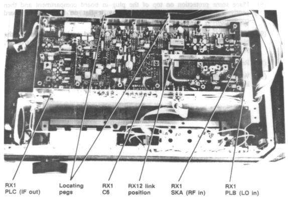
Fig. 5-0-2 Receiver tray assembly RX1 with lid removed
