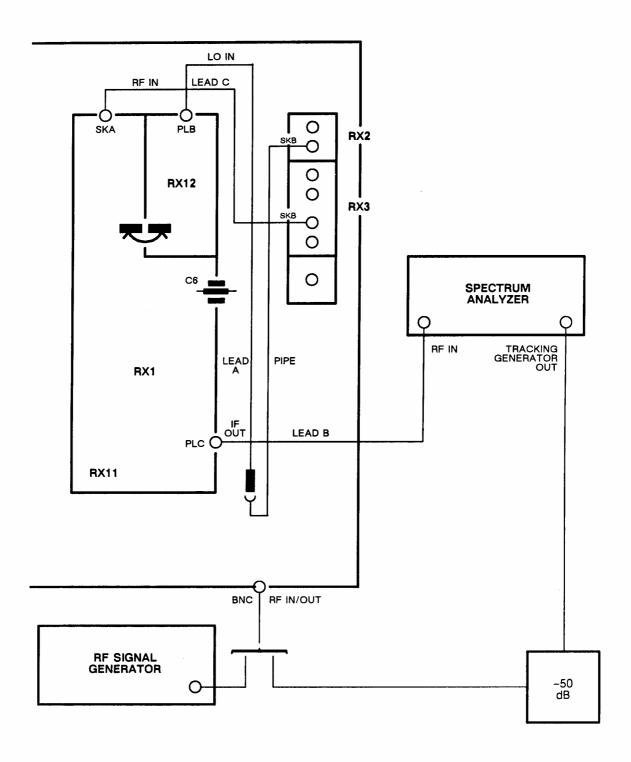
Fig. 5-2-17 Connections for checking 20 dB IF 180 kHz band-pass amplifier
