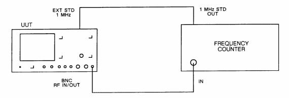
Fig. 5-1-20 Test equipment connections for RF generator RF accuracy performance checks
