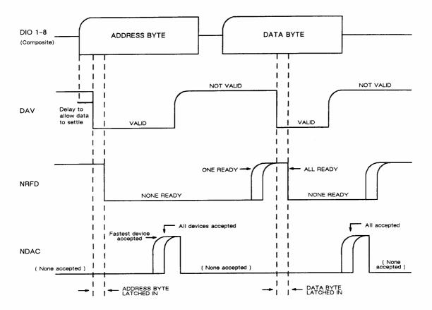
Fig. 4-18 Handshake procedure
