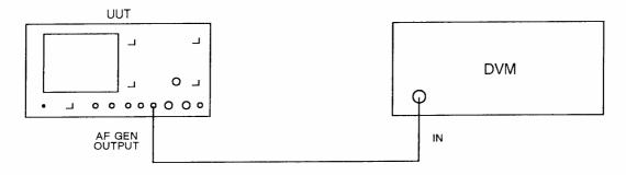
Fig. 5-1-12 Test equipment connections for AF generator output level accuracy performance checks
