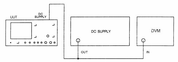
Fig. 5-2-14 Test equipment connections for adjusting R46 on AR1
