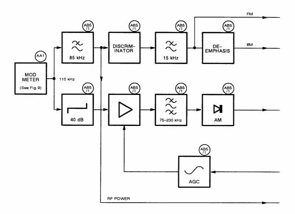
Fig. 4–10 Block diagram of demodulator, voltmeter and power meter (showing main functions of boards)
