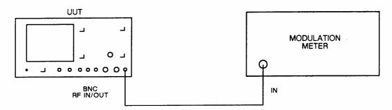
Fig. 5-1-25 Test equipment connections for RF generator FM on CW performance checks
