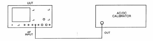
Fig. 5-1-7 Test equipment connections for voltmeter DC & AF level accuracy performance checks
