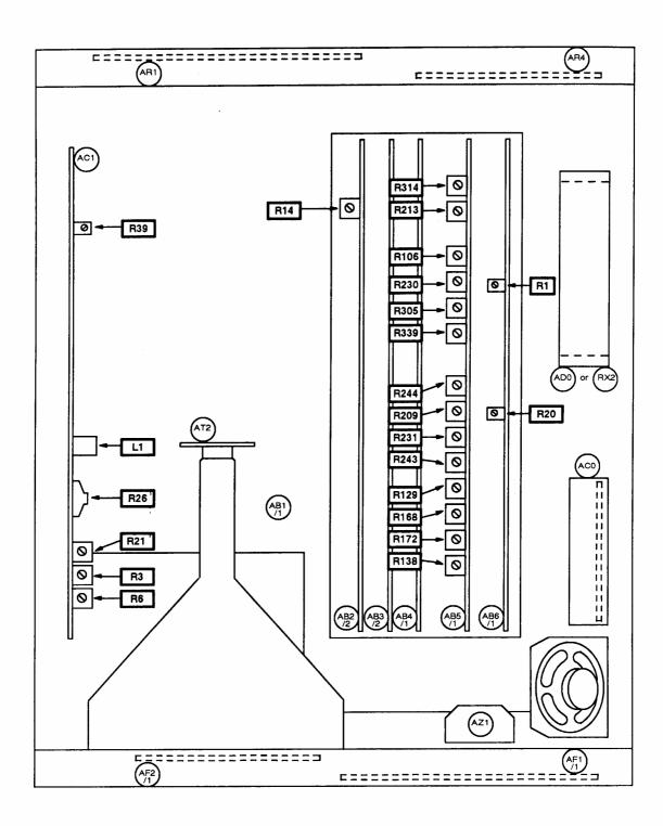
Fig. 5-2-1 Adjustment points accessible from above the instrument
