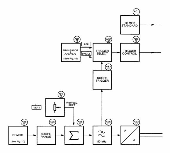
Fig. 4-12 Block diagram of oscilloscope (showing main functions of boards)
