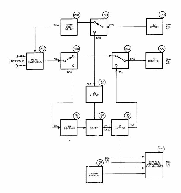
Fig. 4-20 Block diagram of the 2955R
