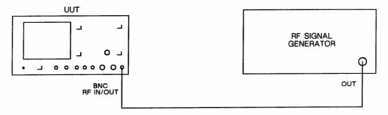
Fig. 5-1-28 Test equipment connections for 2955R level accuracy check
