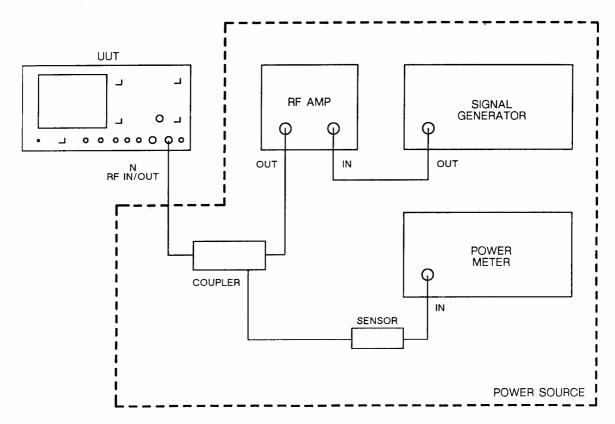
Fig. 5-1-17 Test equipment connections for RF power meter measurement accuracy performance checks
