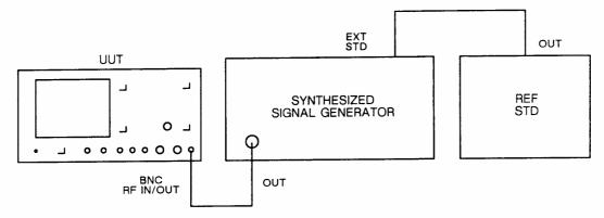
Fig. 5-2-13 Test equipment connections for adjusting R39 on ACI
