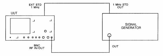
Fig. 5-1-9 Test equipment connections for RF frequency meter accuracy performance checks
