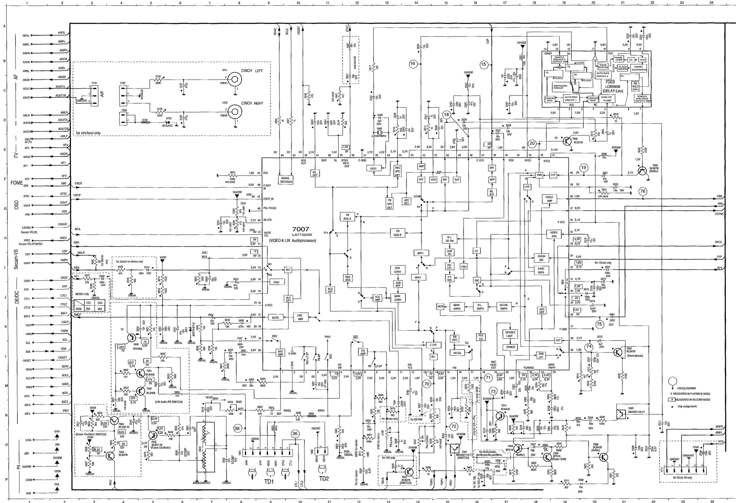
**Video Signal Processing Secam (VS\_S)**
