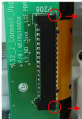
Separate the fixed Screw of Z-Board.
