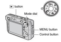
1 Recording: Turn on the camera, then set the mode dial. Playback: Press ▶.
