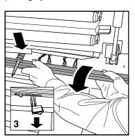
To disassemble the gas pressure springs (53), fold the canopy up and have a second person lock it in this position.
