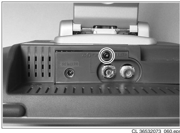
Figure 4-4 Rear cover removal hidden screw EU version
