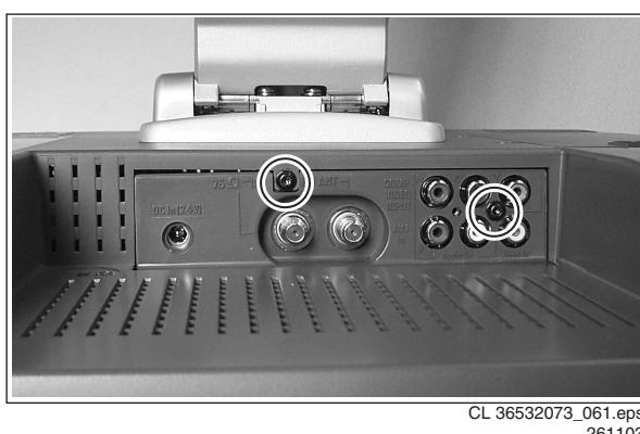
Figure 4-5 Rear cover removal hidden screws US version
