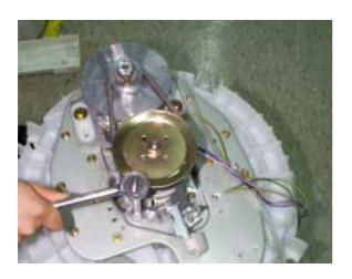
12) Pull out the gear mechanism ass'y.
