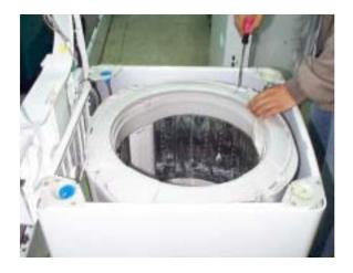
3 Remove the cap pulsator from the pulsator ass'y by using screw driver.
