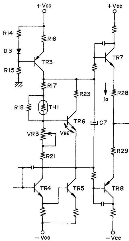
Fig. 6 Idling Current Supply Circuit & Temperature Compensation
