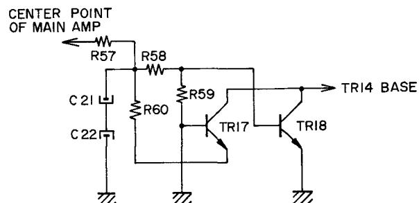
Fig. 10 Center Point DC Voltage Detection Circuit
