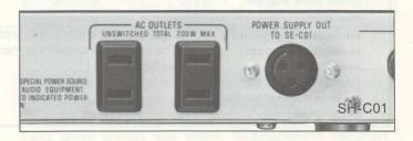
The equipment connected to these AC outlets are not affected by the setting of the power switch. Power is always available from these outlets. The total for the 2 outlets should not exceed 200 W.
