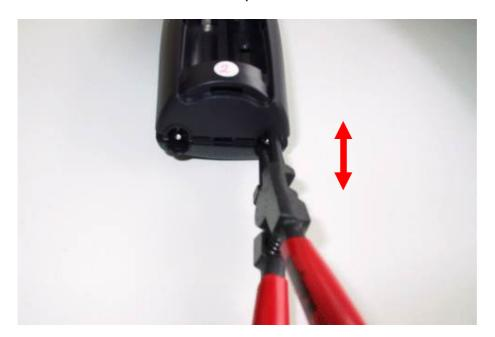
Insert pliers in charging-contact-hole and press to open lower part of the housing. If necessary do the same in the other charging-contact-hole.
