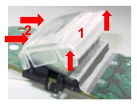
Snap the 2 hooks on the bottom open (1). Then lift the display carefully until the 2 snap hooks on the top open (2).
