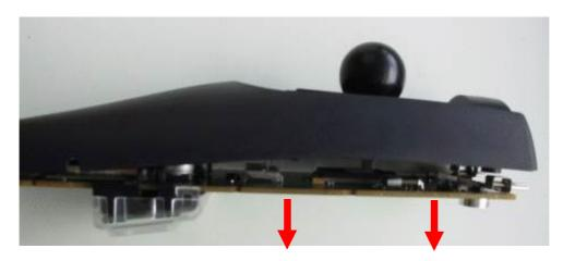
Insert battery dummy G3000 in battery compartment. Pull the board evenly in order to get upper and lower spring at the same time out of the battery compartment.
