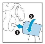
Turn the toothbrush upside down and press it down on a hard surface to remove the battery holder.
