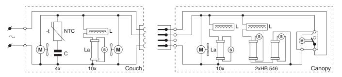
A burned NTC resistor or overheated wiring points to a wiring fault at the connecting block.
