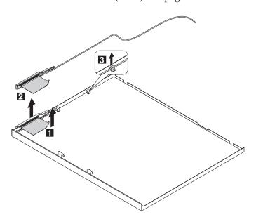
Note: For models with wireless WAN, the antennas present on the right-side are the aux wireless LAN antenna and the main wireless WAN antenna.
