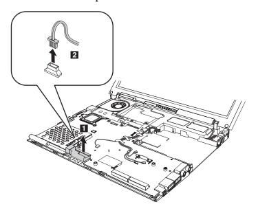
When installing: Make sure that the speaker connector is attached firmly.
