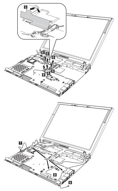
**Note:** For 802.11n wireless models, there is an additional white cable from the left side of the LCD instead of one **7**.
