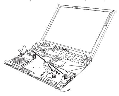
**Note:** For ThinkPad X61 and X61s computers with wireless WAN, re-affix the copper shielding to cover the antenna cables.
