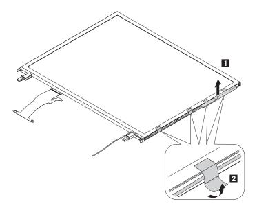
**When installing:** Route the cable properly along the side and into the hinge, and reattach the tape.
