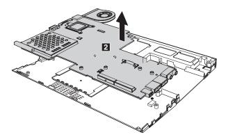
When installing: Do not damage the wireless micro switch 1 on the system board.
