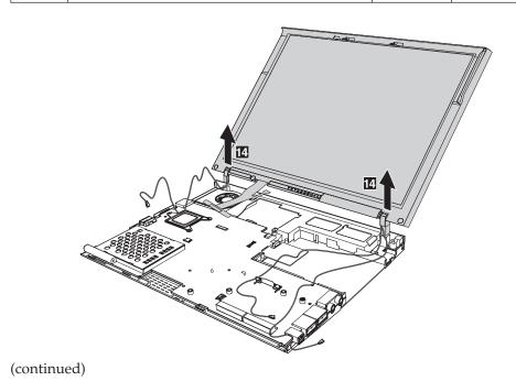
When installing: When fitting the LCD hinge into the system, make sure the wireless antenna cables do not get pinched in by the hinge. Then route the wireless antenna cables as shown below. For wireless WAN: red or black with red tag is main; blue is aux. For wireless LAN: gray is main; black is aux; white is MIMO (for 802.11n models). Remember to reattach the mylar and tapes.
