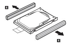
When installing: Make sure that the hard disk is connected firmly.
