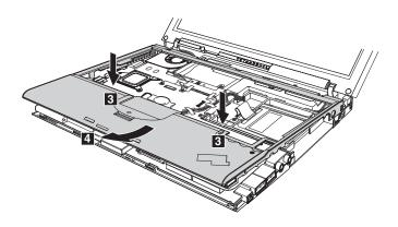
When installing: Follow the steps below to make sure that the upper case is installed firmly.
