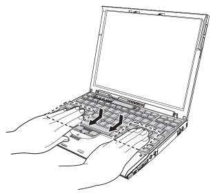
4. Secure the keyboard by tightening the screws from the bottom side of the computer.
