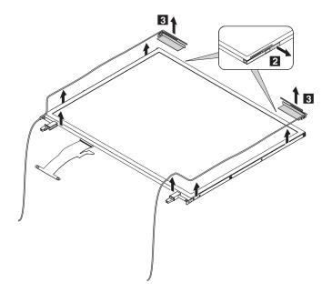
When installing: Route the cable properly along the side and into the hinge.
