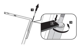
Note: The special tool shown in step 2 for removing the rod antenna is shipped with the rod antenna FRU.
