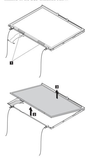
**When installing:** Affix the aluminum shielding for ThinkPad X61 and X61s models with wireless WAN.
