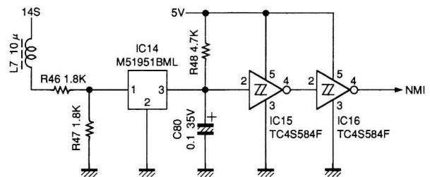
Fig. 4 System backup circuit
