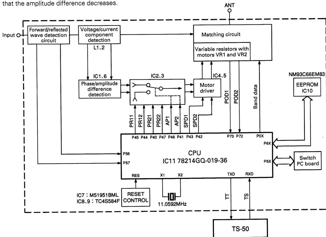
Fig.1 Block diagram
