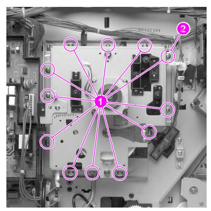
Figure 145. Drum/cartridge drive assembly
