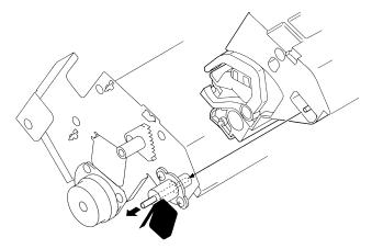
Figure 216. Black toner cartridge detection interlock
