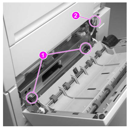
Figure 152. Vertical transfer unit
