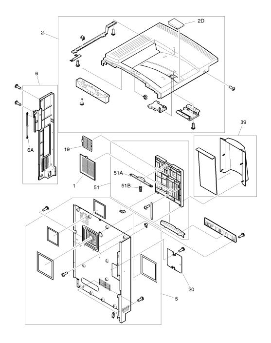
Figure 251. Printer covers and doors (3 of 4)
