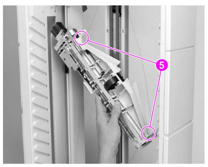
Figure 184. Delivery head assembly (4 of 4)
