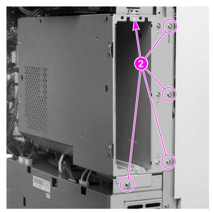
Figure 124. Formatter pan (left side)
