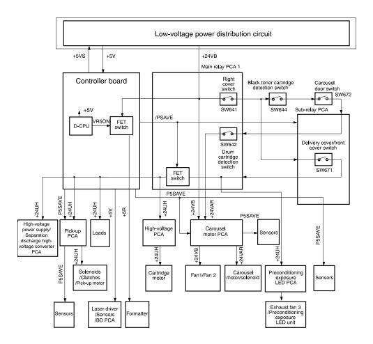
Figure 44. Power distribution circuit diagram
