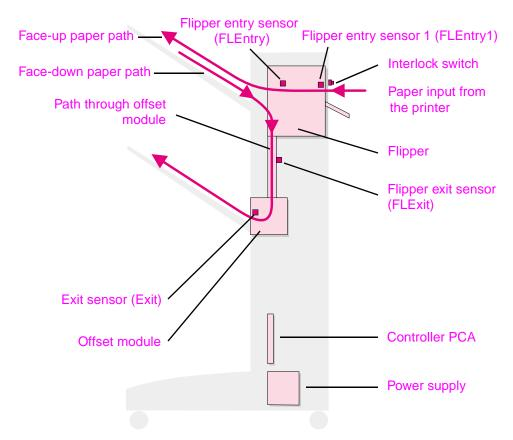
Figure 74. Stacker paper path and sensors
