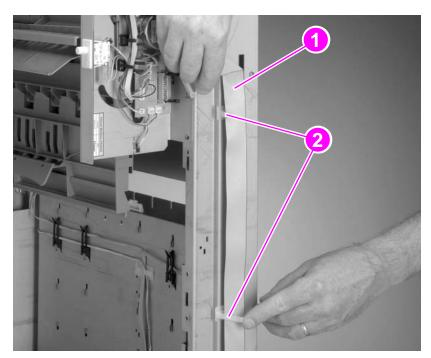
Figure 209. Flipper ribbon cable removal
