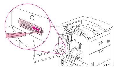
Figure 17. Removing the toner catch tray cover
