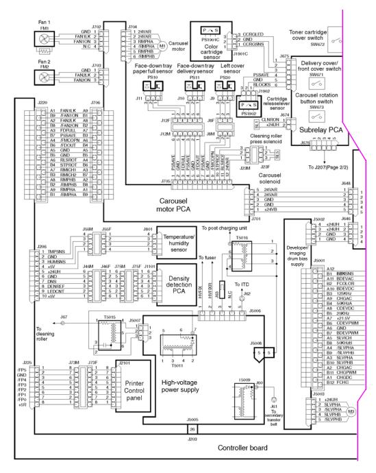
Figure 243. General printer circuit diagram (1 of 4)
