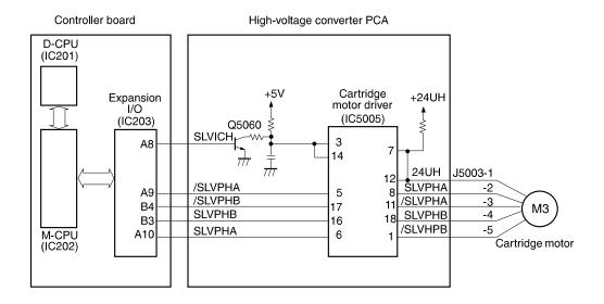
Figure 51. Cartridge motor (M3)
