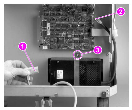
Figure 205. Power supply removal
