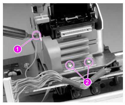
Figure 201. Stapler removal (2 of 3)
