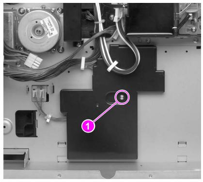
Figure 147. Plate over media size sensing PCAs
