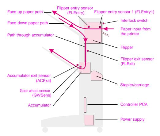
Figure 73. Stapler/stacker paper path and sensors
