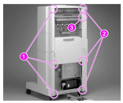
Figure 190. Front and back covers removal
