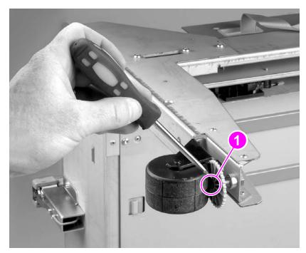
Figure 211. Adjustable caster removal
