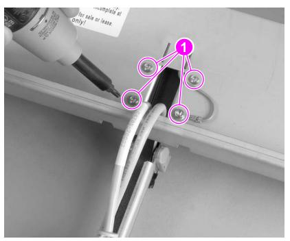
Figure 208. Attachment assembly removal
