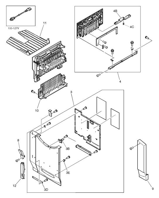
Figure 250. Printer covers and doors (2 of 4)
