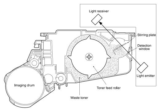
Figure 37. Waste toner level detection
