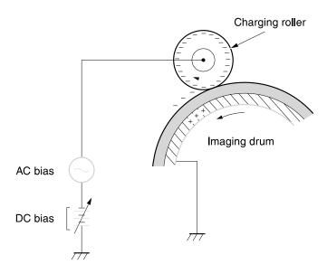
Figure 27. Primary charging of imaging drum
