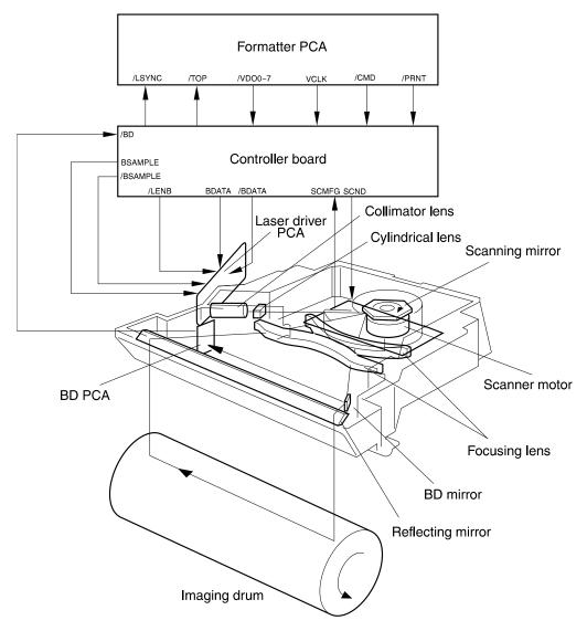
Figure 47. Laser/scanner
