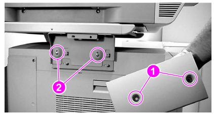
Figure 77. Attachment bracket, HP Color LaserJet 8550 MFP printer
