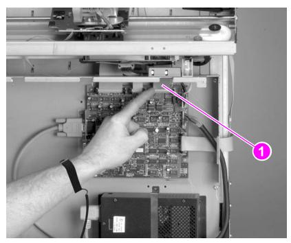
Figure 195. Carriage assembly removal (1 of 2)
