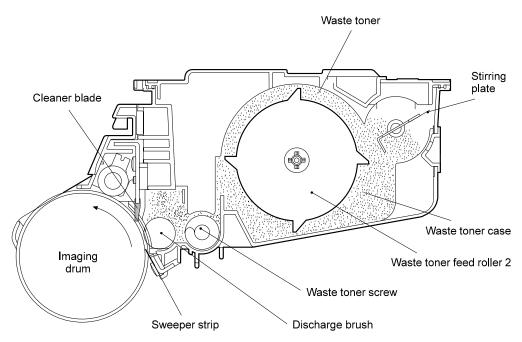
Figure 35. Imaging drum cleaning block
