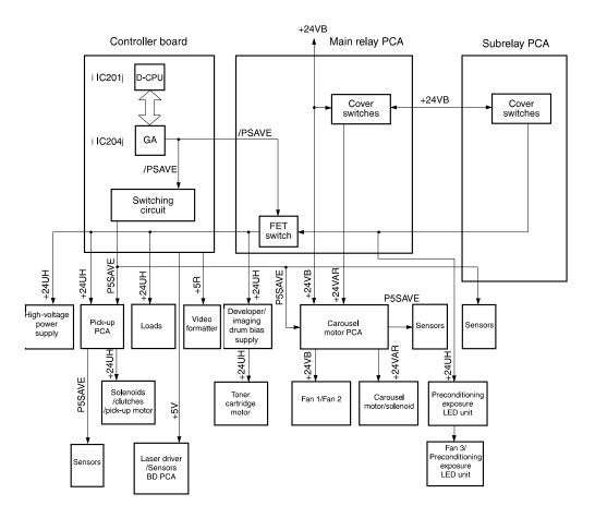
Figure 45. Power Save circuit diagram
