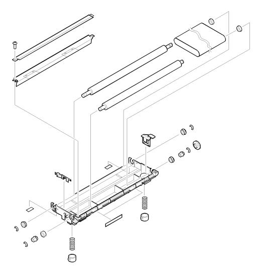
Figure 274. Transfer belt assembly
