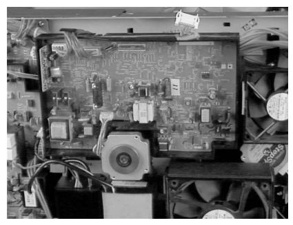
Figure 139. Developer/imaging drum bias supply, HP Color LaserJet 8550 printer
