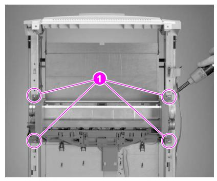
Figure 198. Accumulator assembly removal (2 of 2)
