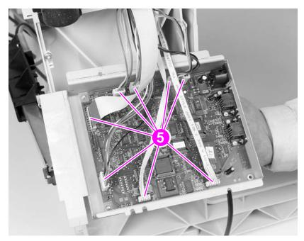
Figure 178. Controller PCA (2 of 2)
