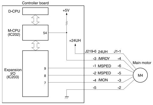
Figure 52. Main motor (M4)
