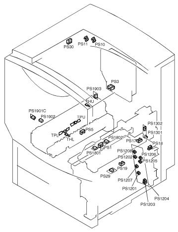
Figure 57. Printer sensors
