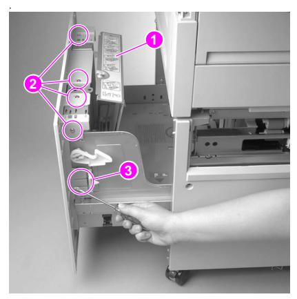
Figure 149. Front cover of the 2,000-sheet input unit
