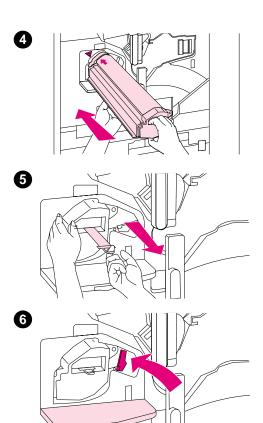
4 Align the arrows on the top of the cartridge and at the top of the slot. Slide the cartridge into the printer.
