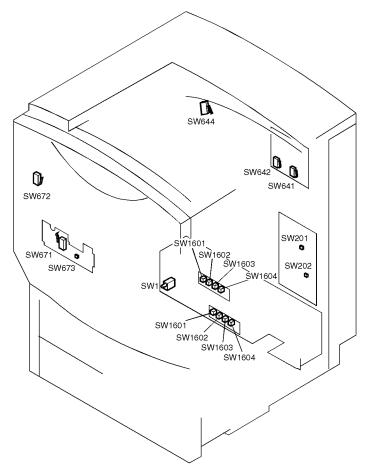
Figure 58. Printer switches
