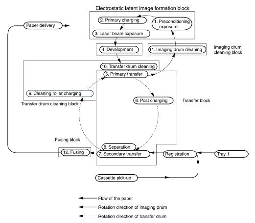
Figure 25. Electrostatic latent image formation block
