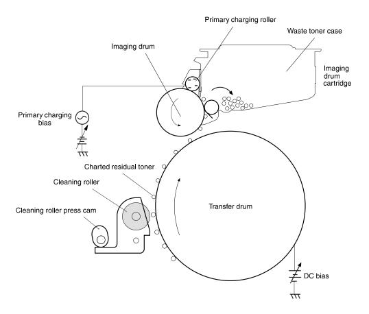
Figure 34. Transfer drum cleaning
