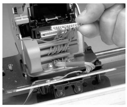
Figure 200. Stapler removal (1 of 3)
