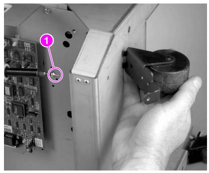
Figure 210. Stationary caster removal
