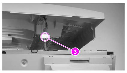
Figure 85. Connector on top cover
