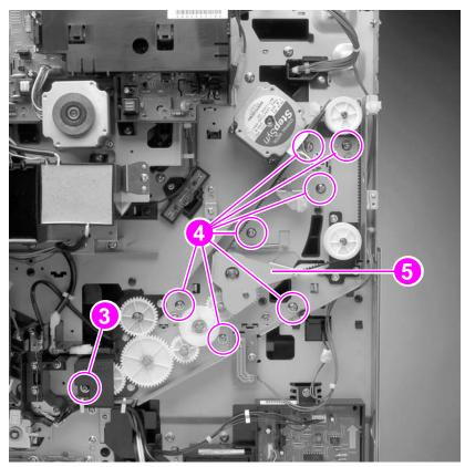
Figure 137. Screws on the delivery drive assembly
