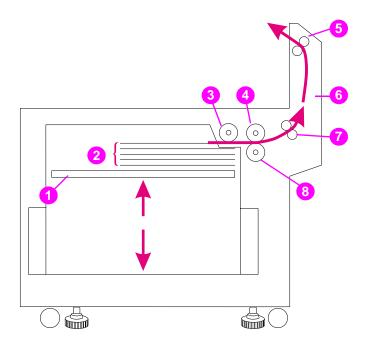
Figure 68. 2,000-sheet input unit paper path
