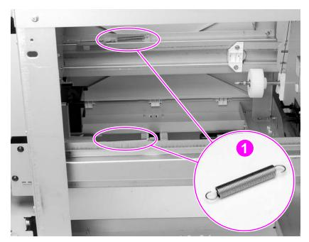
Figure 163. Tension springs
