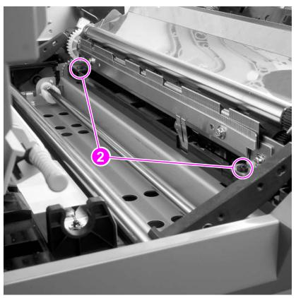
Figure 115. Registration roller assembly (back)
