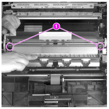
Figure 114. Registration roller assembly (front)
