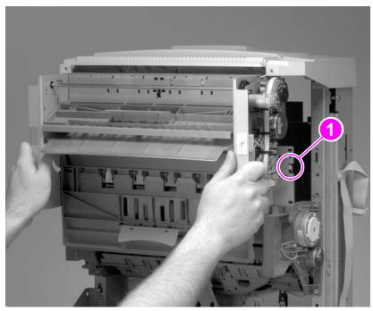
Figure 194. Flipper assembly removal (2 of 2)
