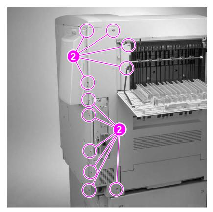
Figure 87. Screws on left rear cover
