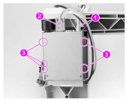
Figure 177. Controller PCA (1 of 2)
