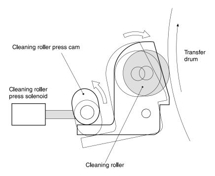
Figure 42. Cleaning roller control
