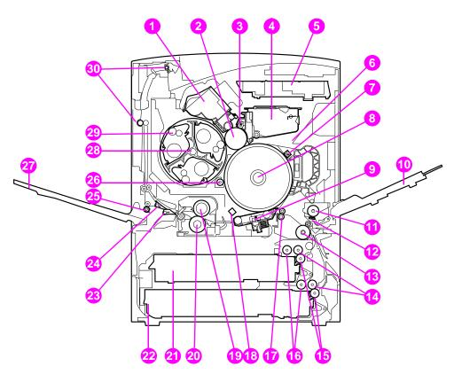
Figure 23. Cross-section view of internal components
