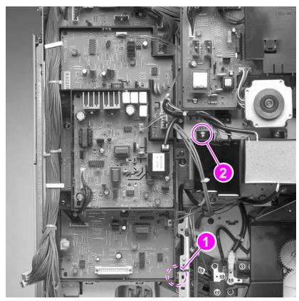
Figure 141. Post charger HV module
