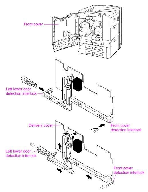
Figure 218. Front cover/delivery cover detection interlocks
