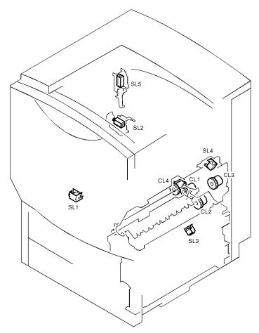
Figure 59. Printer clutches and solenoids
