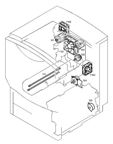
Figure 48. Printer motors and heaters
