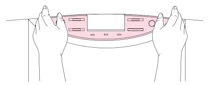
Figure 12. Changing the printer control panel overlay
