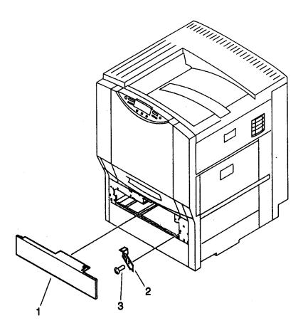
Figure 249. Printer covers and doors (1 of 4)—Filler panel for tray 2 (HP Color LaserJet 8550 base model only)
