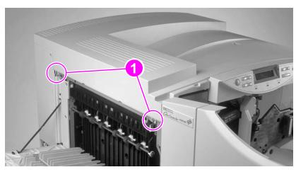
Figure 83. Screws behind left door
