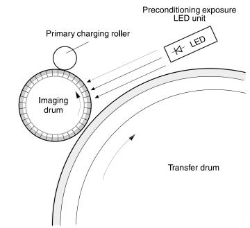
Figure 26. Preconditioning exposure
