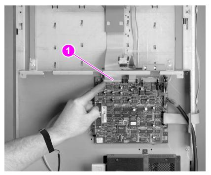
Figure 197. Accumulator assembly removal (1 of 2)
