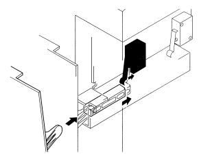
Figure 214. Right upper cover detection interlock
