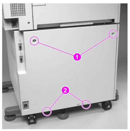
Figure 151. Left cover removal
