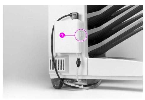
Figure 238. Multi-bin mailbox power supply test mode switch
