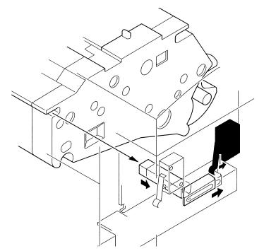
Figure 215. Drum cartridge detection interlock
