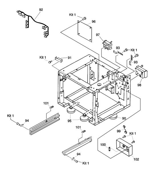
Figure 279. 2,000-sheet input unit internal components
