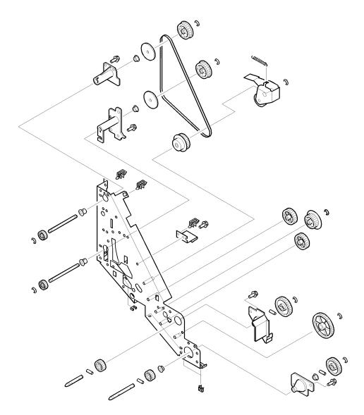
Figure 261. Delivery drive assembly
