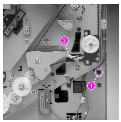
Figure 109. Face-up solenoid (1 of 2)
