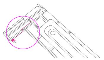
Figure 92. Spring on right cover subassembly
