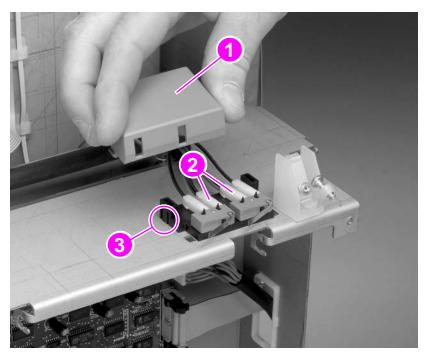
Figure 207. Safety switch assembly removal
