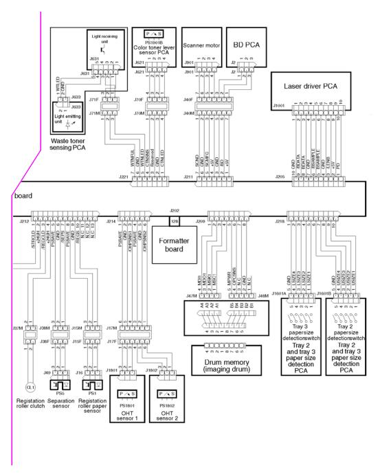
Figure 246. General printer circuit diagram (4 of 4)
