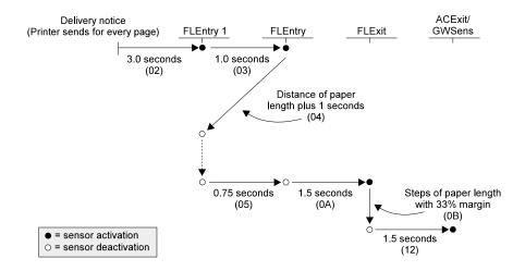
Figure 240. Device timing
