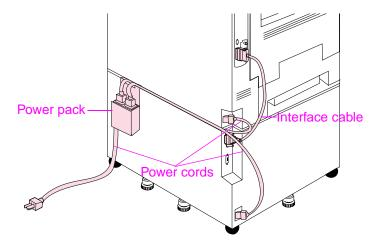
Figure 9. C-link and power cables connections
