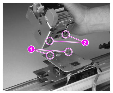
Figure 202. Stapler removal (3 of 3)
