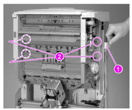
Figure 193. Flipper assembly removal (1 of 2)
