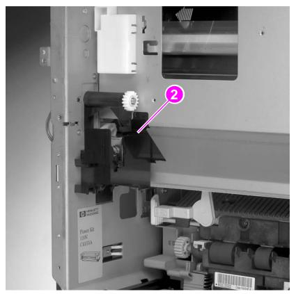
Figure 110. Face-up solenoid (2 of 2)
