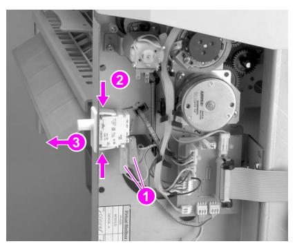
Figure 206. Interlock switch removal
