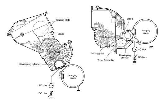
Figure 28. Black toner cartridge (left) and color toner cartridge (right) development
