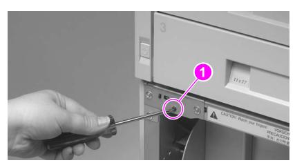
Figure 157. Screw on front LED PCA assembly
