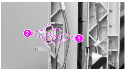
Figure 185. Interlock switch
