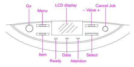
Figure 13. Location of printer control panel features
