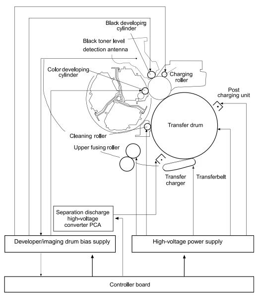
Figure 46. High-voltage power supply circuit
