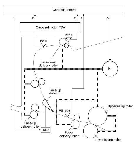
Figure 60. Fusing and delivery unit
