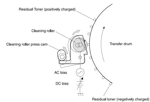
Figure 33. Cleaning roller charging
