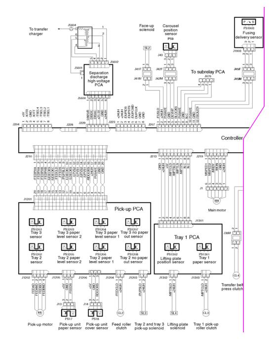
Figure 245. General printer circuit diagram (3 of 4)
