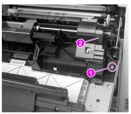
Figure 119. Tray 1 pick-up assembly (1 of 2)
