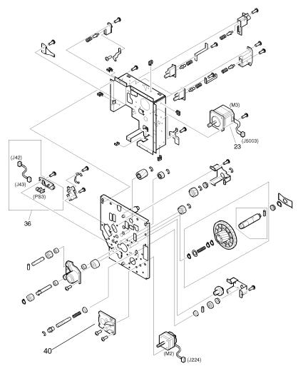
Figure 260. Drum/cartridge drive assembly
