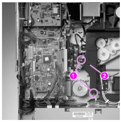
Figure 136. Lower air duct
