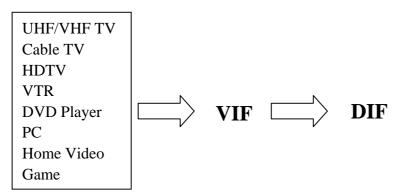
Currently the video signal sources are video cassette recorder, DVD player, CATV, RF tuner, VGA card(PC). In order that all the video signal sources can be displayed on PDP, so we need a interface to transfer these signals to a specified signals for PDP to display, and this is the function of VIF(Video Interface).
