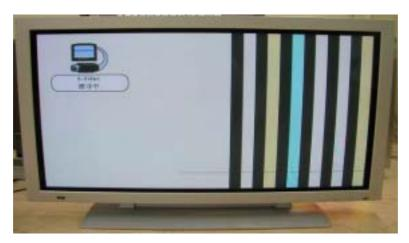
8.11 There are many dark , flicking, bright dot defect or a single or multi pieces of line always appear in the screen, please replace the PDP module.
