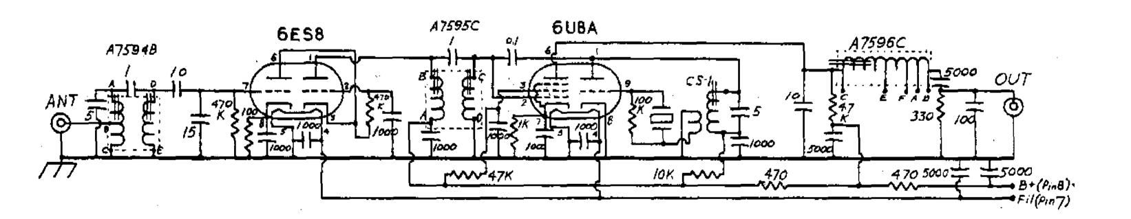
Fig. 2. Wiring schematic of 6 meter Converter, Model CB-6 for 7 to 11 Mc. output. Capacitances are in mmfd. and resistances are in ohms. For other outputs, see changes listed in section on "Selecting the Output IF Frequency".
