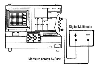
Figure 5-5: Adjusting for Current Amplifier Bias
