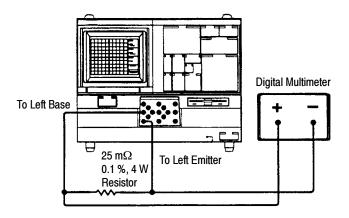
Figure 5-6: Checking for Maximum OFFSET of 200 mA Range
