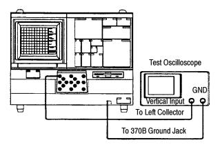
Figure 5-9: Examining for DC and LEAKAGE operation
