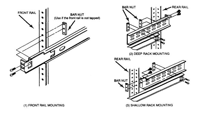
Figure 2-6: Mounting Stationary Rackmount Sections
