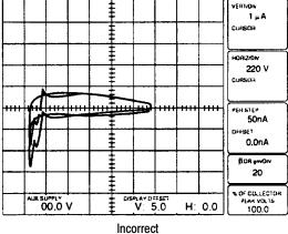
Figure 5-2: Looping compensation display
