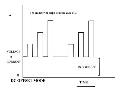
**DC Offset.** Base line offset voltage is always applied to the DUT in spite of Step Generator mode and the Measurement Mode setting.
