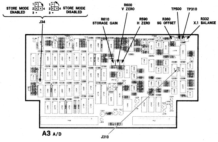
Establishment in shipping is pin 1 and 2 are connected.
