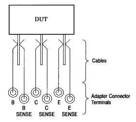
Figure 2-1: Example of Kelvin sense connection
