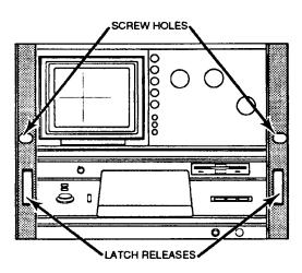
Figure 2-2: Location of the Rackmount Latch Release
