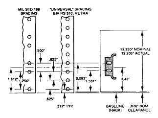
Figure 2-3: Rackmount hole spacing
