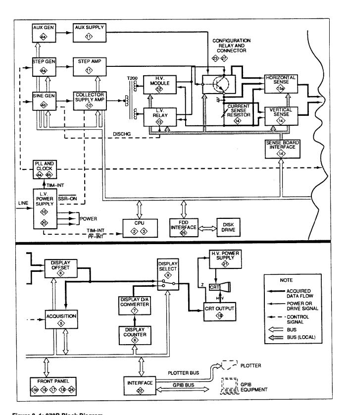
Figure 3-1: 370B Block Diagram
