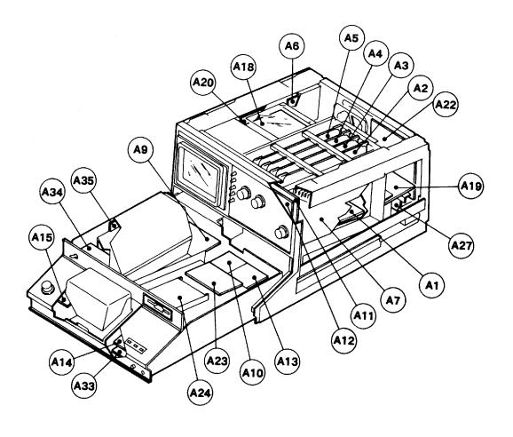
Figure 8-1: 370B circuit board locator
