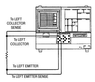
Figure 5-3: Checking Collector high current range
