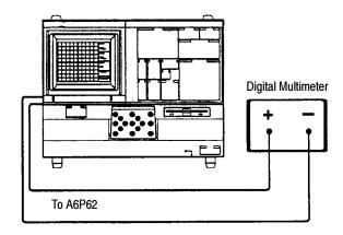
Figure 5-8: Adjusting for Collector Supply Amplifier Offset
