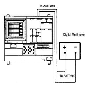
Figure 5-4: Examining and Adjusting for Step Generator Offset
