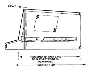
Figure 2-4: Rackmounting Length and Clearance
