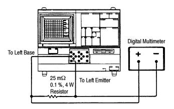
Figure 5-7: Checking for Maximum Current Output of 100 mA and 200 mA range
