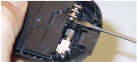
When inserting the battery contacs make sure that you press only on the plastic part.
