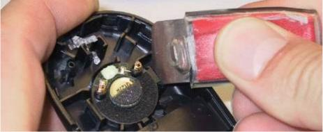
Do not press the contacts when inserting the loudspeaker.
