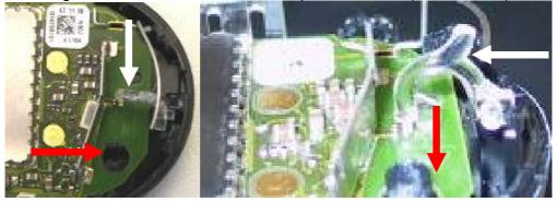
Insert battery connector, vibrator, loudspeaker and close the housing. Pay attention on the light conductor while closing. It must fit exactly in the hole.
