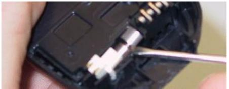
When inserting the vibrator make sure that you press only on the plastic part.
