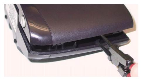
Now the complete side is opened. Open the remaining hooks by spreading the case shells as shown in the next picture.
