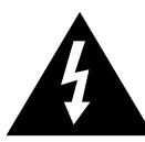
The lightning flash with arrowhead within a triangle is intended to tell the user that parts inside the product are risk of electric shock to persons.
