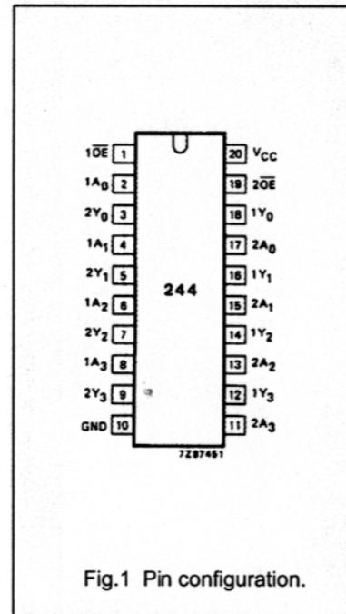
Fig.1 Pin configuration.
