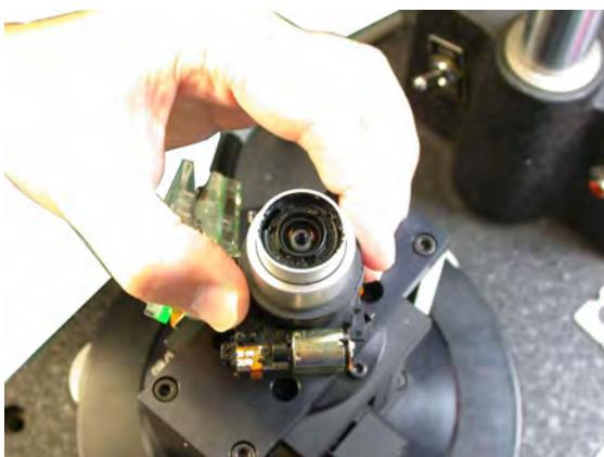
Note: If the lens-barrel unit is held too tightly, the FFD value cannot be measured correctly.
