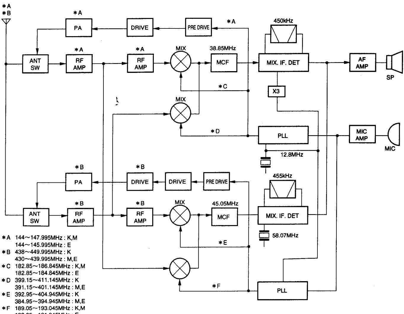
Fig.1 Frequency configuration
