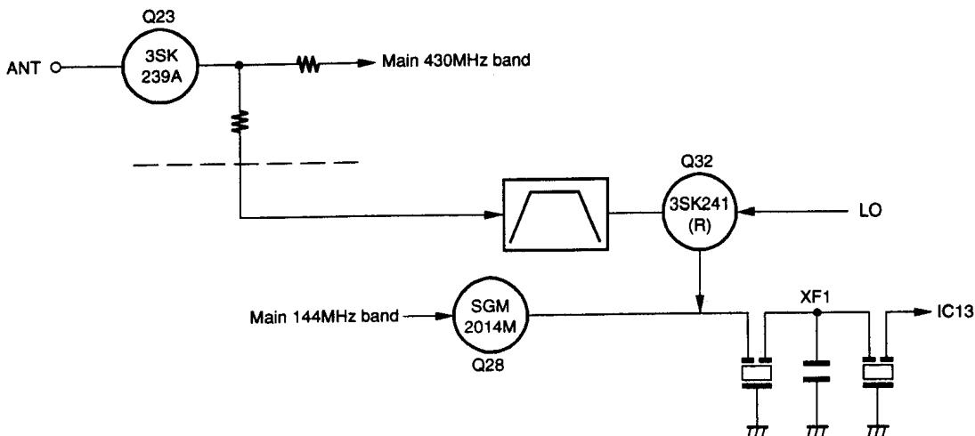
Fig.4 430MHz sub band receive circuit block diagram
