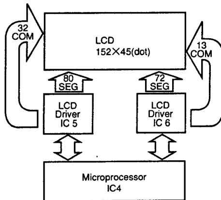
Fig.16 Display circuit
