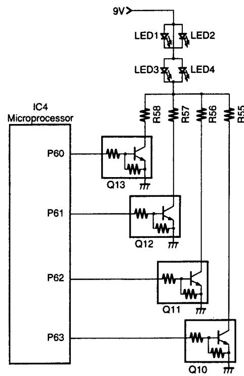
Fig.17 Dimmer circuit
