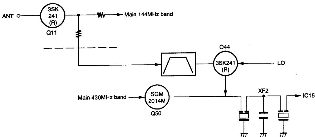
Fig.3 144MHz sub band receive circuit block diagram
