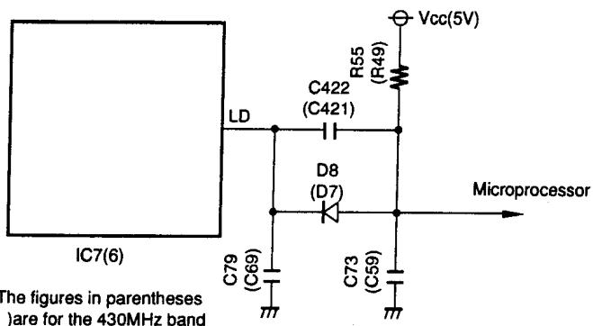
Fig.5 Unlock circuit
