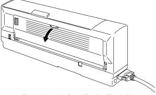
Fig. 2-2 Open the Paper Feeding Slot Guide
