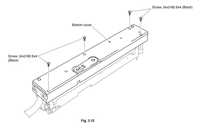
(3) Lift up the Bottom cover. Turn it over, then place it down next to the Paper feed frame ASSY
