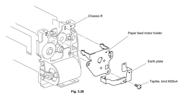
**Note:** The Release plate, Gear 10/30, and Gear 10/20 are assembled on the Paper feed motor holder. Handle the Paper feed motor holder assembly carefully so as not to lose these three parts.
