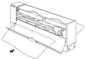
Fig. 5-2 Pulling the Jammed Paper Out
