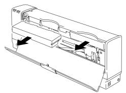
Fig. 4-1 Removing the Cartridge
