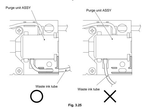
**Important:** Check that the Waste ink tube is fitted correctly into the three guides and two hooks on the Platen cover.
