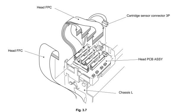
(4) Lifting the outer edge of the PCB, remove the Head PCB ASSY while pulling the hook securing the Head PCB ASSY outwards.
