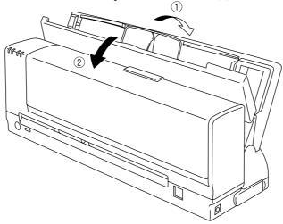
Fig. 2-10 Tilt the Feeder and Open the Cover
