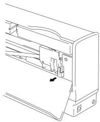
Fig. 5-1 Pulling the Release Lever
