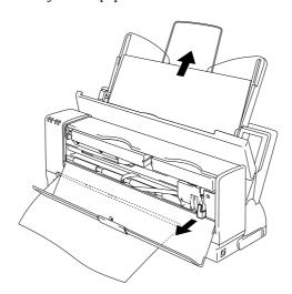
Fig. 5-3 Pulling the Jammed Paper Out
