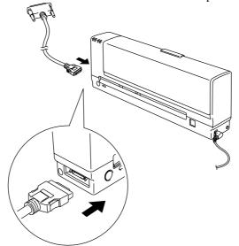
Fig. 9 Connecting the Parallel Interface Cable
