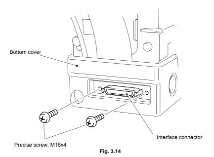
(2) Turn the printer upside down. Remove the four screws.
