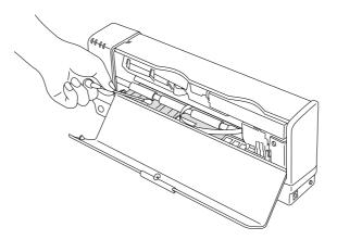
Fig. 4-3 Cleaning the Printer Platen
