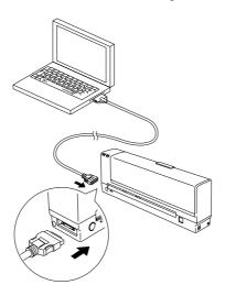
Fig. 7 Connecting the PC Card Cable
