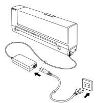
Fig. 8 Connecting the AC Adapter
