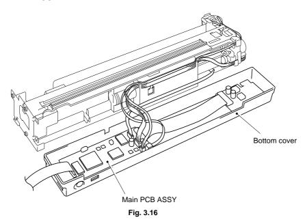
(4) Remove the Carriage motor harness 2P, Paper feed motor harness 4P, Maintenance sensor FFC 3P, and Encoder FFC 5P from the Main PCB ASSY.
