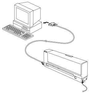
Fig. 10 Connecting the Parallel Interface Cable
