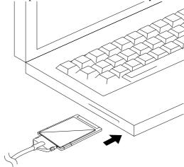
Fig. 6 Inserting the Printer Interface Card
