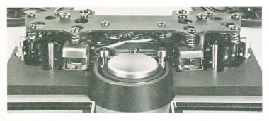
The arrangement of the head block is completely symmetrical in relation to the center capstan. The short and equi-distant tape path within the head block and between heads and reel tables on both sides assure identical performance in both directions. Tension Arms on both the take-up and supply reel sides provide perfect tape tension, also contributing to operating
