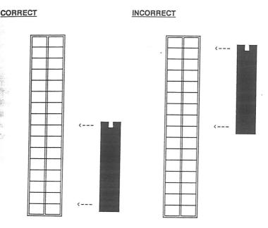
Industry standard 30 pin SIMM modules are inserted into the black 30 pin single in line socket on the unit. Insert the SIMM with the ICs facing to the left. Pin 1 of the SIMM socket is nearest the display. Industry standard 30 pin SIP modules are inserted into the green 30 pin single in line ZIF socket on the unit. Insert the SIP with the ICs facing to the left. Pin 1 of the SIP socket is nearest the display.
