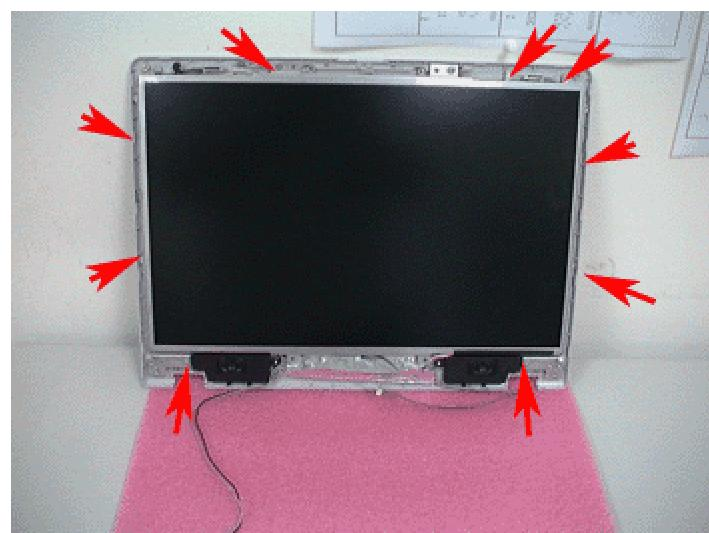
**7. Unfasten 8 screws and remove the lcd panel from the lcd back cabinet.**
