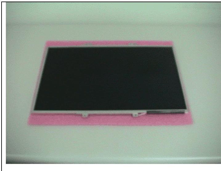
**10. LCD display panel disassembly finished.**
