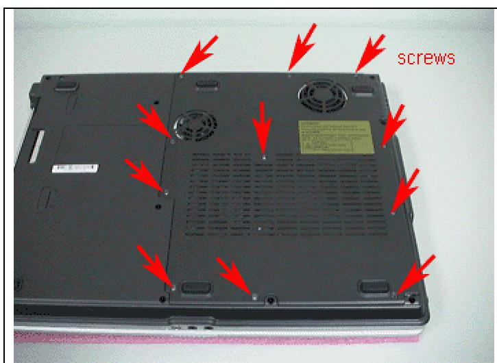
**1. Unfasten 11 screws and remove the CPU cover.**
