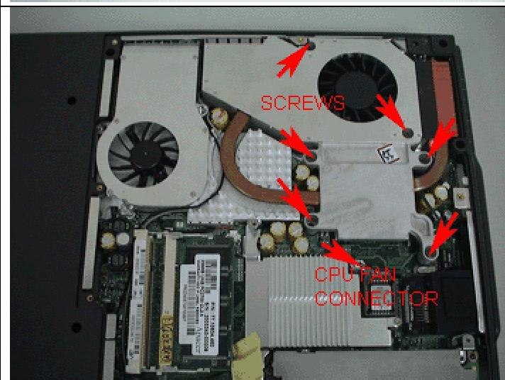
**5. Unfasten 6 screws, disconnect the Cpu fan cable and remove the Cpu fan.**
