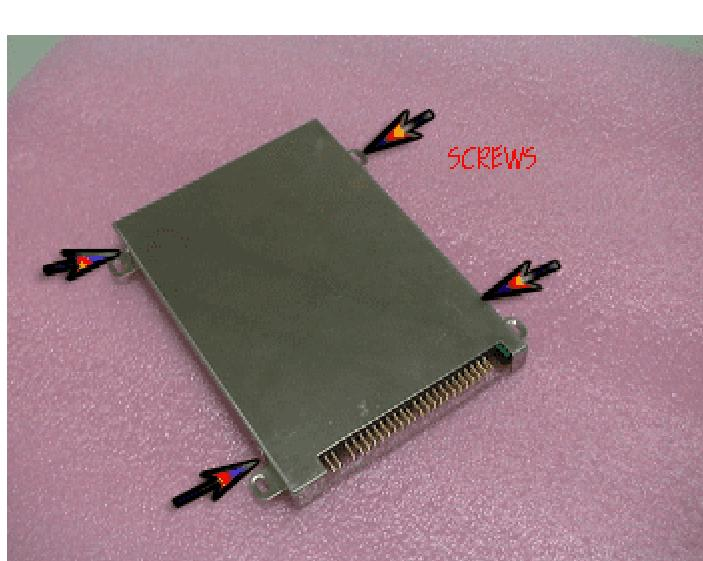
**1. Fasten 4 screws of HDD module.**
