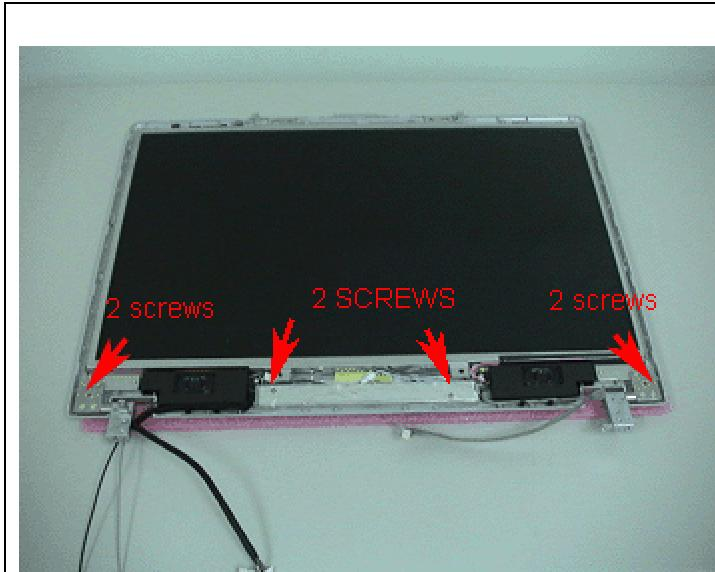
**4. Unfasten the 2 screws in right hinge and 2 screws in left hinge together the the 2 screws in inverter board.**
