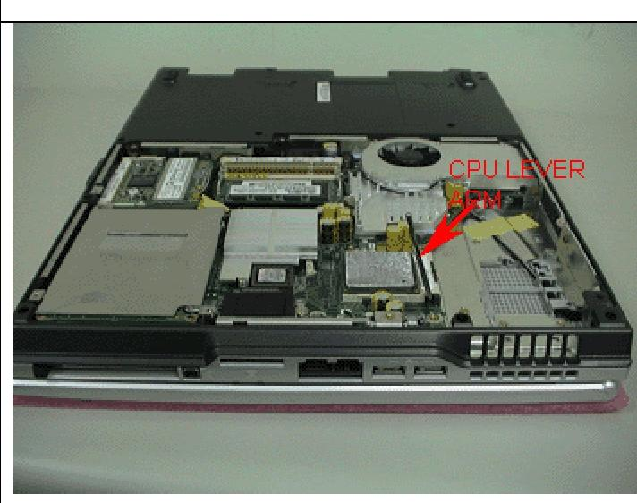
**6. Lift up the CPU lever arm with an angel of 90 degree and remove the CPU.**
