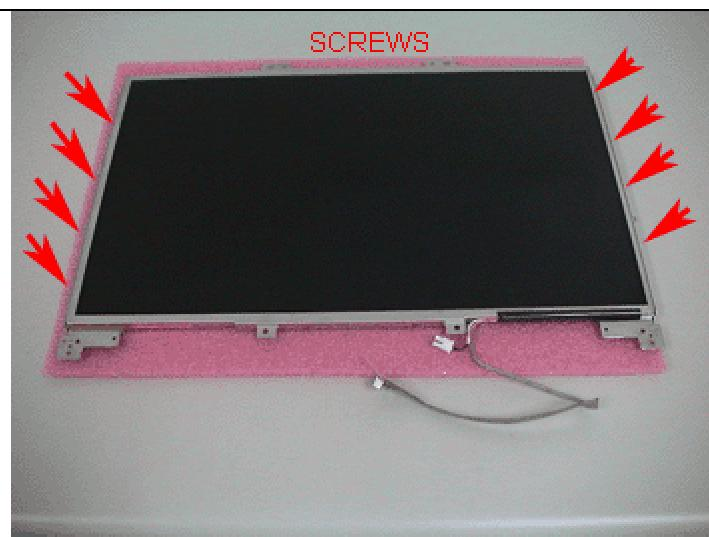
**8. Unfasten 8 screws and remove the right & left lcd bracket.**
