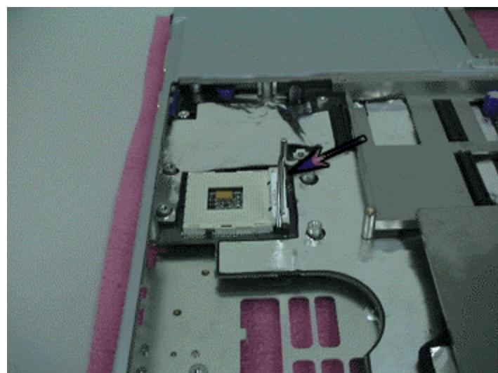
**3. Pull up the lever arm to 90 degree angle sure that the CPU socket is in unlocking position.**
