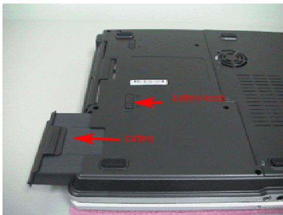
**Unlock the battery knob and pull out the battery pack**
