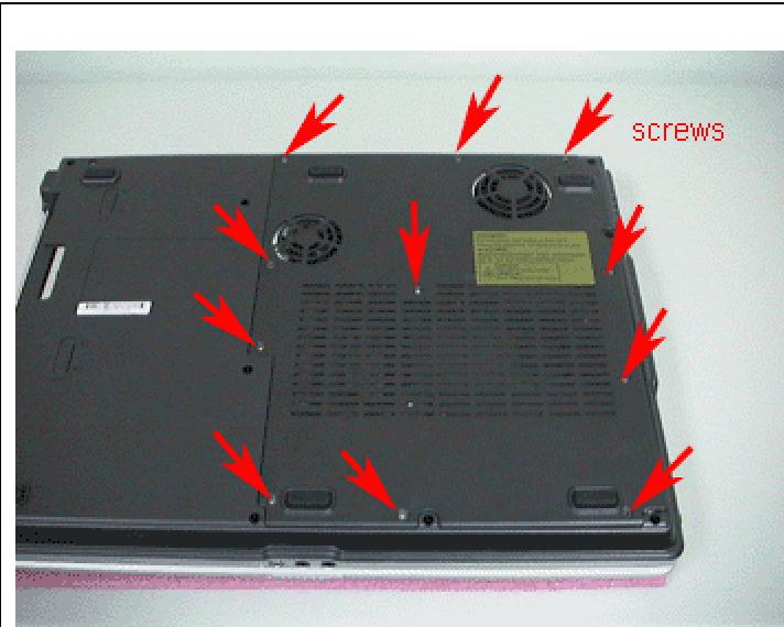
**4. Unfasten 11 screws and remove the CPU and VGA cover.**
