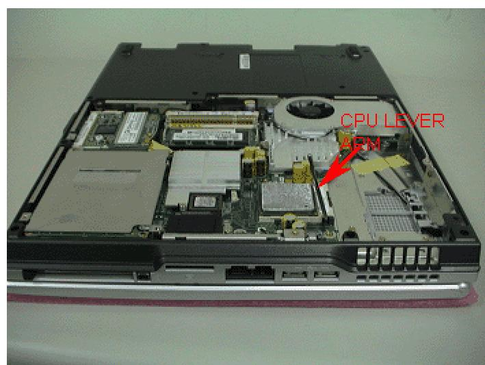
**4. Align the pin 1 of CPU with pin 1 of CPU socket and gently put the CPU into the CPU socket and press down the lever arm.**
