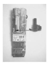
The Vibra Alert unit consisting of the Vibra motor, Capacitor and the flex cable, is attached to the shield case. It is removed by disconnecting from the 9pin connector.
