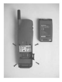
Remove the battery and the 4 screws in the battery compartment. Note that the SIM card is also located in this area
