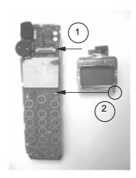
The LCD unit can be lifted out in the way as follows:
