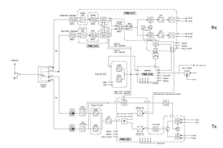
The GMSK modulated 900 MHz / 1800 MHz signal received by the antenna is downconverted into the baseband via an intermediate frequency of 282 MHz. In the transmit direction the digitally GMSK-modulated baseband signal is modulated to the transmit frequency in the 900 MHz / 1800 MHz bands by means of a modulation loop and the dual power VCO.
