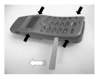
Insert the hook release jig (p/n 3-043-180-01) in the gap between upper and lower case. Then gently slide the jig in the direction of the white arrow. This is to release the claws between the upper and lower case (as indicated by the black arrows).
