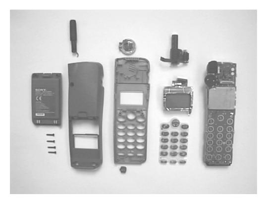
Parts on the main board specified in the parts list can now be reached.
